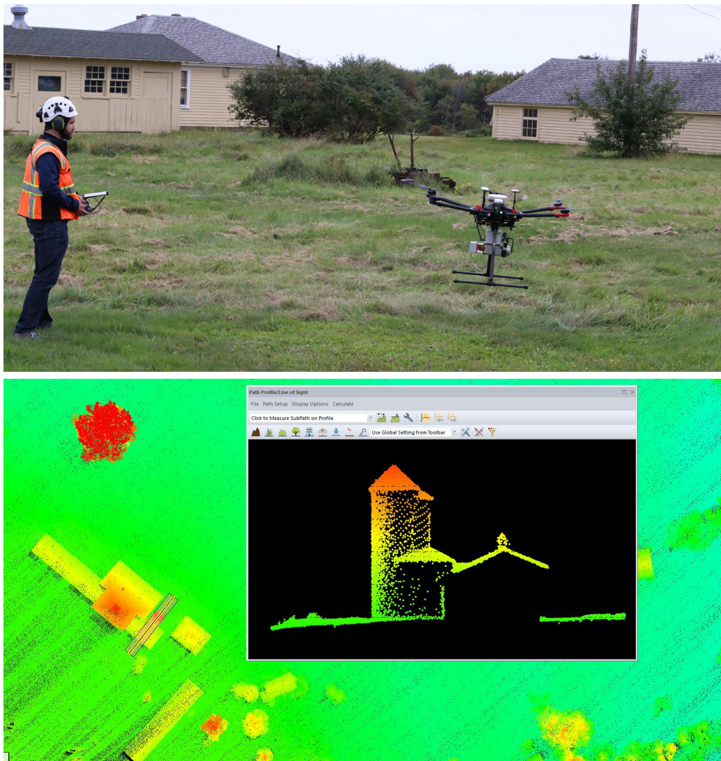
Upper: Landing at end of the AirShark demonstration flight. Lower: LiDAR views from AirShark demonstration flight.
