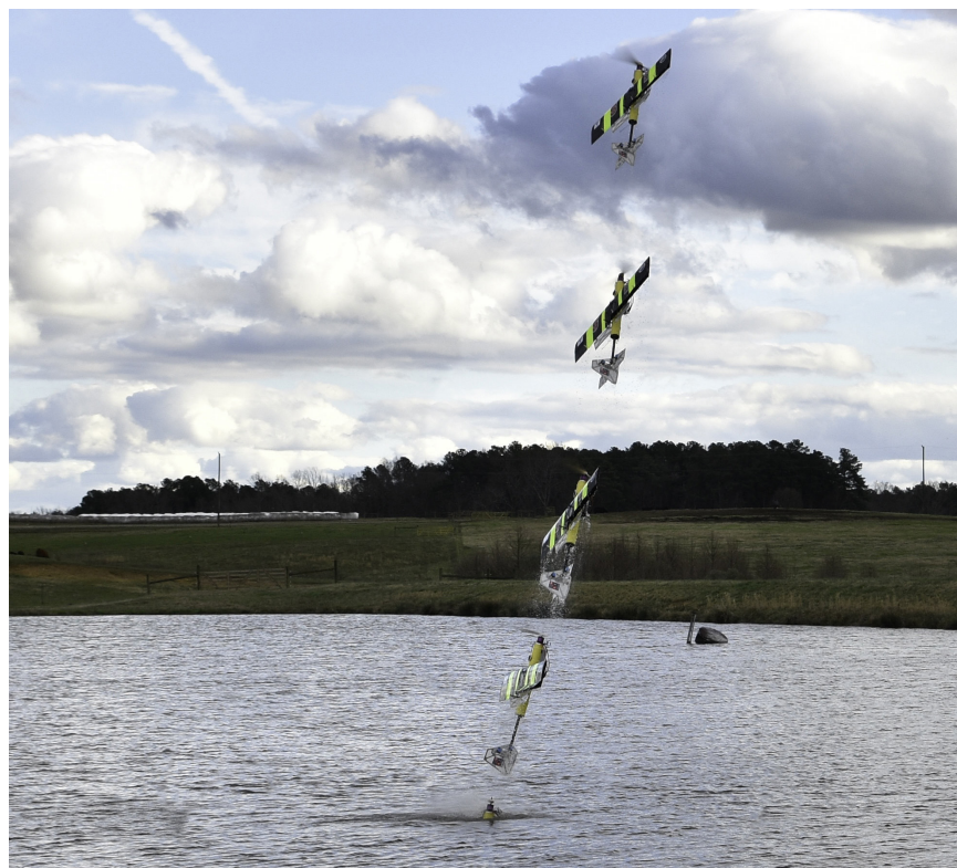
Time lapse photograph of EagleRay XAV leaving the water and entering the air.
