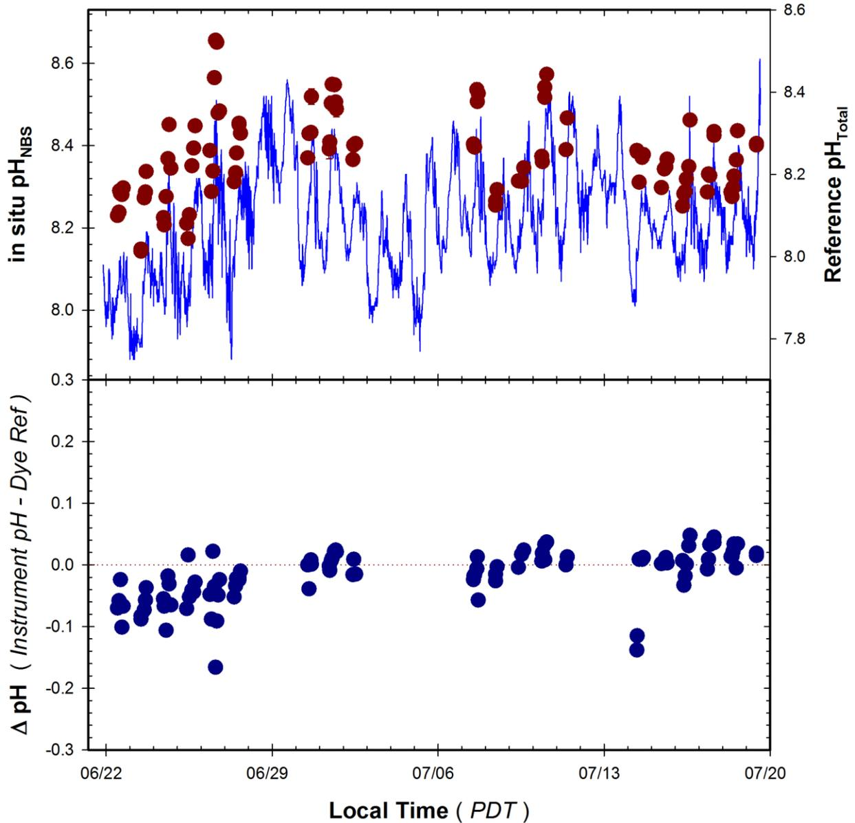
**Figure 29.** Time series of pH measured by the Xylem EXO-pH-2 instrument deployed during the 1 month GLERL field trial. *Top Panel:* Continuous pH<sub>Total</sub> recordings from instrument (blue line) and pH<sub>Total</sub> of adjacent grab samples determined by phenol red dye (red circles). *Bottom Panel:* Difference in measured pH relative to reference samples (Instrument – Dye Ref) observed during deployment.
