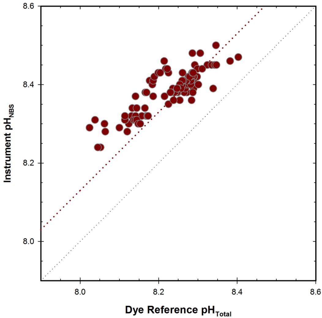
**Figure 25.** CBL field response plot a Xylem EXO pH instrument compared to reference pH<sub>Total</sub> samples. Fine dotted line represents 1:1 correspondence, coarse dotted line represents correspondence predicted based on difference between pH<sub>NBS</sub> and pH<sub>Total</sub> in seawater ( $\text{pH}_{\text{NBS}} = \text{pH}_{\text{Total}} + 0.13$ ).
