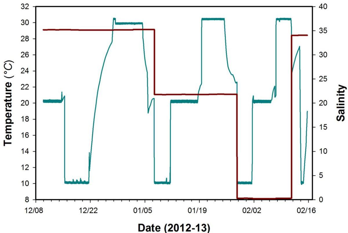
**Figure 1.** Temperature (Teal) and salinity (Red) conditions maintained throughout the ten week long laboratory test. Sensors were tested at three temperatures (10, 20, 30 °C) at each of three salinities (0.3, 22, 35). Full seawater salinity conditions were briefly re-established at the end of the test and cycled through the same temperature range to fill in missing instrument coverage.
