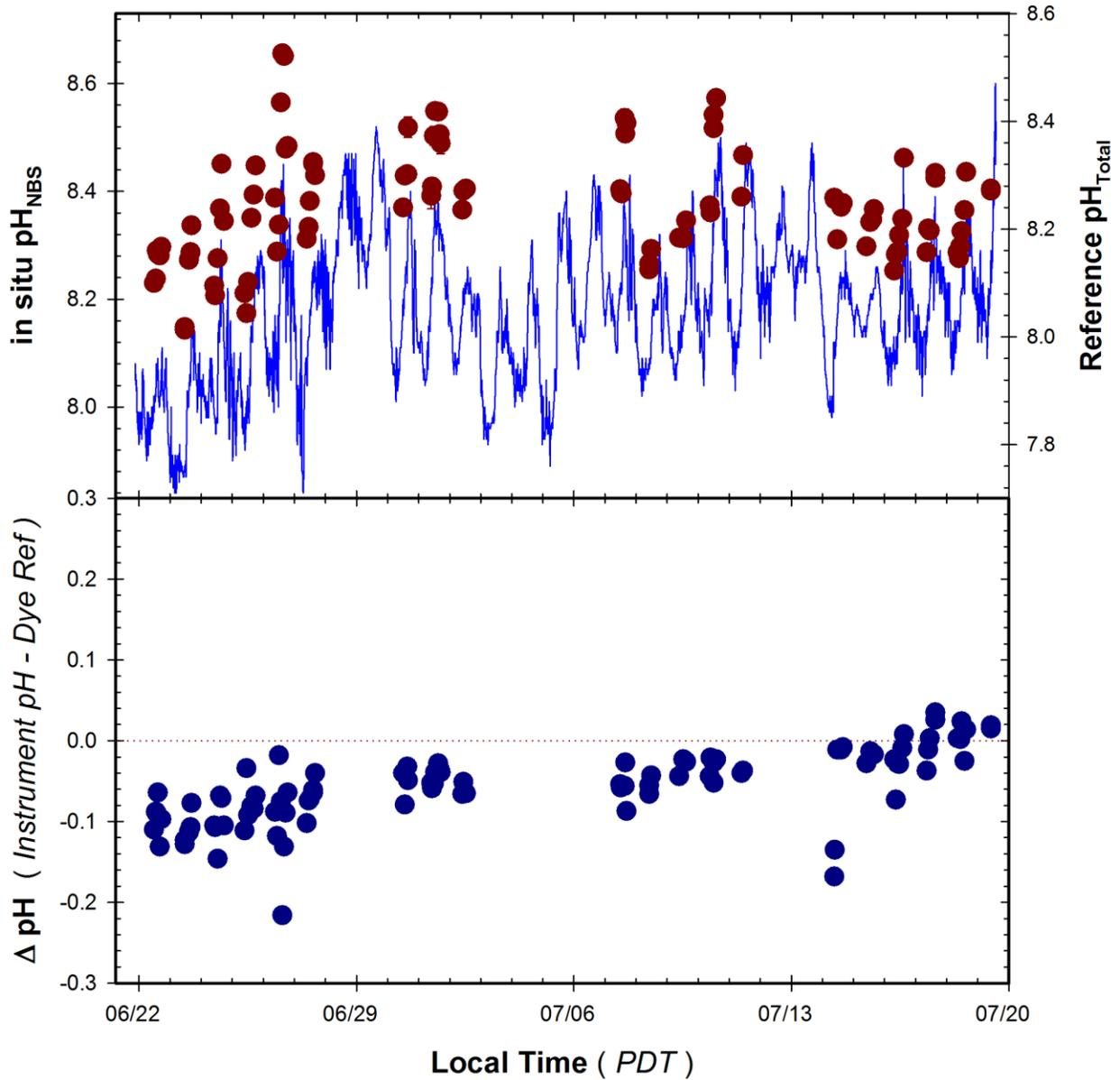
**Figure 27.** Time series of pH measured by the Xylem EXO-pH1 instrument deployed during the 1 month GLERL field trial. *Top Panel:* Continuous pH<sub>Total</sub> recordings from instrument (blue line) and pH<sub>Total</sub> of adjacent grab samples determined by phenol red dye (red circles). *Bottom Panel:* Difference in measured pH relative to reference samples (Instrument – Dye Ref) observed during deployment.
