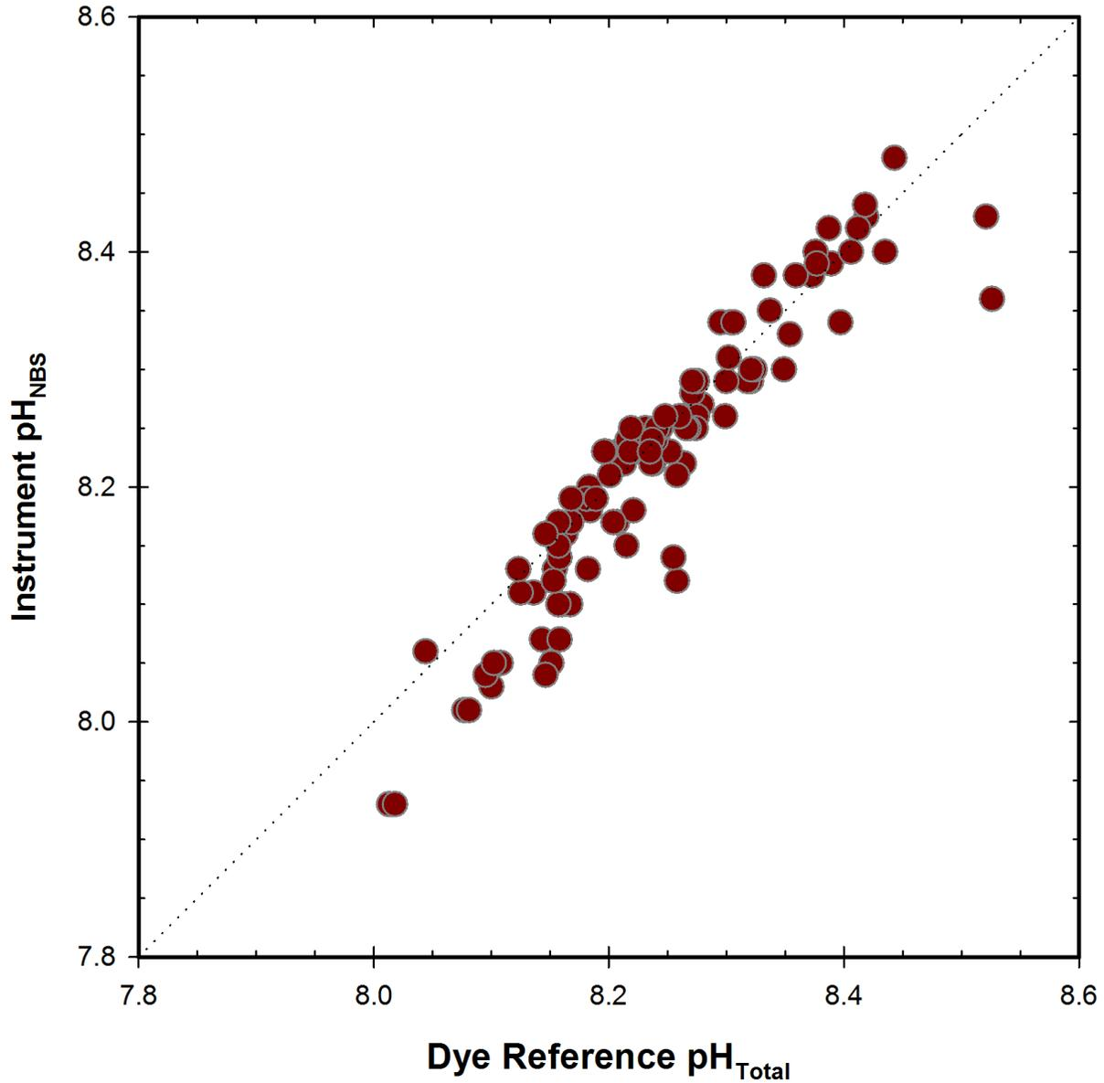
**Figure 30.** GLERL field response plot for the Xylem EXO-pH2 instrument compared to reference pH<sub>Total</sub> samples. Fine dotted line represents 1:1 correspondence.
