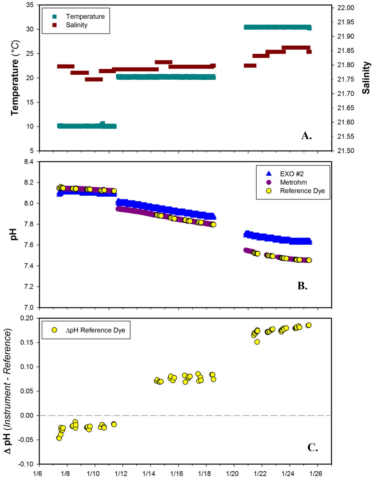
**Figure 8.** Time series results of the Xylem EXO-pH2 sensor for the stable portion of the brackish water trials. Measurements taken during temperature and pH shifts have been removed. Panel (a) temperature and salinity conditions during the brackish water trials; panel (b) measured pH from the EXO-pH2 plotted against both Metrohm and Dye reference pH measurements; and, panel (c) the difference between EXO and reference pH values.
