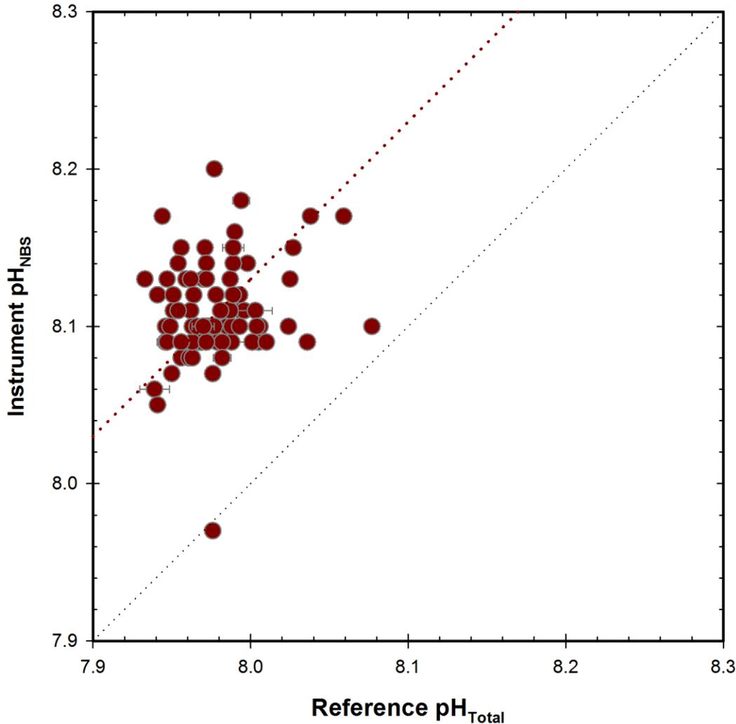
**Figure 15.** MLML field response plot of the Xylem EXO-pH1 instrument compared to reference pH<sub>Total</sub> samples. Fine dotted line represents 1:1 correspondence, coarse dotted line represents correspondence predicted based on difference between pH<sub>NBS</sub> and pH<sub>Total</sub> in seawater ( $pH_{NBS} = pH_{Total} + 0.13$ ).
