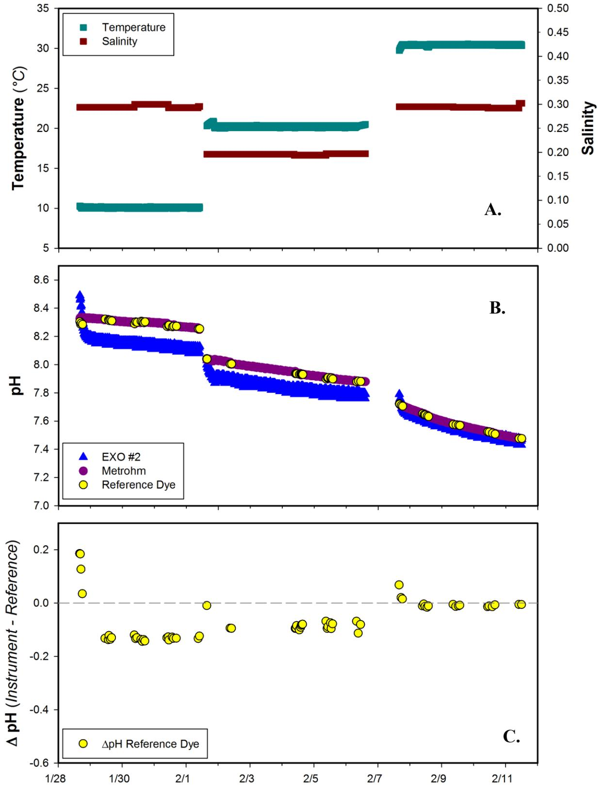
**Figure 10.** Time series results of the Xylem EXO-pH2 sensor for the stable portion of the freshwater trials. Measurements taken during temperature and pH shifts have been removed. Panel (a) temperature and salinity conditions during the freshwater trials; panel (b) measured pH from the EXO-pH2 plotted against both Metrohm and Dye reference pH measurements; and, panel (c) the difference between EXO and reference pH values.
