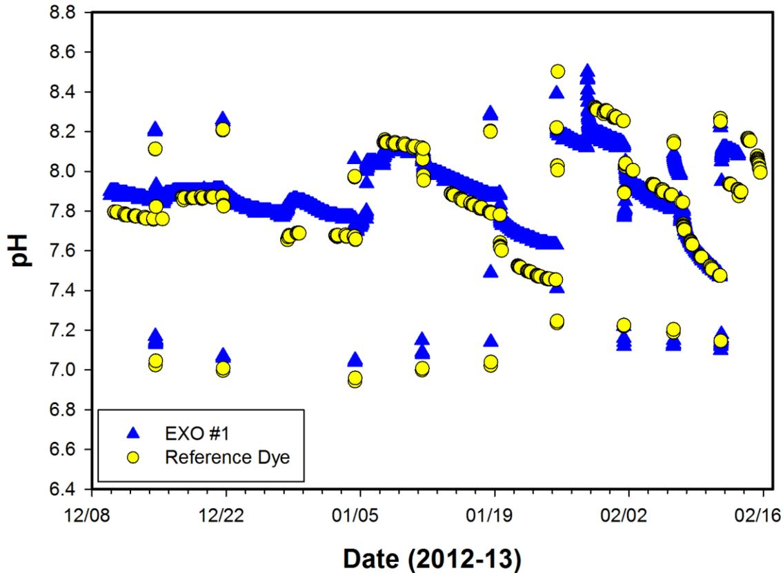
**Figure 3.** Time series of the Xylem EXO-pH1 test instrument pH results along with the dye reference pH results for the complete ten week lab test. Results include nine rapid pH transition tests conducted at each temperature and salinity condition. Detailed plots of each transition test are provided in Appendix I.
