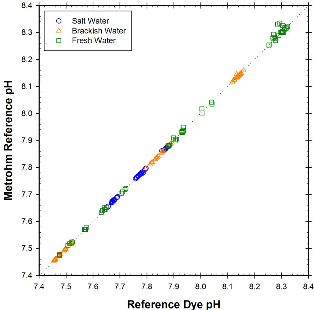
**Figure 2.** Cross plot of matched Metrohm pH results that measured continuously within the test tank at 15 minute intervals versus dye measured reference pH results. Three-hundred, fifty-one dye based pH measurements were made over the ten week test.
