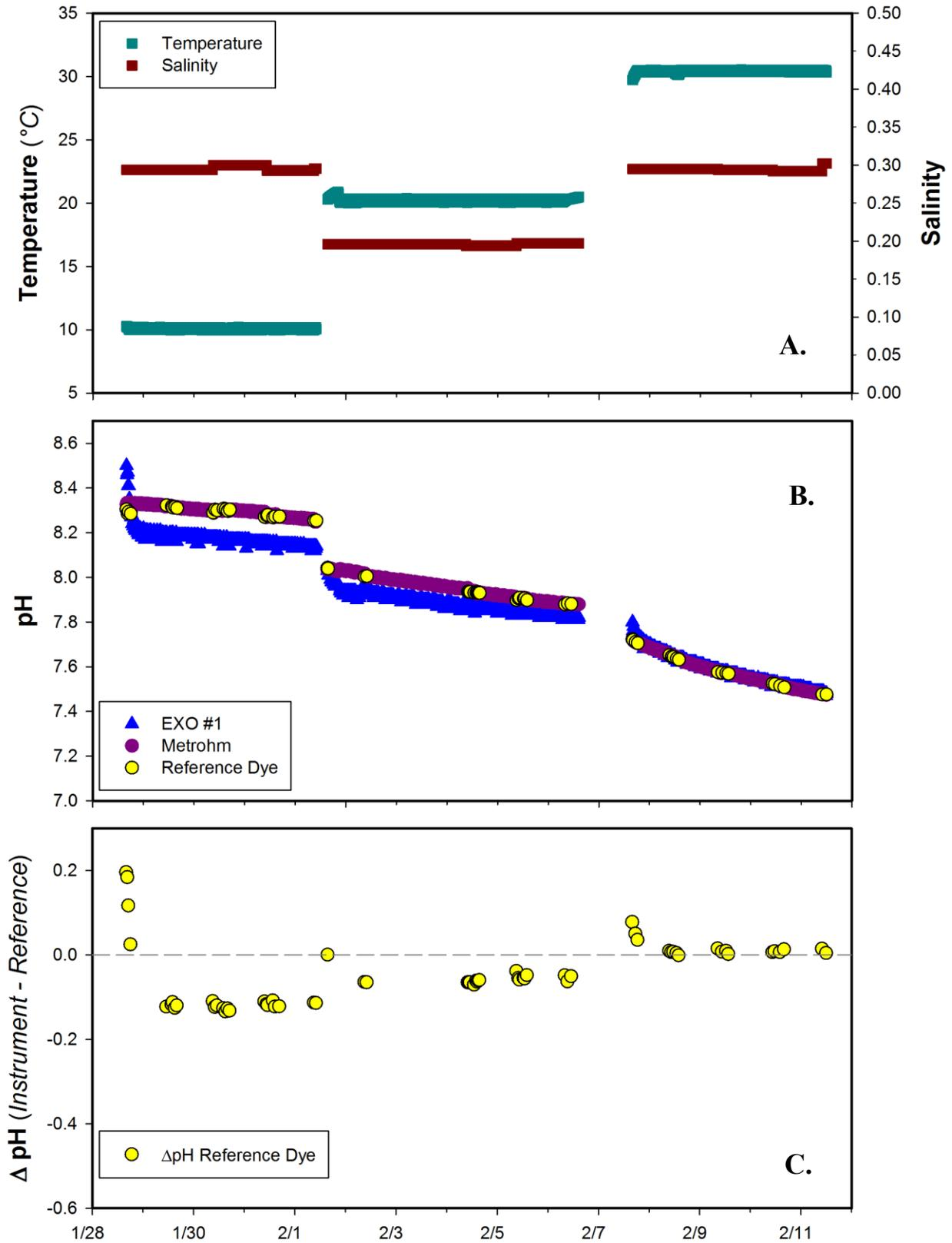
**Figure 9.** Time series results of the Xylem EXO-pH1 sensor for the stable portion of the freshwater trials. Measurements taken during temperature and pH shifts have been removed. Panel (a) temperature and salinity conditions during the freshwater trials; panel (b) measured pH from the EXO-pH1 plotted against both Metrohm and Dye reference pH measurements; and, panel (c) the difference between EXO and reference pH values.
