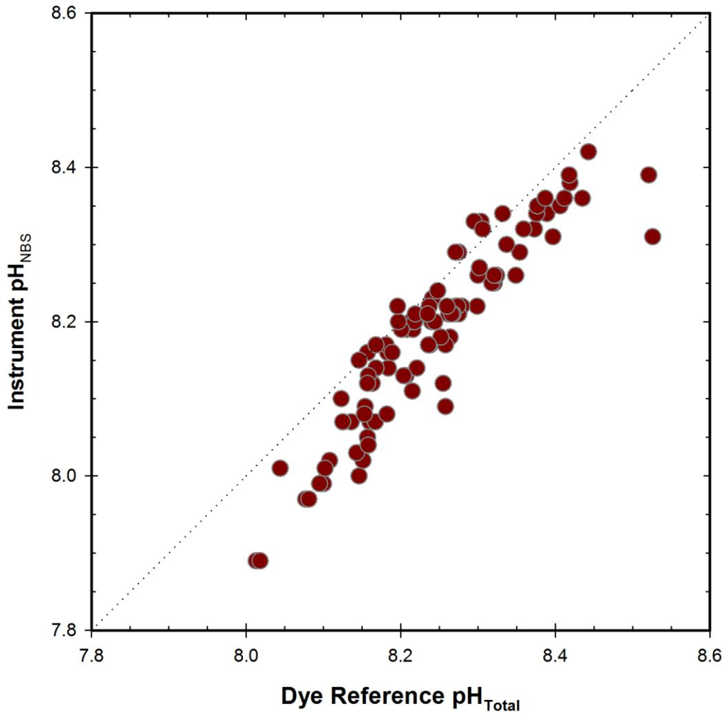
**Figure 28.** GLERL field response plot for the Xylem EXO pH 1 instrument compared to reference pH<sub>Total</sub> samples. Fine dotted line represents 1:1 correspondence.
