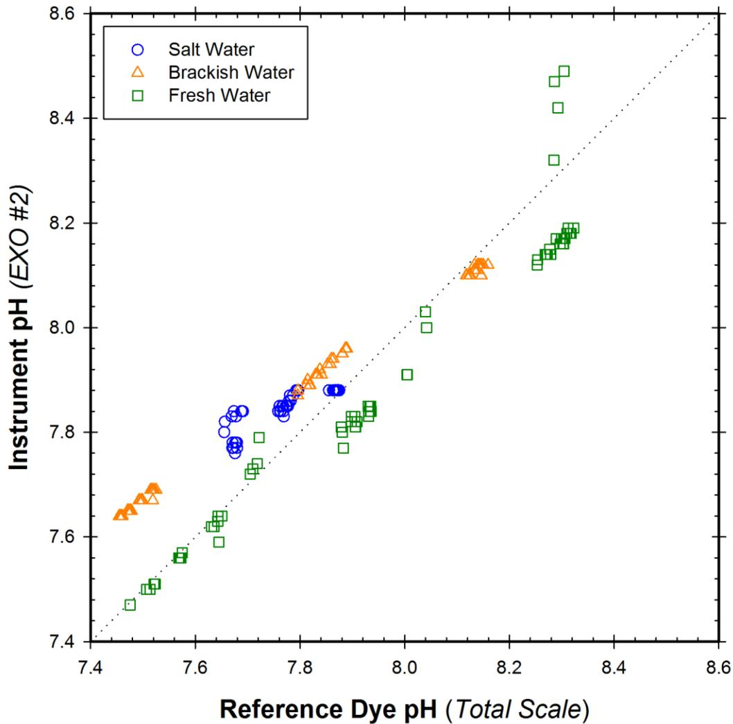
**Figure 12.** Cross plot of Xylem EXO-pH2 measurements against the dye reference pH measurements for 201 matched observations during the stable Temperature and Salinity portions of the entire lab test.
