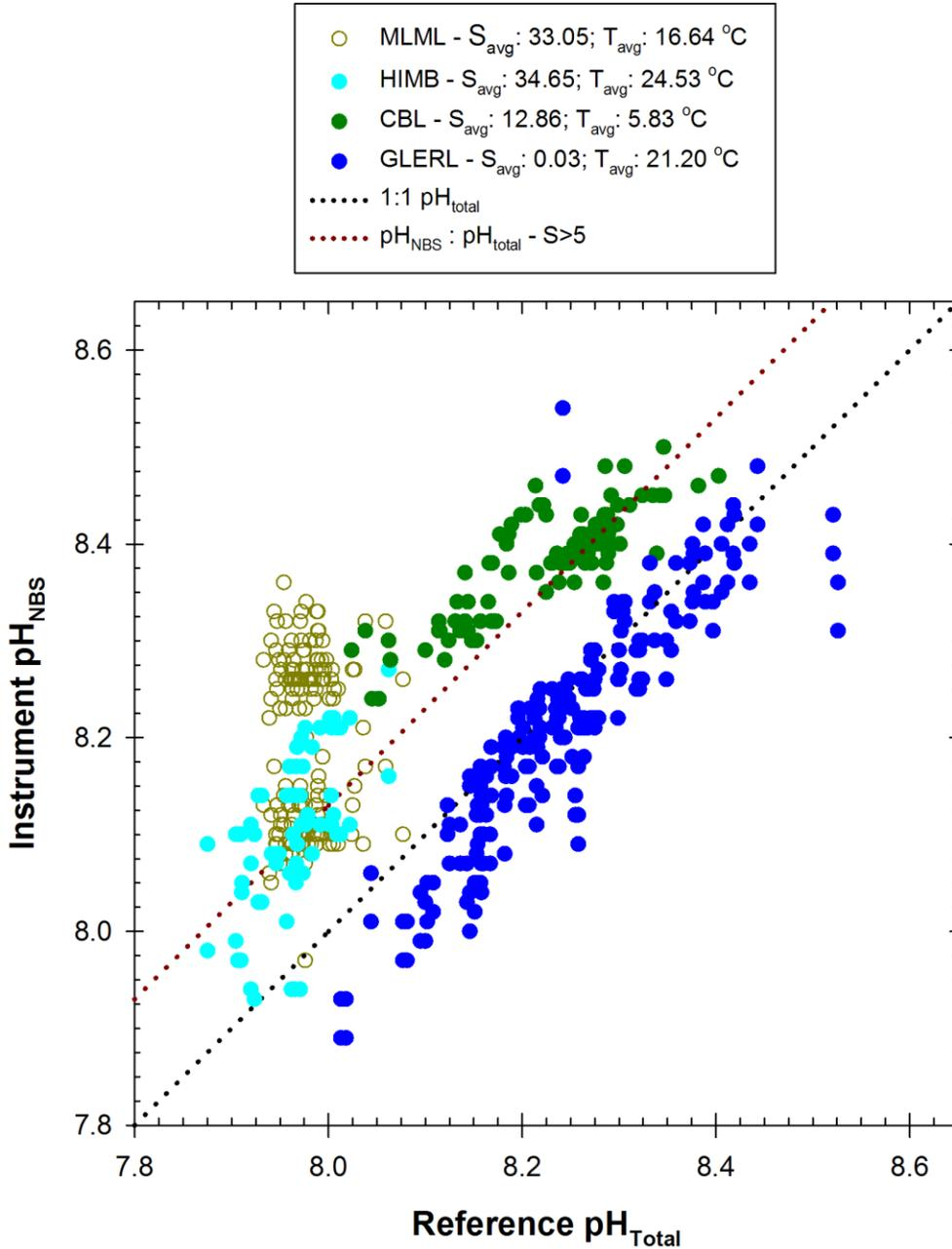
**Figure 31.** Global response plot for all of the Xylem EXO pH sensors deployed during ACT field trials. Black dotted line represents 1:1 equivalence of scales expected in freshwater, dark red dotted line represents correspondence predicted based on difference between  $pH_{NBS}$  and  $pH_{Total}$  in seawater ( $pH_{NBS} = pH_{Total} + 0.13$ ).
