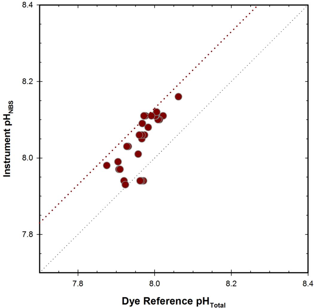
**Figure 22.** HIMB field response plot of EXO-pH2 compared to reference pH<sub>Total</sub> samples. Fine dotted line represents 1:1 correspondence, coarse dotted line represents correspondence predicted based on difference between pH<sub>NBS</sub> and pH<sub>Total</sub> in seawater ( $\text{pH}_{\text{NBS}} = \text{pH}_{\text{Total}} + 0.13$ ).
