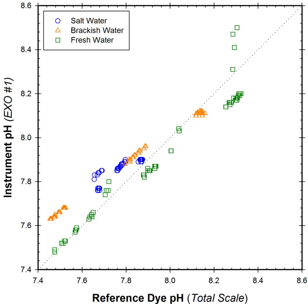
**Figure 11.** Cross plot of Xylem EXO-pH1 measurements against the dye reference pH measurements for 201 matched observations during the stable Temperature and Salinity portions of the entire lab test.
