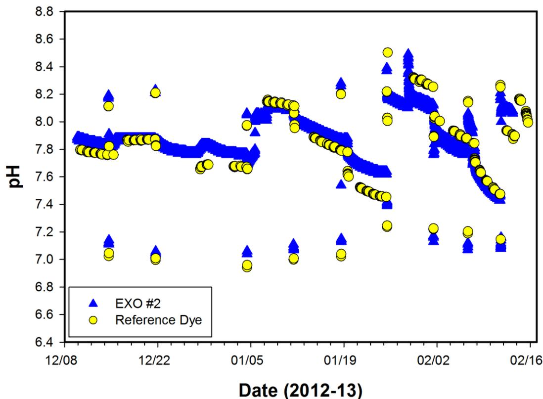
**Figure 4.** Time series of the Xylem EXO-pH2 test instrument pH results along with the dye reference pH results for the complete ten week lab test. Results include nine rapid pH transition tests conducted at each temperature and salinity condition. Detailed plots of each transition test are provided in Appendix I.
