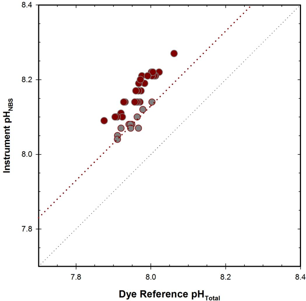
**Figure 20.** HIMB field response plot of EXO-pH1 (dark red circles) and the second deployed EXO sonde pH (grey circles) compared to reference  $pH_{Total}$  samples. Fine dotted line represents 1:1 correspondence, coarse dotted line represents correspondence predicted based on difference between  $pH_{NBS}$  and  $pH_{Total}$  in seawater ( $pH_{NBS} = pH_{Total} + 0.13$ ).
