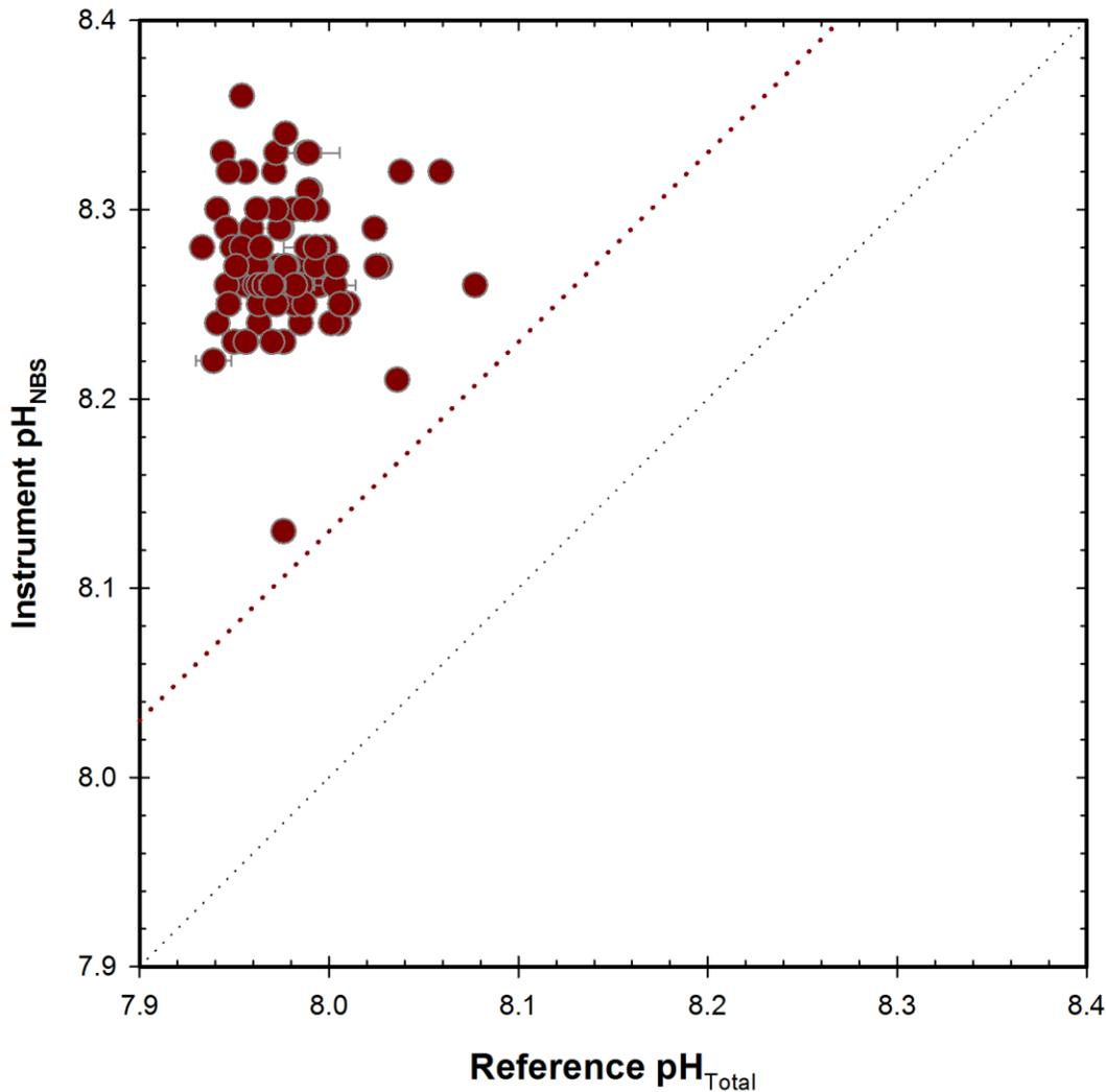
**Figure 17.** MLML field response plot of the Xylem EXO-pH2 instrument compared to reference pH<sub>Total</sub> samples. Fine dotted line represents 1:1 correspondence, coarse dotted line represents the correspondence predicted based on difference between pH<sub>NBS</sub> and pH<sub>Total</sub> in seawater ( $\text{pH}_{\text{NBS}} = \text{pH}_{\text{Total}} + 0.13$ ).
