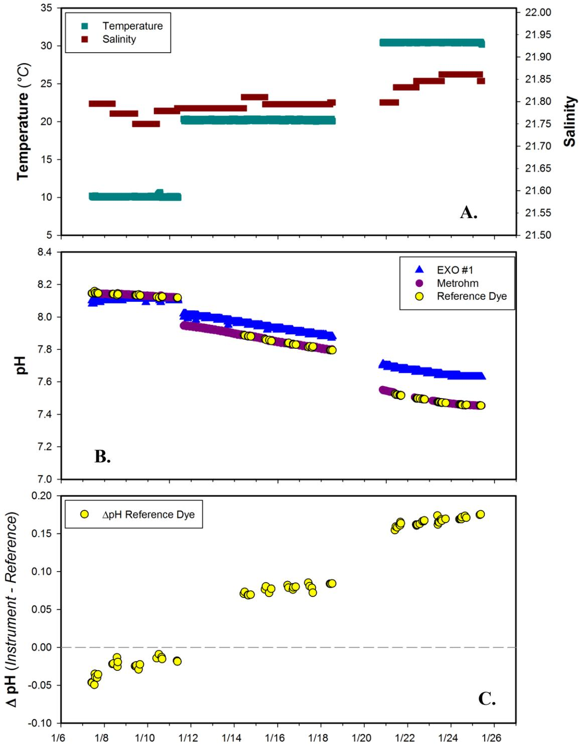
**Figure 7.** Time series results of the Xylem EXO- pH1 sensor for the stable portion of the brackish water trials. Measurements taken during temperature and pH shifts have been removed. Panel (a) temperature and salinity conditions during the brackish water trials; panel (b) measured pH from the EXO-pH1 plotted against both Metrohm and Dye reference pH measurements; and, panel (c) the difference between EXO and reference pH values.
