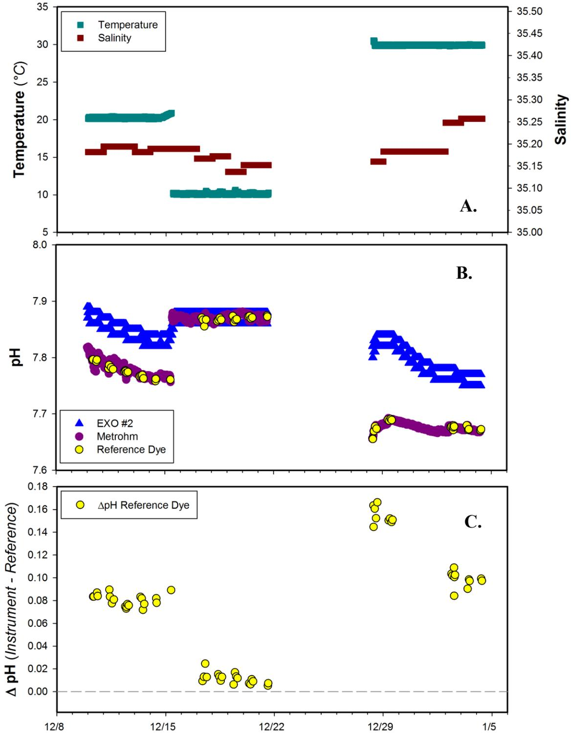
**Figure 6.** Time series results of the Xylem EXO-pH2 sensor for the stable portion of the seawater trials. Measurements taken during temperature and pH shifts have been removed. Panel (a) temperature and salinity conditions during the seawater trials; panel (b) measured pH from the EXO-pH2 plotted against both Metrohm and Dye reference pH measurements; and, panel (c) the difference between EXO and reference pH values.
