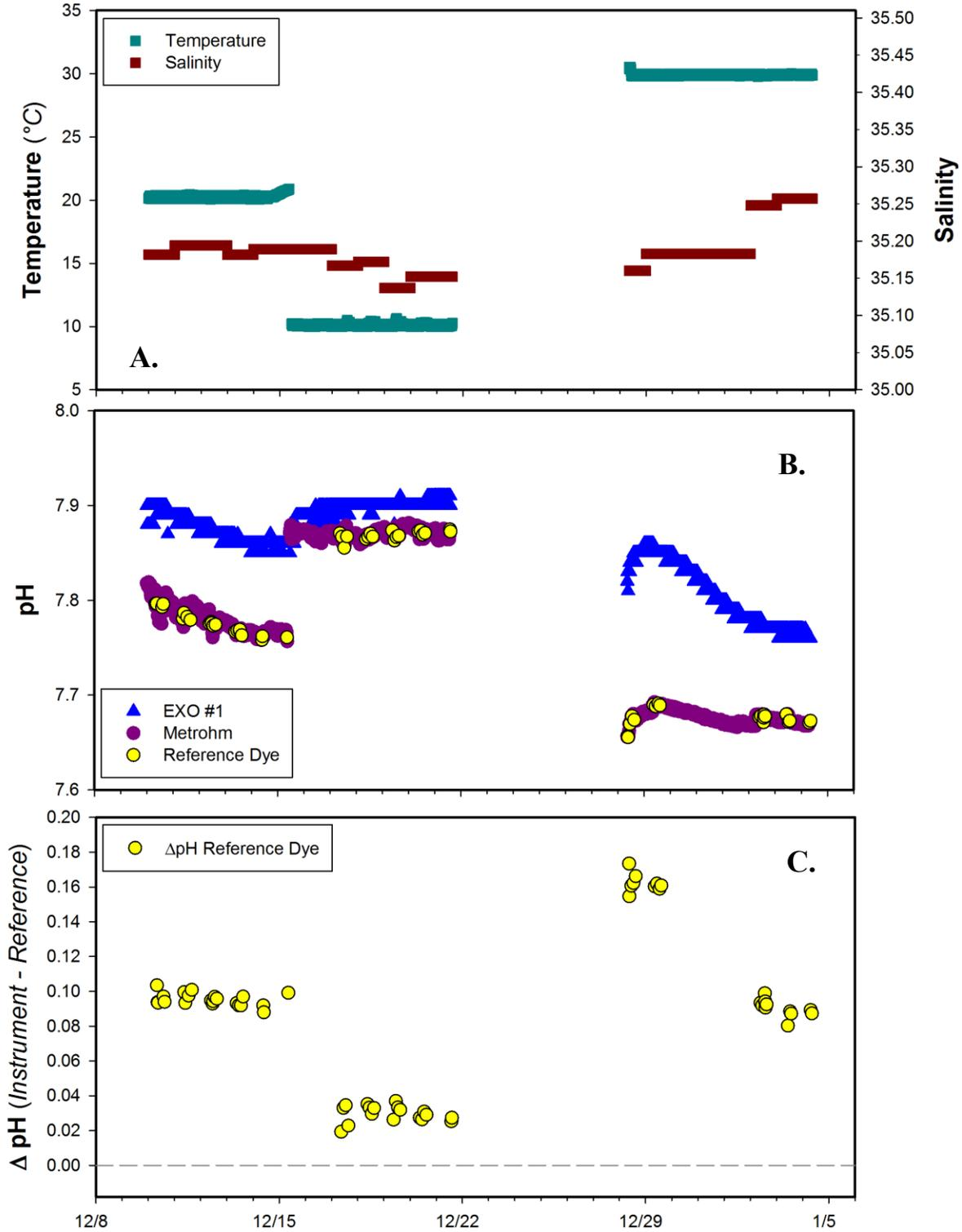
**Figure 5.** Time series results of the Xylem EXO-pH1 sensor for the stable portion of the seawater trials. Measurements taken during temperature and pH shifts have been removed. Panel (a) temperature and salinity conditions during the seawater trials; panel (b) measured pH from the EXO-pH1 plotted against both Metrohm and Dye reference pH measurements; and, panel (c) the difference between EXO and reference pH values.
