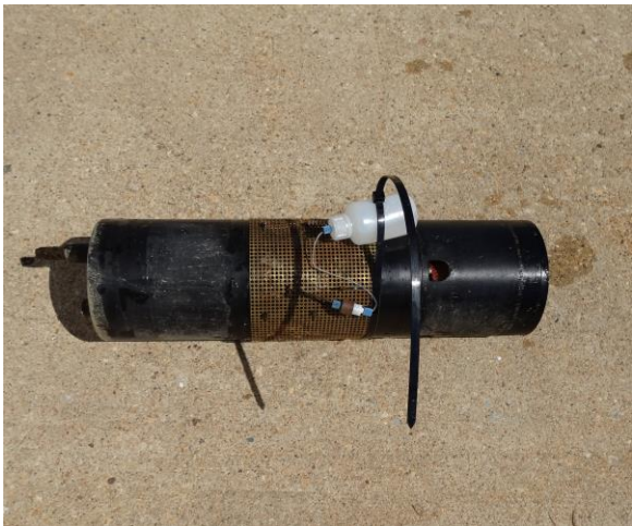
Photo 7. The SAMI pH prior to and following the 1 month deployment for the CBL field test.
