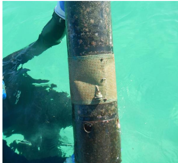
Photo 5. The SAMI pH prior to and following the 3 month deployment for the HIMB field test.
