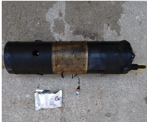
Photo 9. The SAMI pH prior to and following the 1 month deployment for the Great Lakes field test.
