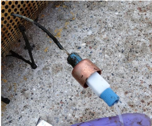
Photo 9. The SAMI pH prior to and following the 1 month deployment for the Great Lakes field test.
