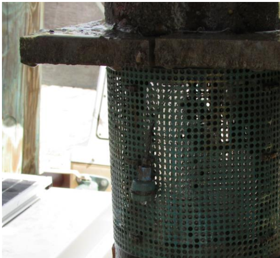
Photo 3. The SAMI pH prior to and following the 1 month deployment for the MLML field test.
