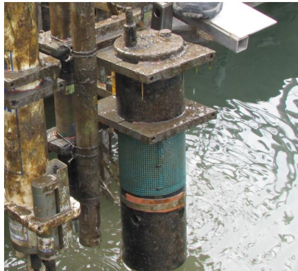
Photo 3. The SAMI pH prior to and following the 1 month deployment for the MLML field test.
