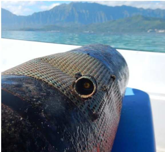
Photo 5. The SAMI pH prior to and following the 3 month deployment for the HIMB field test.
