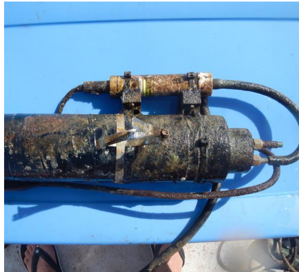
Photo 5. Satlantic SeaFET instrument deployed with SBE 5M pumping system prior to and following the 3 month HIMB field trial.
