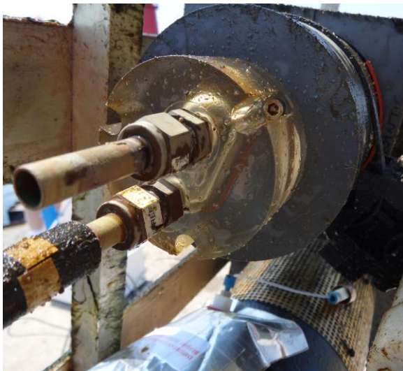
Photo 9. Satlantic SeaFET instrument deployed with SBE 5M pumping system prior to and following the 1 month Great Lakes field trial.
