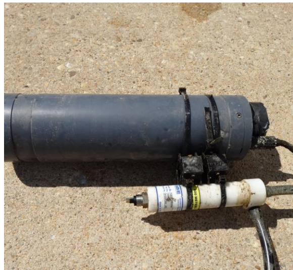
Photo 7. Satlantic SeaFET instrument deployed with SBE 5M pumping system prior to and following the 1 month CBL field trial.
