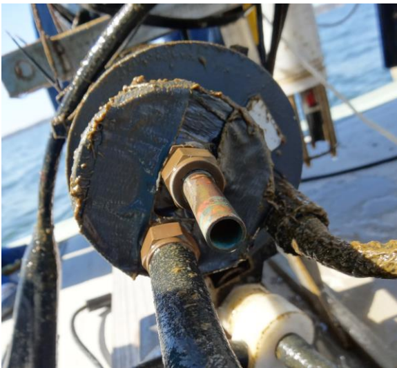
Photo 7. Satlantic SeaFET instrument deployed with SBE 5M pumping system prior to and following the 1 month CBL field trial.
