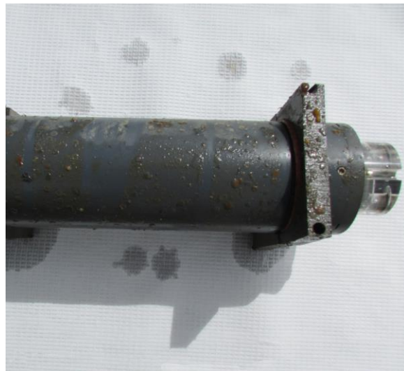
Photo 3. Satlantic SeaFET prior to and following one month deployment for the MLML field test.
