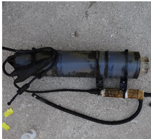
Photo 9. Satlantic SeaFET instrument deployed with SBE 5M pumping system prior to and following the 1 month Great Lakes field trial.
