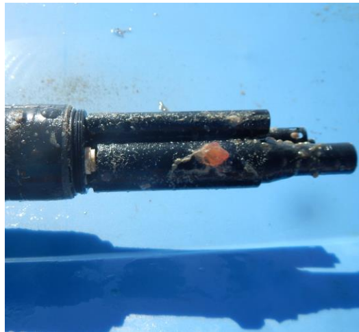
Photo 5. The Troll 9500 prior to and following 3 month deployment for the HIMB field test.
