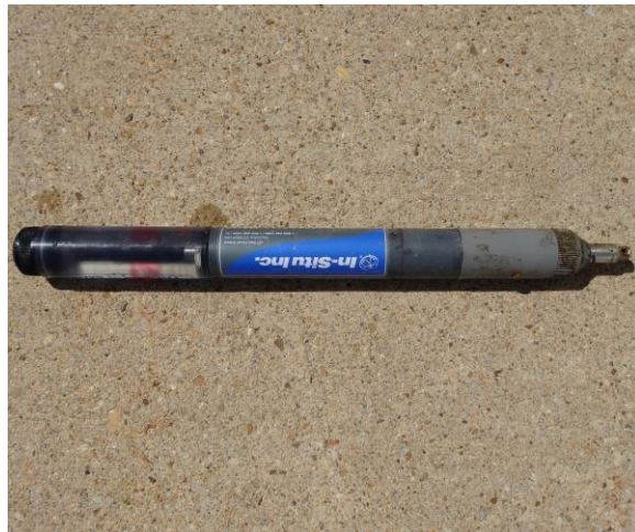
Photo 7. The Troll 9500 prior to and following deployment the 1 month deployment for the CBL field test.
