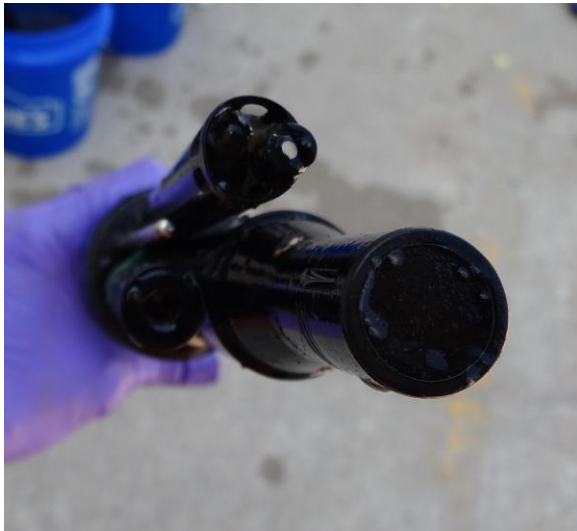
Photo 9. The Troll 9500 prior to and following the 1 month deployment for the Great Lakes field test.
