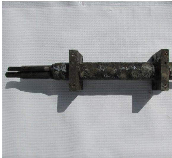
Photo 3. The Troll 9500 prior to and following the 1 month deployment for the MLML field test.
