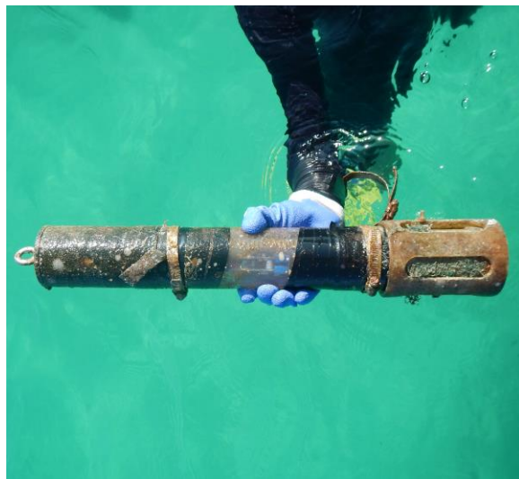
Photo 4. The Eureka Manta prior to and following the 3 month deployment in Kaneohe Bay. Note the broken bulb in the close up post deployment photo.
