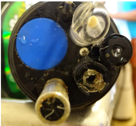
Photo 4. The Eureka Manta prior to and following the 3 month deployment in Kaneohe Bay. Note the broken bulb in the close up post deployment photo.
