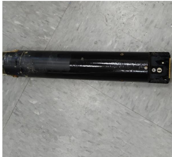
Photo 7. The CSI pH sensor prior to and following the 1 month deployment for the CBL field test.
