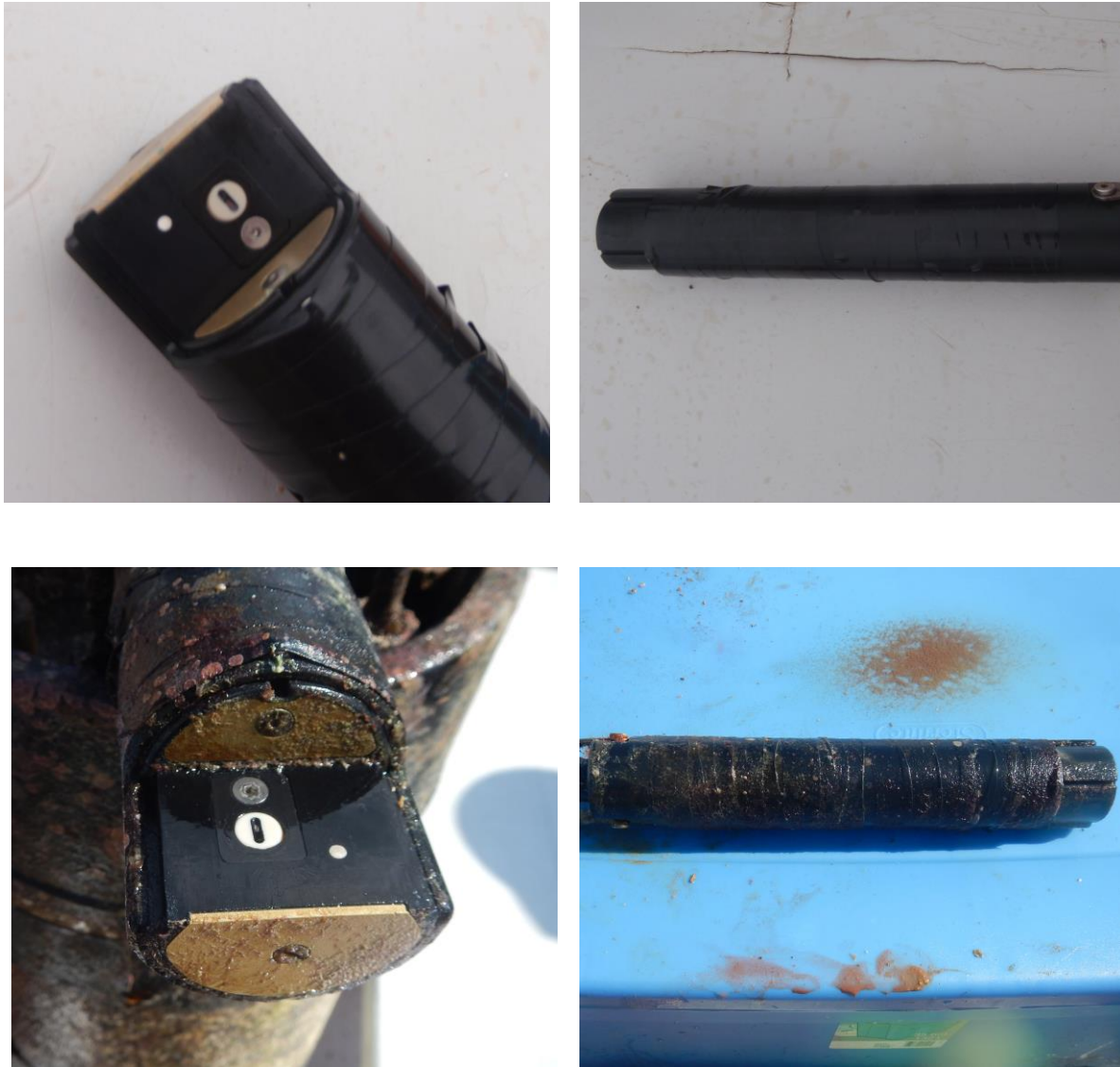
Photo 5. The CSI pH sensor prior to and following the 2 month deployment in Kaneohe Bay for the HIMB field test.
