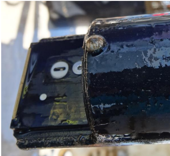
Photo 7. The CSI pH sensor prior to and following the 1 month deployment for the CBL field test.
