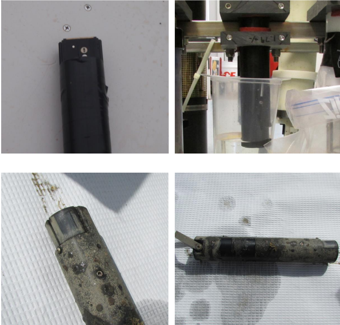
Photo 3. The Campbell Scientific pH sensor prior to and following the 1 month deployment for the MLML field test.
