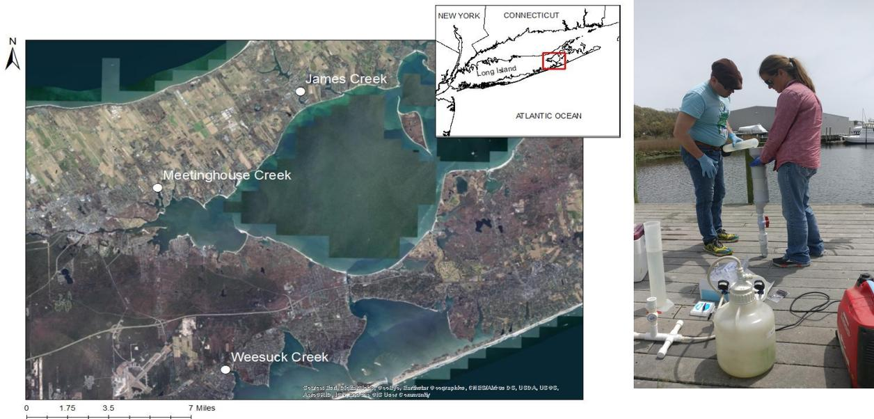
Figure 17. *Left*: Sample sites on Long Island. *Right*: Concentration of whole water (3L capacity) via PVC device.
