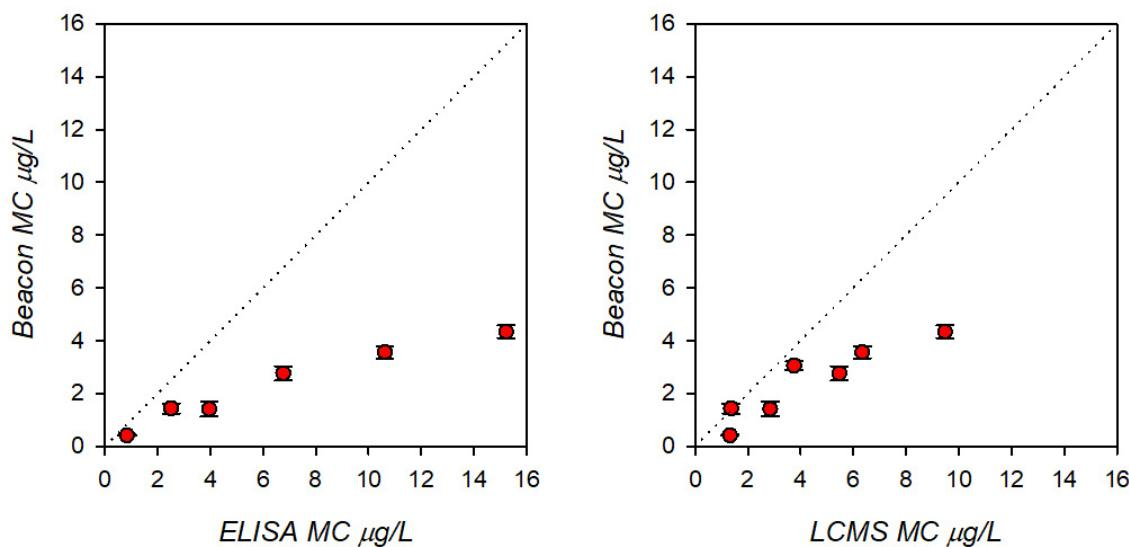
Figure 9. A cross plot of Beacon measurements compared to reference ELISA and LCMS-LR microcystin measurements for the laboratory range trial. Error bars represent one standard deviation ( $n = 2$ ) for Beacon and ELISA, LCMS-LR have no error bars as there was a single value.
