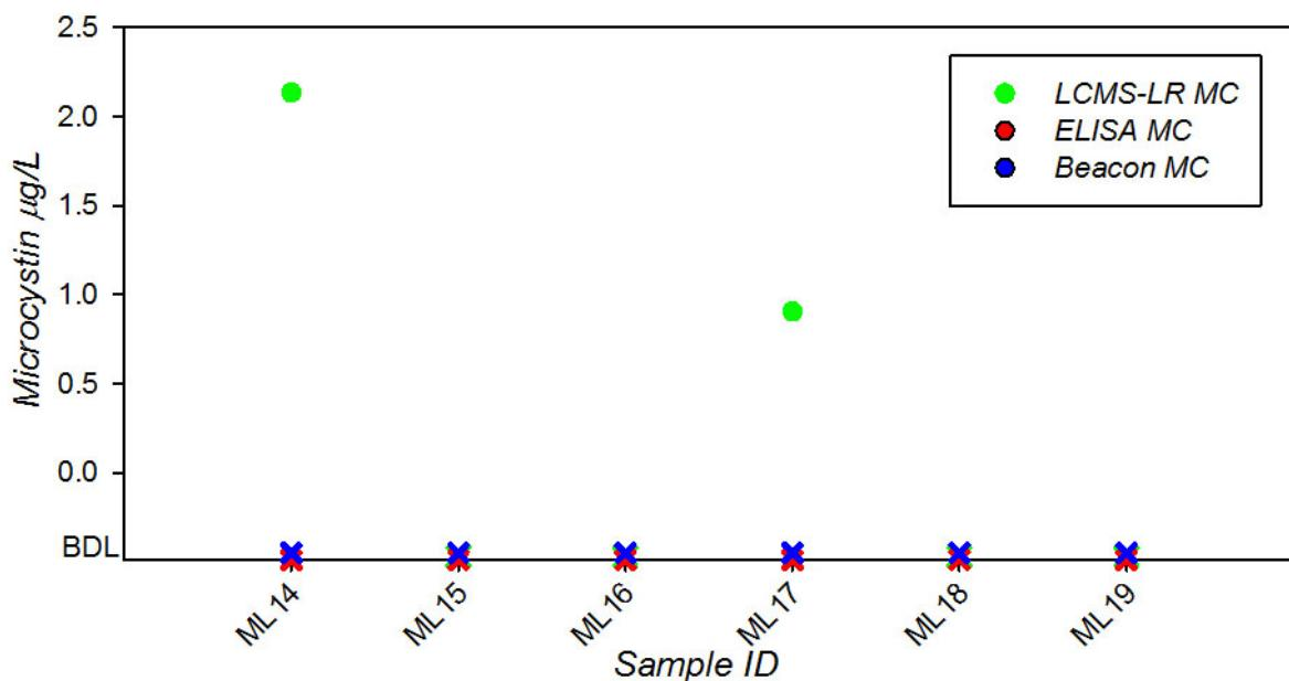
Figure 18. MLML Pinto and El Estero Lakes (ML 15) comparison of instrument (blue), reference ELISA (red) and LCMS-LR (green) whole microcystin data. Error bars denote one standard deviation for Beacon ( $n=2$ ) and ELISA ( $n=2$ ), LCMS-LR has no error bars as it was a single value. Beacon BDL < 0.5  $\mu\text{g}/\text{L}$ . Samples ML18 and ML19 are independently collected field duplicates.
