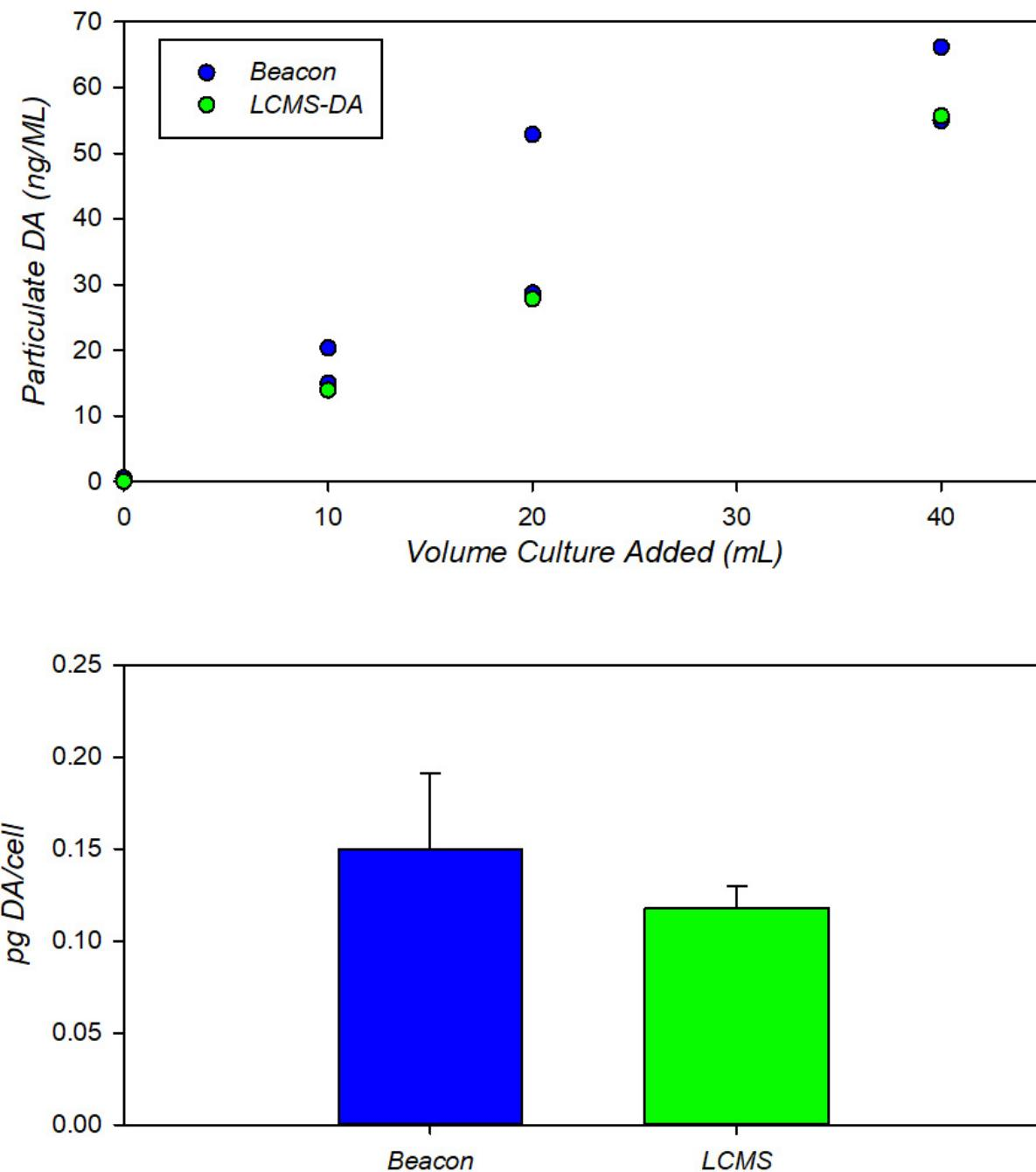
Figure 20. pDA analysis of toxic *Pseudo-nitzschia multiseries* laboratory cultures. *Top Panel*: Increasing volumes of a stock *P. multiseries* cultures were added to 0.2 $\mu$  filtered seawater and 100 mL of well mixed culture were collected onto GFF filters. *Bottom Panel*: Normalization of pDA measurements to *P. multiseries* cell abundance in each sample yielded similar estimates of *P. multiseries* cellular DA quotas.
