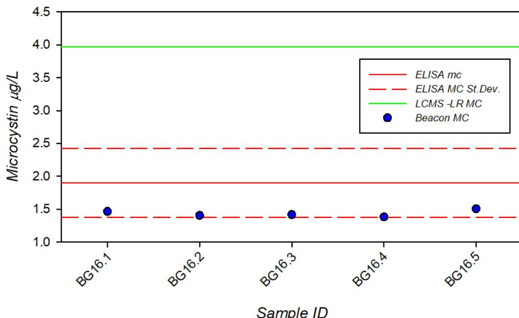
Figure 10. Results of the precision trial laboratory test using repeated measurement of a diluted certified MC standard to a targeted concentration of 1.5 µg/L, the ELISA estimated the concentration at  $1.9 \pm 0.53$ .
