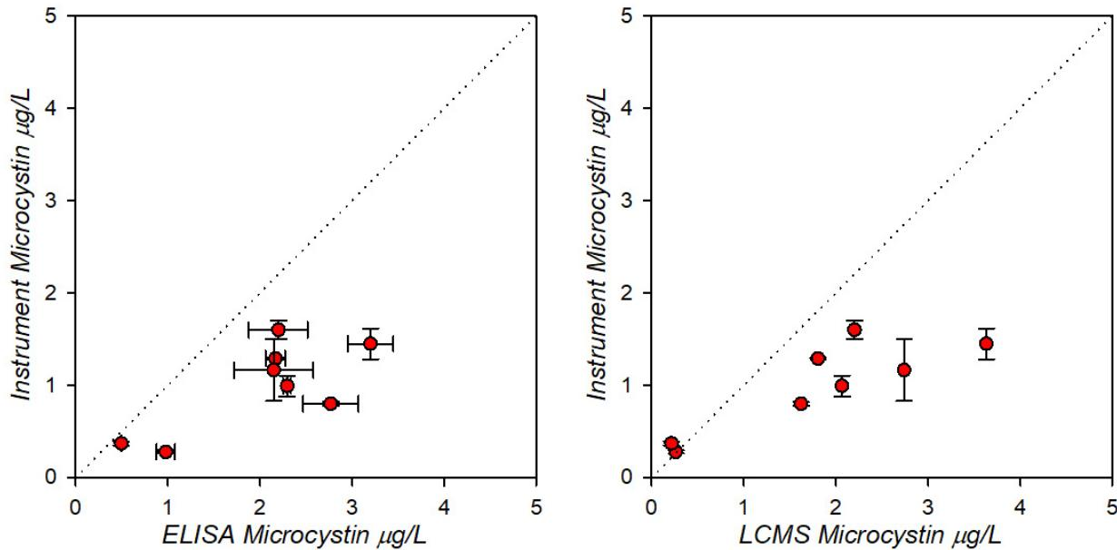
Figure 14. Western Lake Erie field response plot of Beacon compared to the ELISA (left) and LCMS-LR (right) whole water reference data. Error bars represent one standard deviation for Beacon and ELISA (n=2), LCMS-LR has no error bars as there was only one value. Data below detection is not included.
