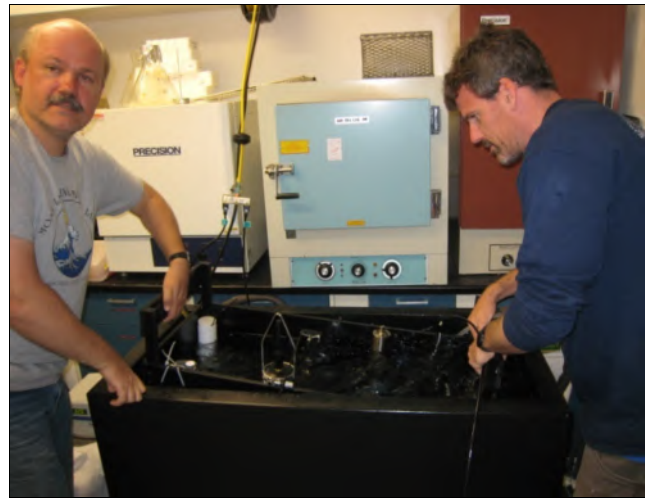
Figure 1. Analytical instrumentation (Portasal 8410A) used for laboratory analysis of salinity reference samples and one of the test baths and instrument racks used for the laboratory tests.
