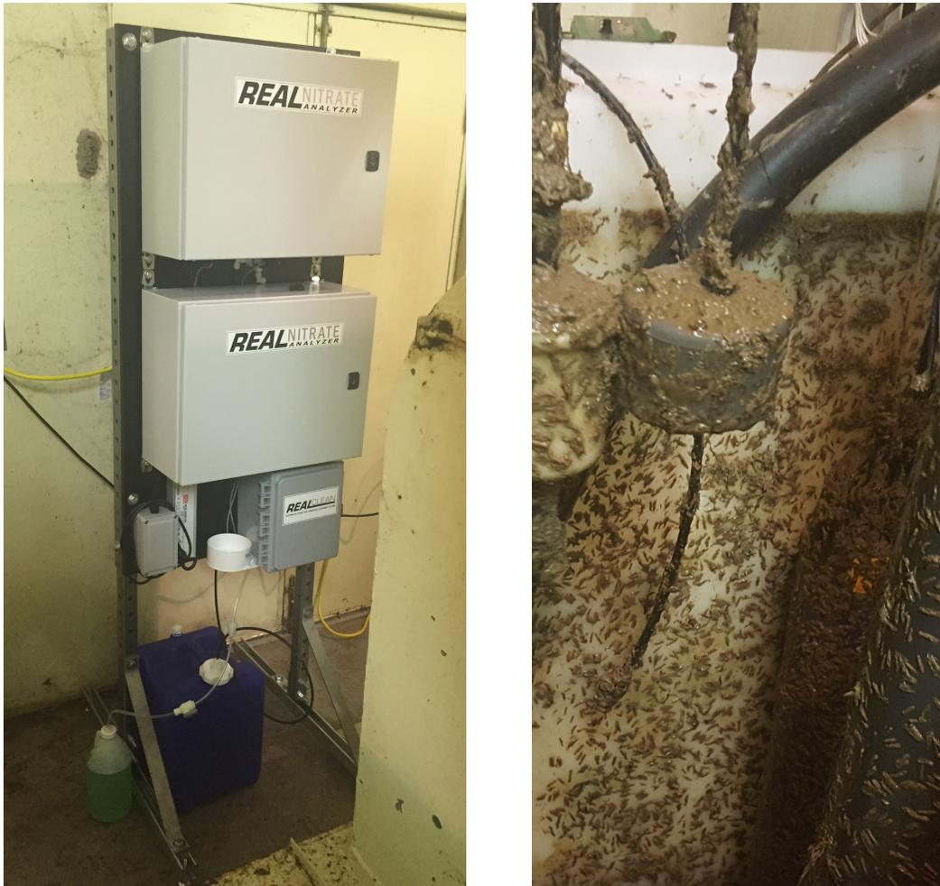
**Figure 12.** Photographs of the Real-NO<sub>3</sub> nitrate analyzer and the filter intake from the flow-through test tank following a 32 day field test in the Maumee River.
