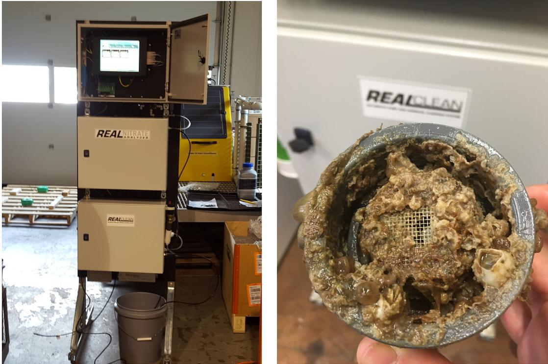
**Figure 17.** Photographs of the Real-NO<sub>3</sub> instrument prior to and following the CBL field trial.
