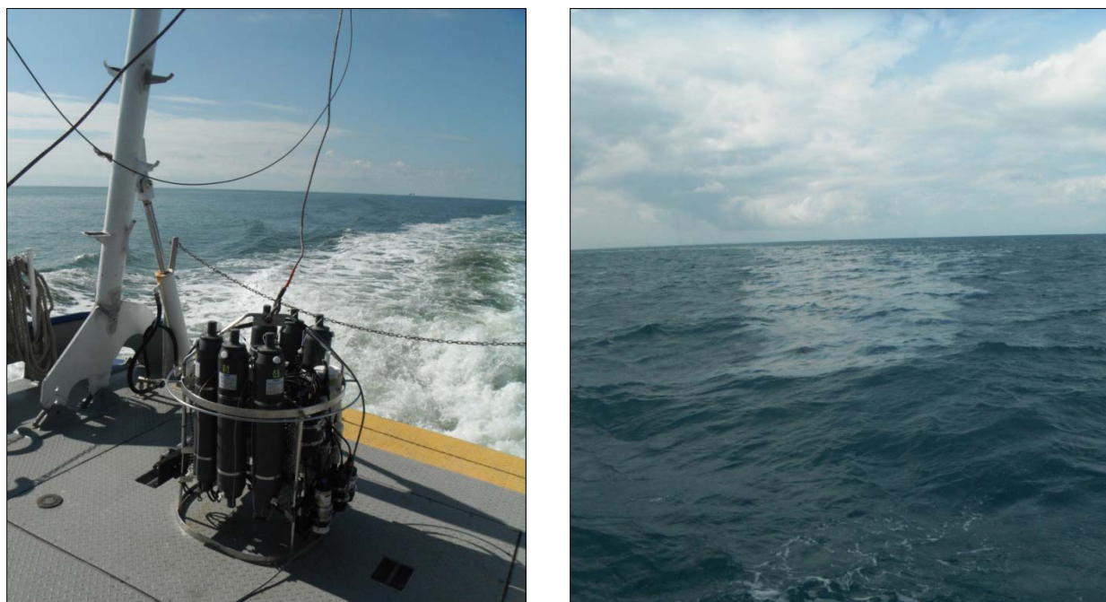
Photo 10. Vertical Profiling Rosette and visible surface oil slick above location of submerged, leaking barge.
