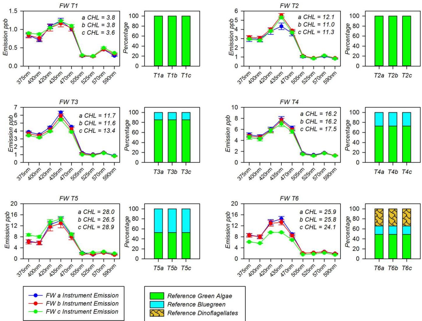
Figure 12. Algal classification from microscope counts on preserved reference samples compared to emission spectra of the JFE. Algal counts were grouped at the functional class level and represented as a percentage of biovolume. Each row represents three timepoint replicates of the same batch of algae and matrix conditions.
