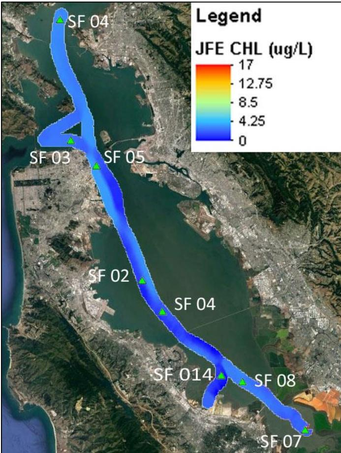
Figure 19. Chlorophyll data contours from the JFE during the underway surface mapping survey in San Francisco on the USGS *R/V Peterson*. Green triangles denote isolated, comparative sampling stations.
