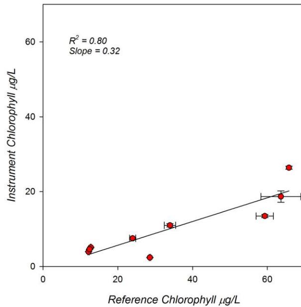
Figure 17. Response plot for the Great Lakes lab test of the JF compared to reference samples. The instrument values were obtained by averaging over 2 minutes. The blue lines represent the linear regression of the data.
