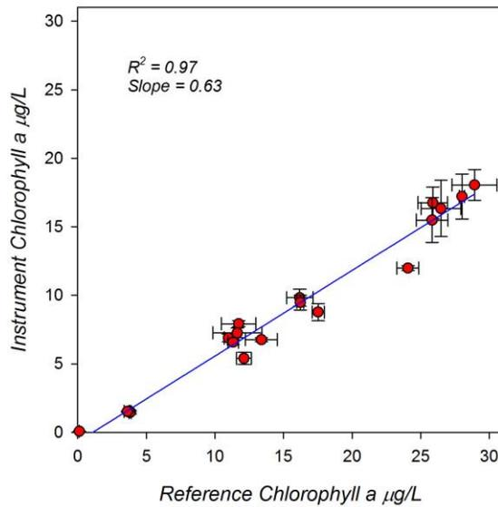
Figure 11. Cross plot of instrument readings versus extracted reference sample pigments for chlorophyll a during the June 28 freshwater algal mixtures lab trials. The blue lines represent the linear regression of the data.
