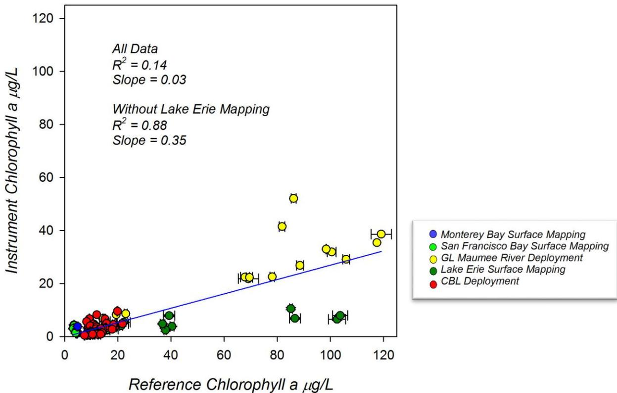
Figure 46. Global response plot for the JFE CHL estimation compared to extracted chlorophyll for all five ACT field trials. The blue lines represent the linear regression excluding the data from the Lake Erie Surface Mapping (GL SM, denoted with dark green circles).
