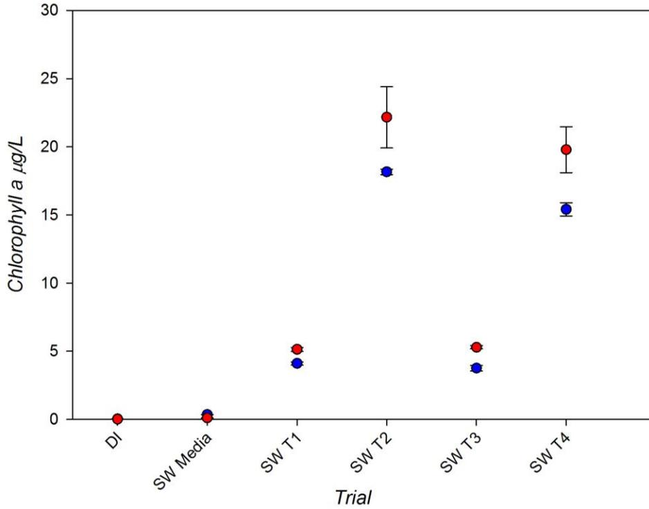
Figure 4. Plot of instrument (blue) and reference (red) measurements of chlorophyll-a in the saltwater individual algae tests including background readings for DI and saltwater media. The plotted reference values represent the average and standard deviation of the two reference measurements taken at the beginning and end of the exposure period. Instrument estimations were generated from the 1 second readings averaged over 1 minute, following an equilibration time of 3 minutes.
