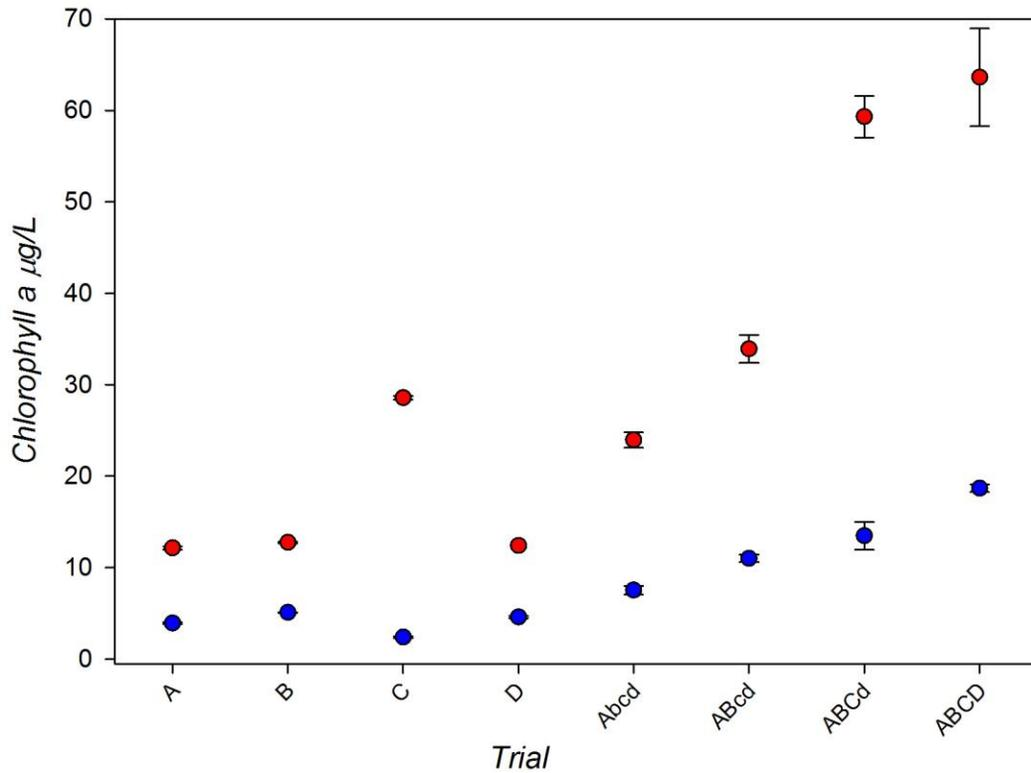
Figure 16. Plot of instrument (blue) and reference (red) measurements of chlorophyll-a in the Great Lakes laboratory trial over 4 individual algae cultures, 4 mixtures and a CDOM and turbidity addition. One reference measurement was made at each level and instrument was averaged over 5 minute periods.
