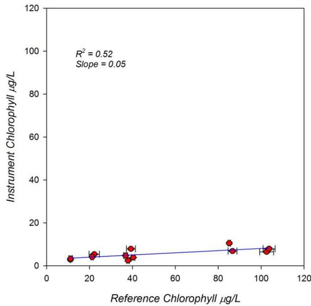
Figure 32. Lake Erie surface mapping response plot for the JFE chlorophyll measurements compared to reference chlorophyll a.
