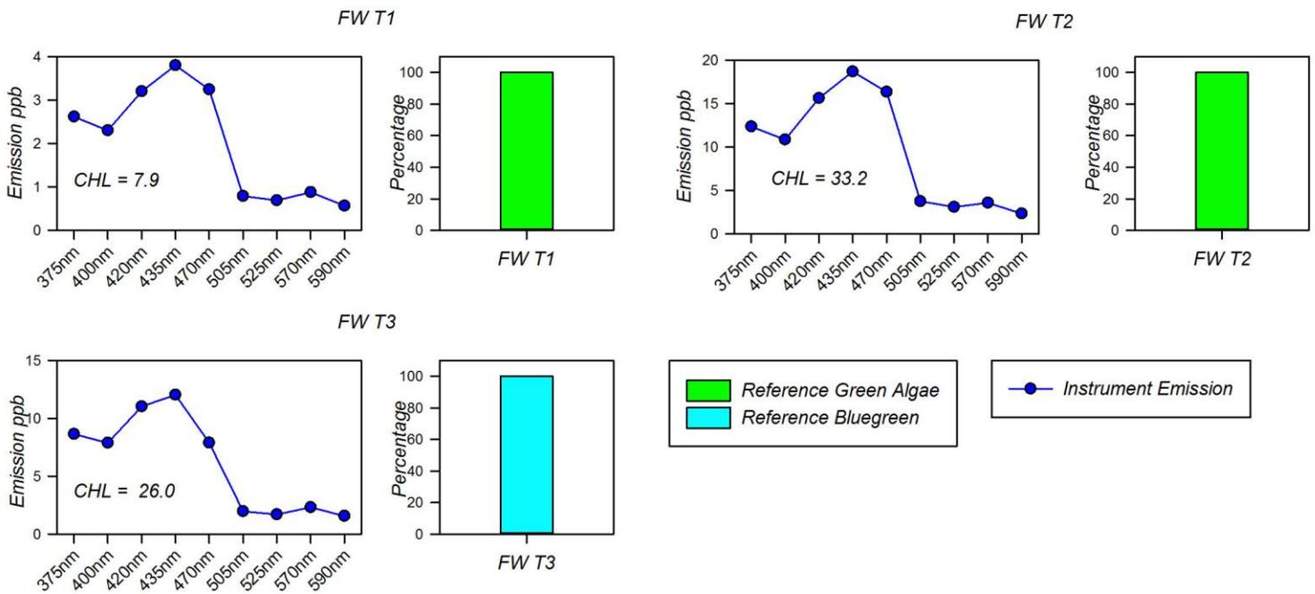
Figure 3. Algal classification from microscope counts on preserved reference samples as a percentage of biomass grouped at the functional class level, compared to the JFE emission measurements at each excitation wavelength. Algal counts were grouped at the functional class level.
