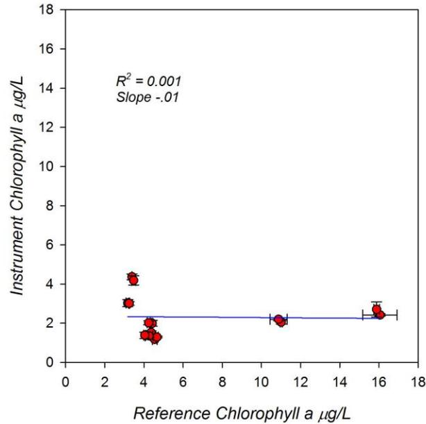
Figure 22. San Francisco Bay surface mapping response plot of the JFE chlorophyll measurements compared to reference chlorophyll measured.
