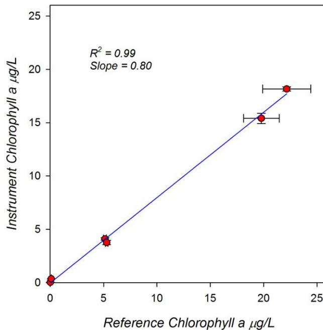
Figure 5. Cross plot of instrument readings versus extracted reference sample pigments for chlorophyll-a during the saltwater individual algae lab trials.
