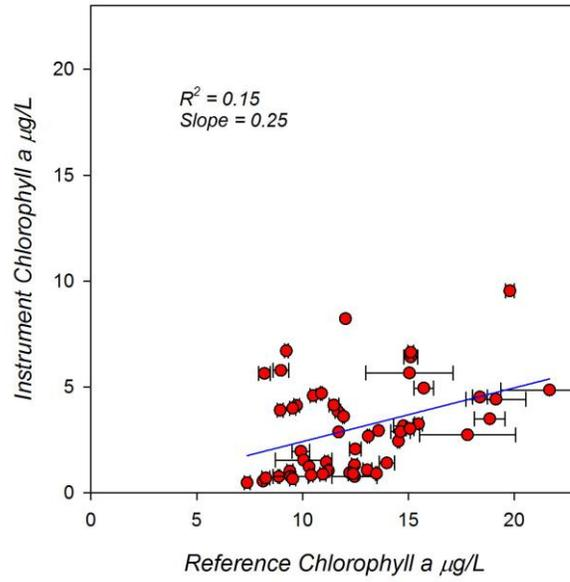
Figure 43. Cross plot of JFE and reference sample measurements during the CBL field deployment.
