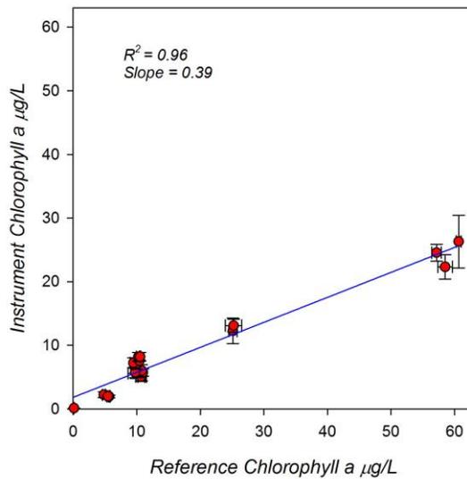
Figure 14. Response plot for the freshwater algae addition lab trial of the JFE chlorophyll a compared to reference samples. The blue lines represent the linear regression of the data.
