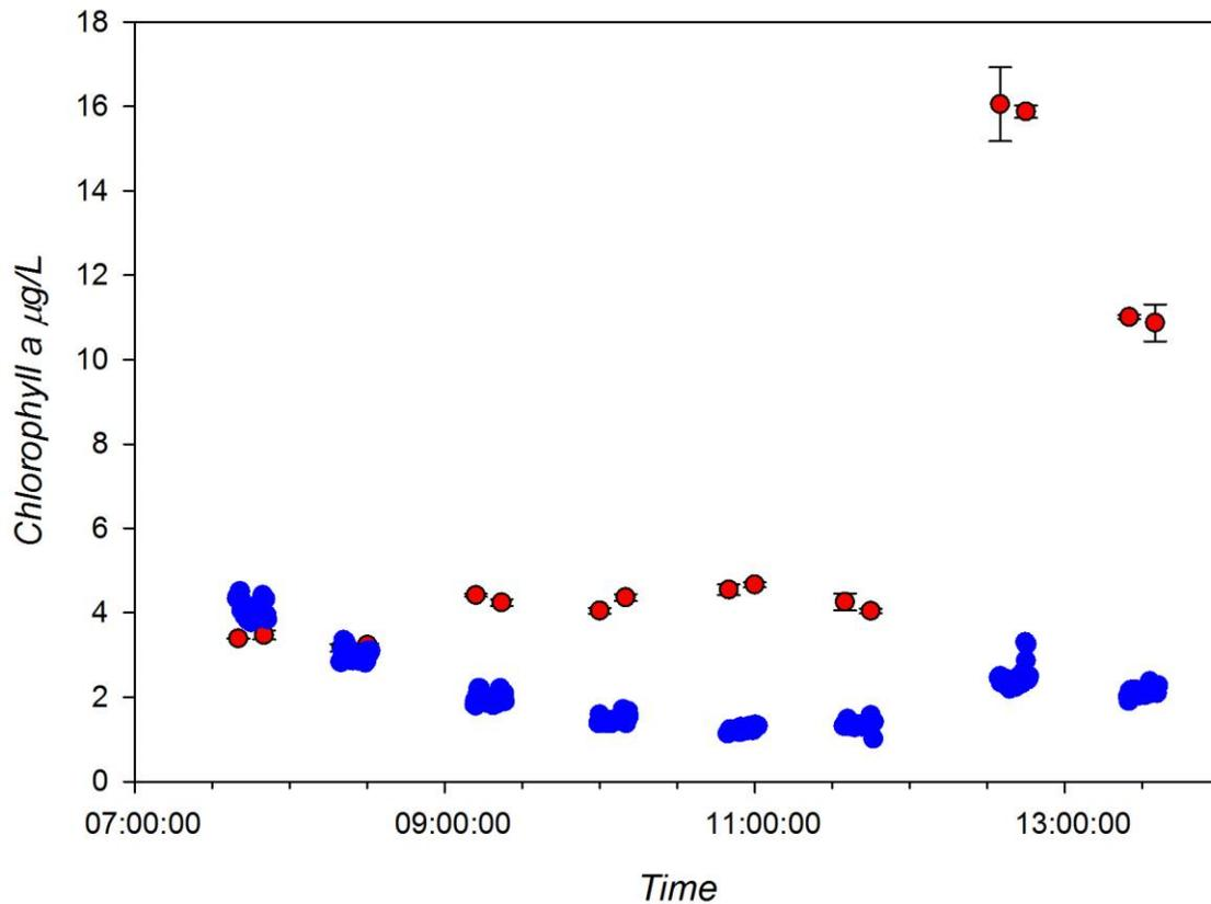
Figure 21. Plot of instrument (blue) and reference (red) measurements of chlorophyll a during San Francisco Bay surface mapping. Two reference measurements were made at each station, the instrument data was averaged over 2 minutes bracketing the reference samples.
