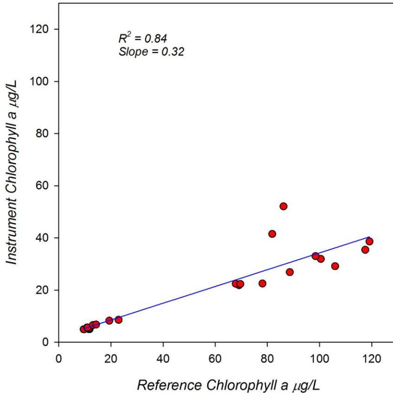
Figure 37. Cross plot of JFE and reference sample chlorophyll measurements during the Maumee River field deployment and resulting linear regression.
