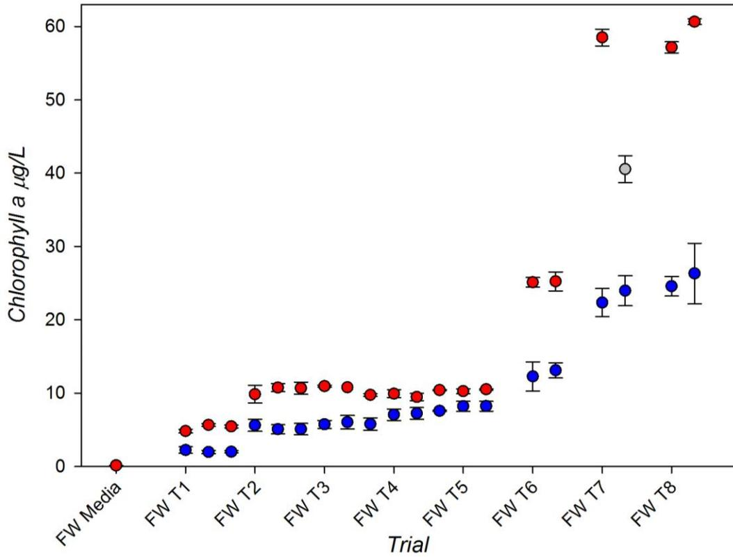
Figure 13. Plot of instrument (blue) and reference (red) measurements of chlorophyll a during the June 29<sup>th</sup> laboratory test with freshwater algae *Microcystis* and *Coelastrum*, and challenge additions of CDOM and turbidity. Three replicate reference measurements were made for trials 1-5, two replicates were made for trials 6-8, and one replicate for the blank media. JFE data was averaged over 1 minute bracketing each reference sample.
