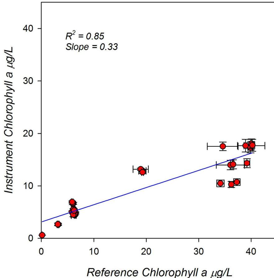
Figure 8. Cross plot of instrument readings versus extracted reference sample pigments for chlorophyll during the saltwater *Synechococcus* algae exposure with add in matrix challenges for CDOM and Turbidity. The blue line represents the linear regression of the data.
