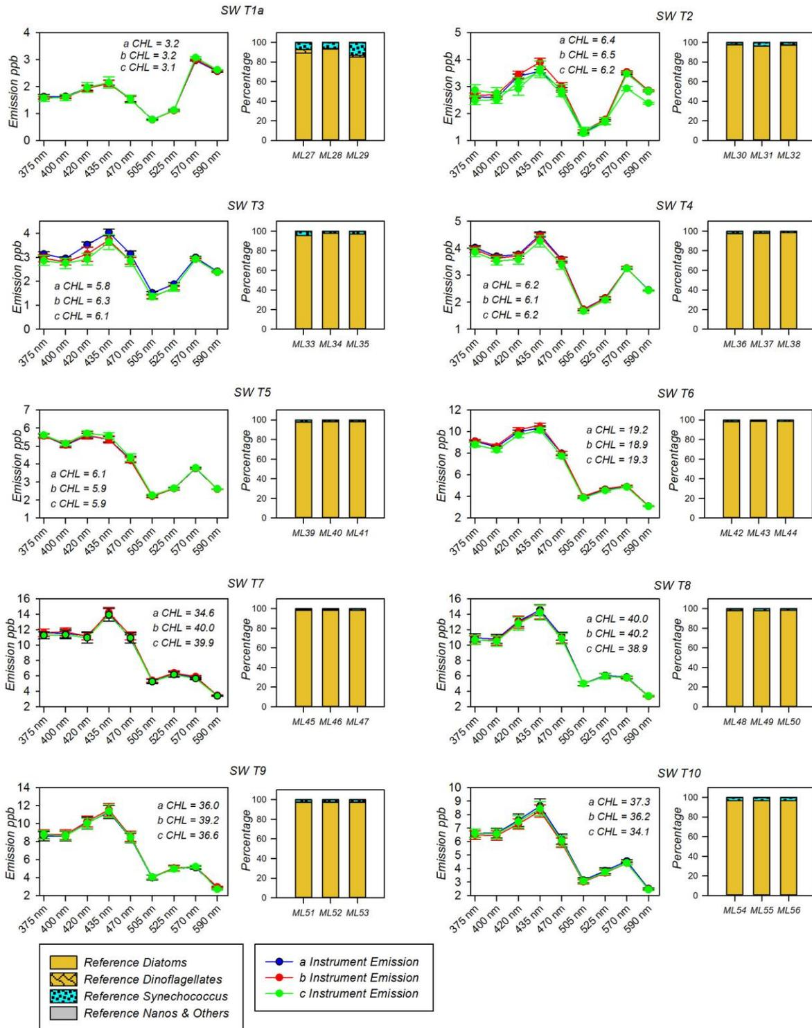
Figure 9. Algal classification from microscope counts on preserved reference samples compared to emission spectra of the JFE. Algal counts were grouped at the functional class level and represented as a percentage of biovolume. Each row represents three timepoint replicates of the same batch of algae and matrix conditions.
