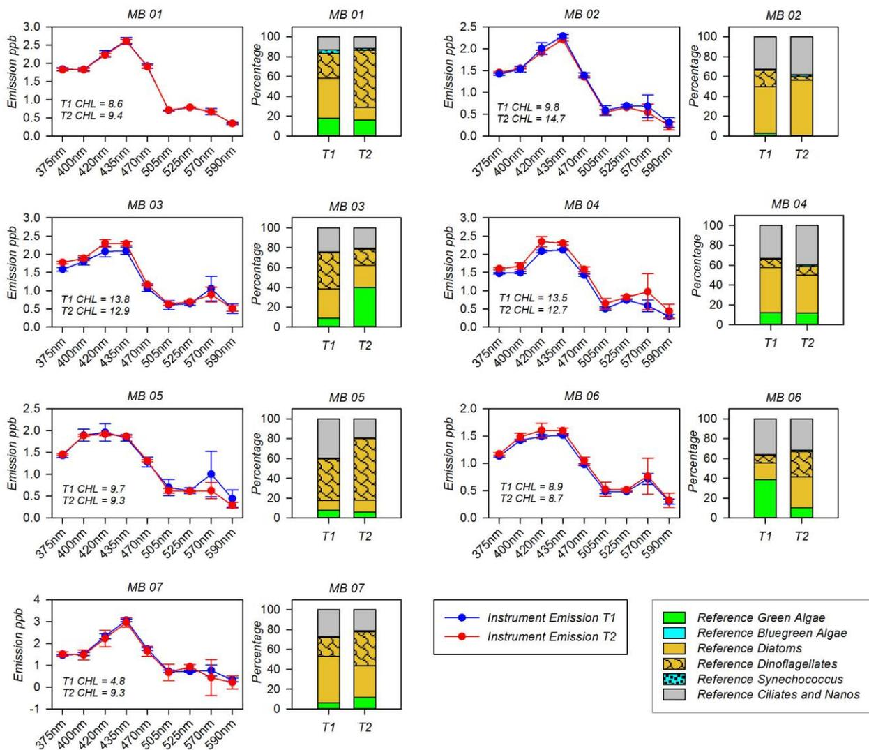
Figure 28. Algal classification from microscope counts on preserved reference samples compared to emission spectra of the JFE during the Monterey Bay underway mapping survey. Algal counts were grouped at the functional class level and represented as a percentage of biovolume. Each row represents two timepoint replicates of the same batch of algae and matrix conditions.
