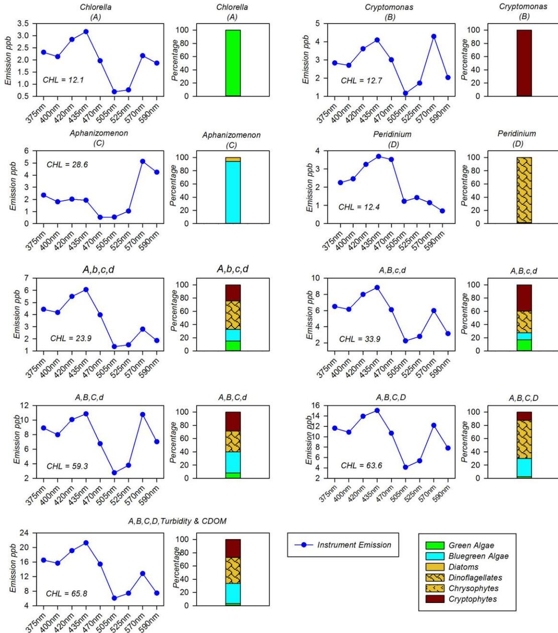
Figure 18. Algal classification from microscope counts on preserved reference samples compared to emission spectra of the JFE. Algal counts were grouped at the functional class level and represented as a percentage of biovolume.
