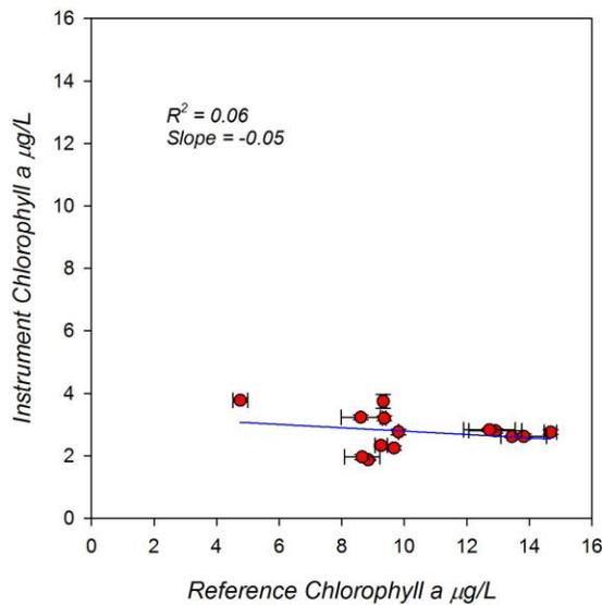
Figure 27. Monterey Bay surface mapping response plot of the JFE chlorophyll a measurements compared to reference chlorophyll a measured in µg/L.
