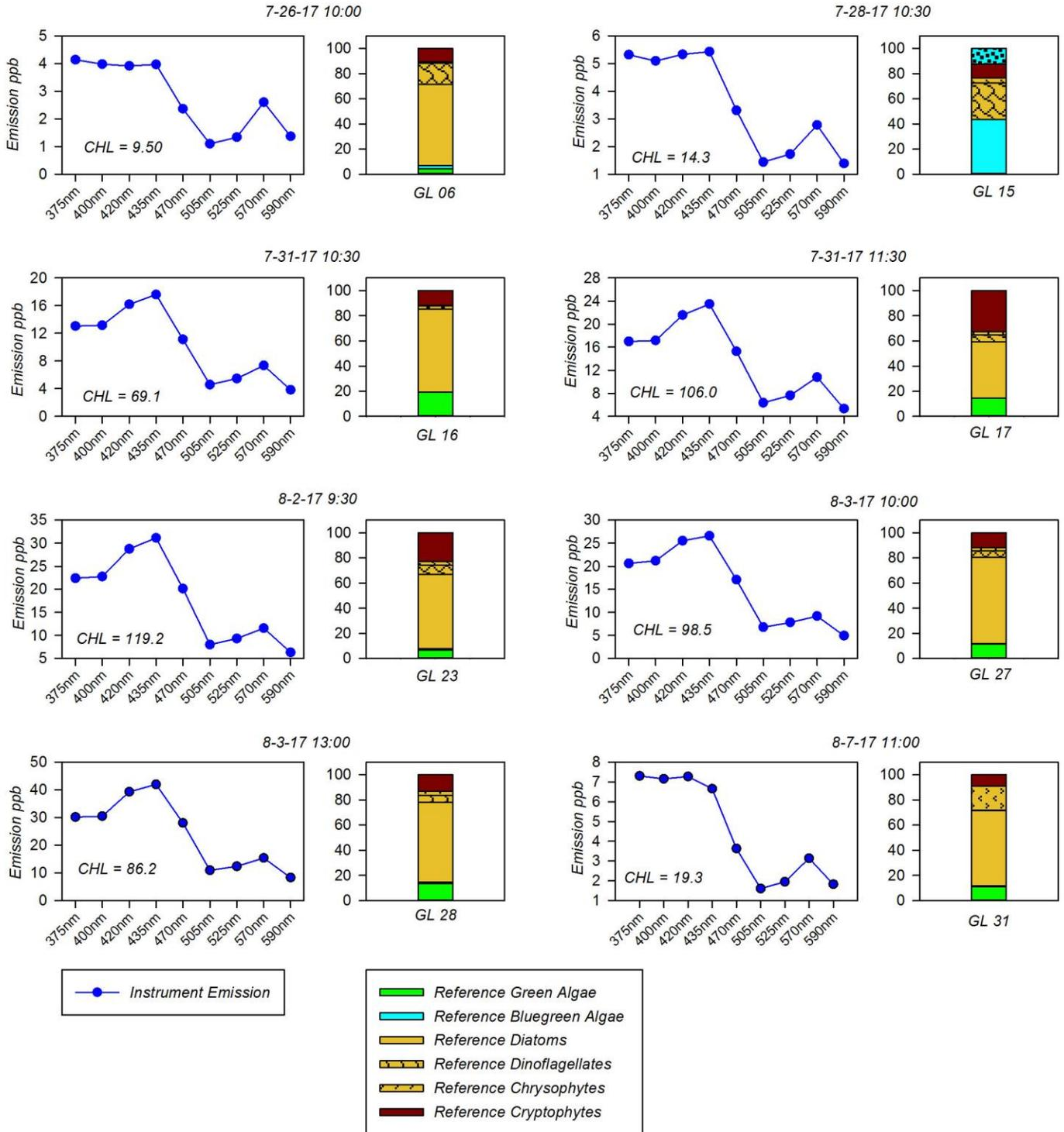
Figure 38. Reference cell counts as percentage of biomass compared to instrument algae categories as percentage of total CHL estimated by the JFE for the Maumee River field deployment test.
