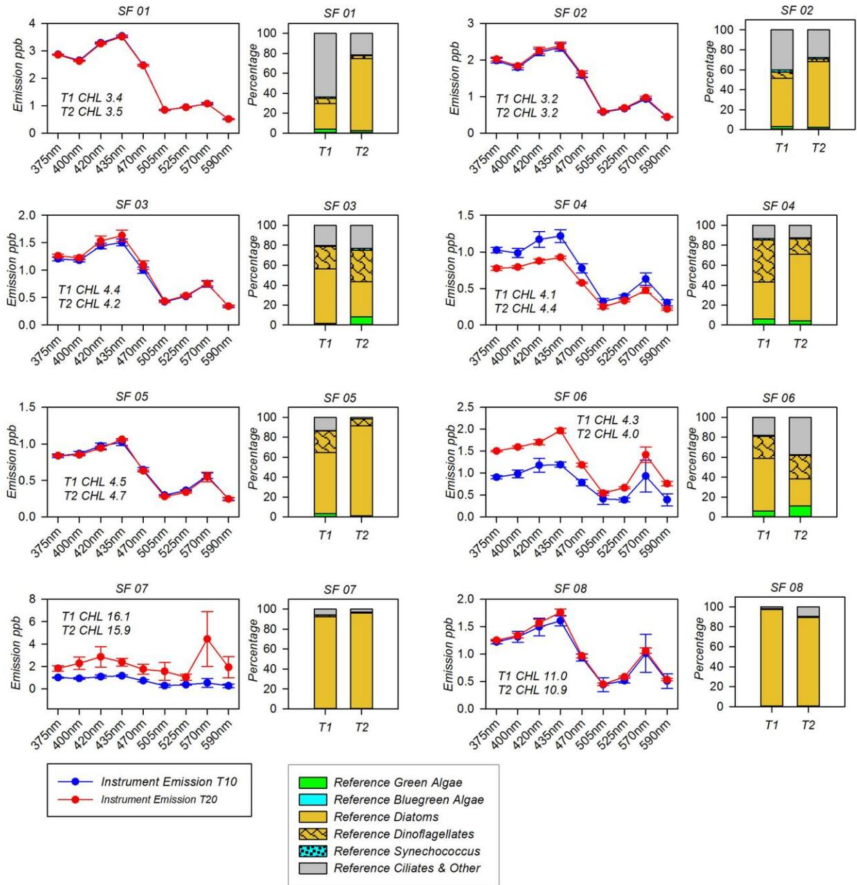
Figure 23. Algal classification from microscope counts on preserved reference samples compared to emission spectra of the JFE during the San Francisco Bay underway mapping survey. Algal counts were grouped at the functional class level and represented as a percentage of biovolume. Each row represents two timepoint replicates of the same batch of algae and matrix conditions.
