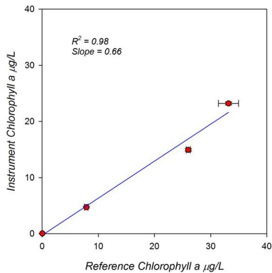
Figure 2. Cross plot of instrument readings versus extracted reference sample pigments for chlorophyll a during the freshwater individual algae lab trials.
