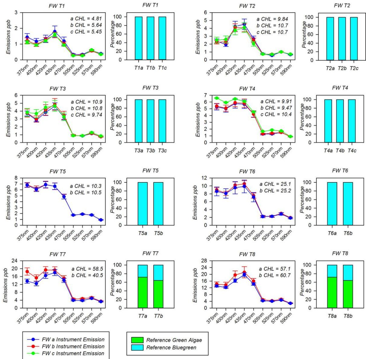
Figure 15. Algal classification from microscope counts on preserved reference samples compared to emission spectra of the JFE. Algal counts were grouped at the functional class level and represented as a percentage of biovolume. Each row represents two timepoint replicates of the same batch of algae and matrix conditions.
