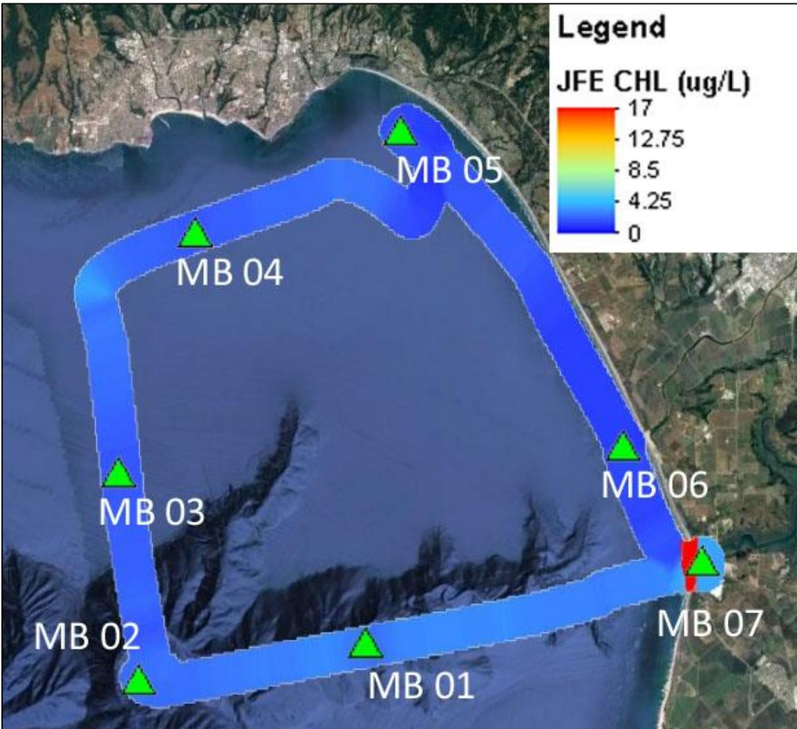
Figure 25. JFE continuous underway chlorophyll data during the surface mapping cruise in Monterey Bay. Triangles denote stations where the flow-through tank was isolated and comparative reference samples analyzed.
