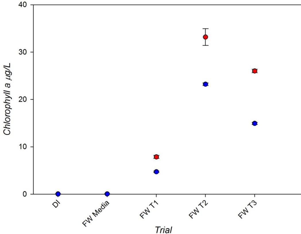
Figure 1. Plot of instrument (blue) and reference (red) measurements of chlorophyll a in the freshwater individual algae tests, including background readings for DI and the freshwater culture media. The plotted reference values represent the average and standard deviation of the two reference measurements taken at the beginning and end of the exposure period. Instrument estimations were generated from the 3 second readings averaged over 1 minute, following an equilibration time of 3 minutes.
