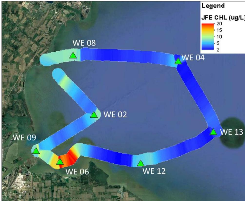
Figure 30. JFE continuous underway chlorophyll data during the surface mapping cruise in western Lake Erie. Triangles denote stations where the flow-through tank was isolated and comparative reference samples analyzed.
