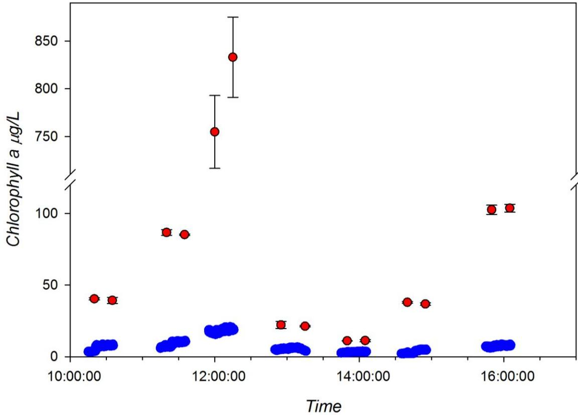
Figure 31. Time series plot of the JFE chlorophyll (blue) and reference (red) during surface mapping deployment on Lake Erie. Two reference measurements were made at each station, instrument data was averaged over 2 minutes bracketing the reference sample time.
