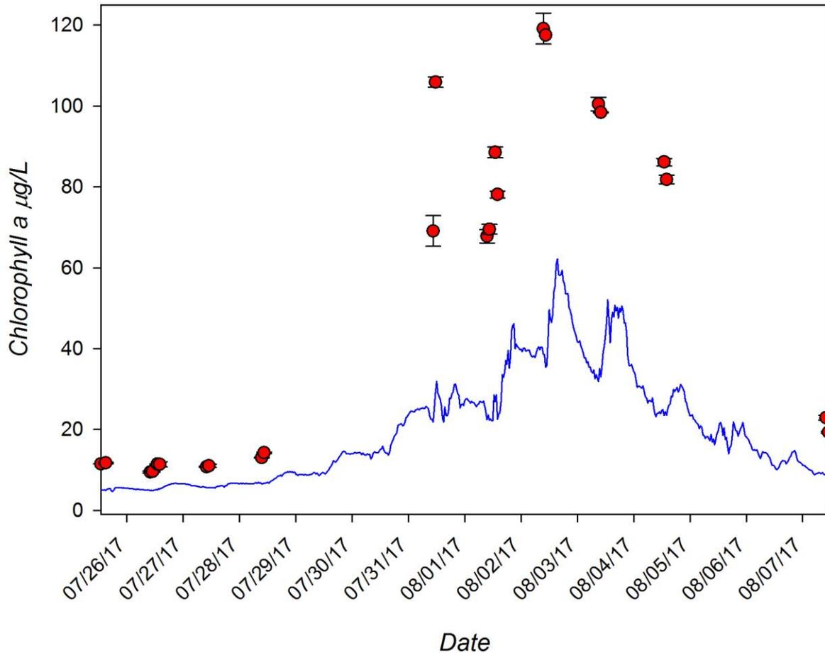
Figure 36. Time series plot of the JFE measurements (blue) and reference measurements (red) of chlorophyll a during the freshwater deployment in the Maumee River at Waterville, OH. Water samples were typically collected 1 hour apart, with either two or four samples on a given day.
