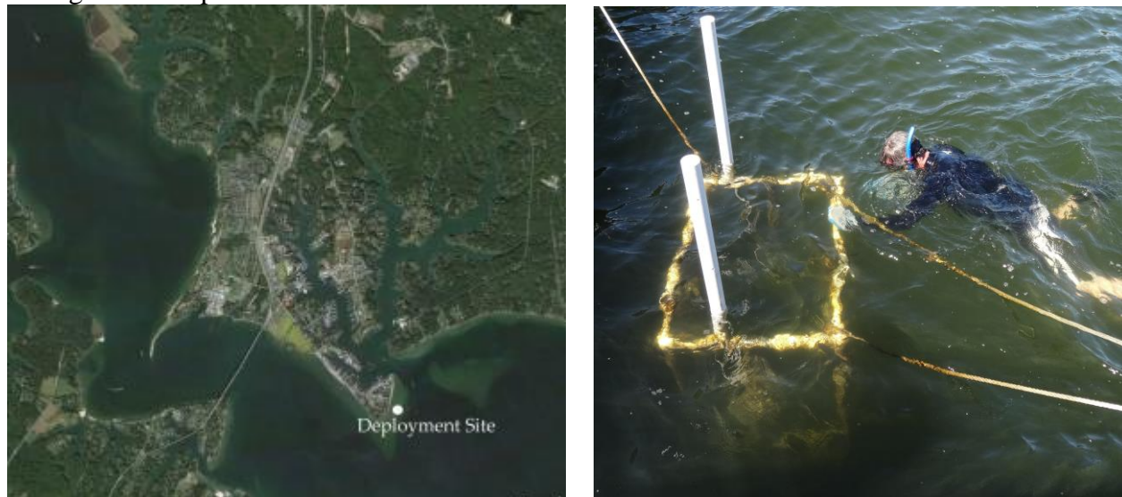
Figure 34. Aerial view of CBL deployment site ( left ) and instrument deployment rack with sensors submerged at a depth of 1 meter.
