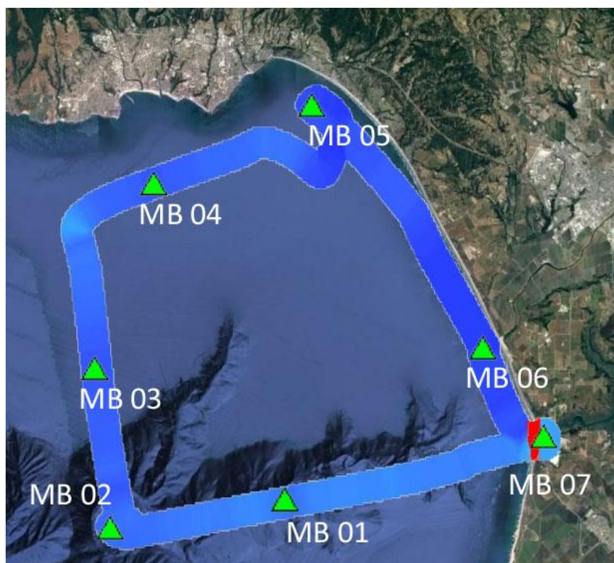
Figure 20. Surface mapping track during the continuous underway surface mapping cruise in on Monterey Bay onboard the R/V JH Martin . Triangles denote stations where the flow-through tank was isolated and comparative reference samples analyzed.
