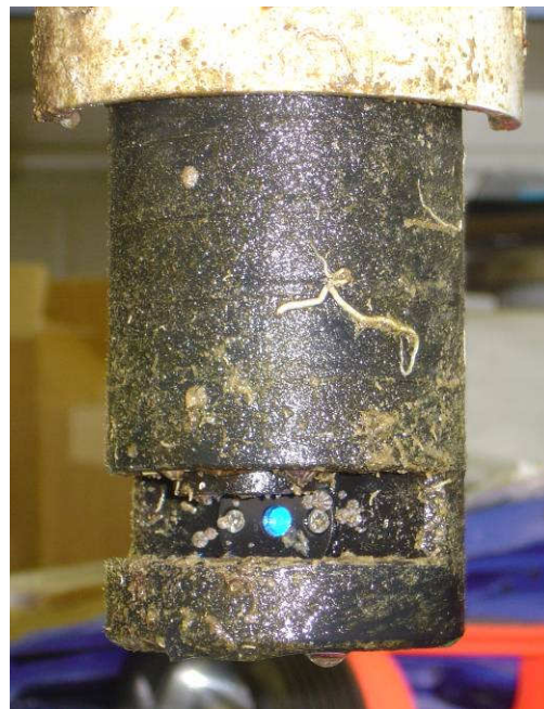
Sensor after the four weeks deployment.
