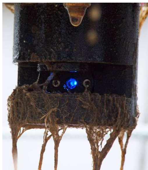
Sensor after the four weeks deployment.
