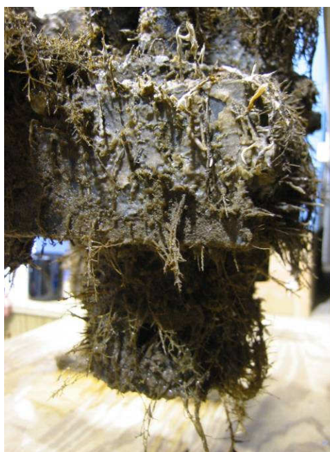
Sensor after the four weeks deployment.
