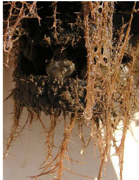
Sensor after the four weeks deployment.
