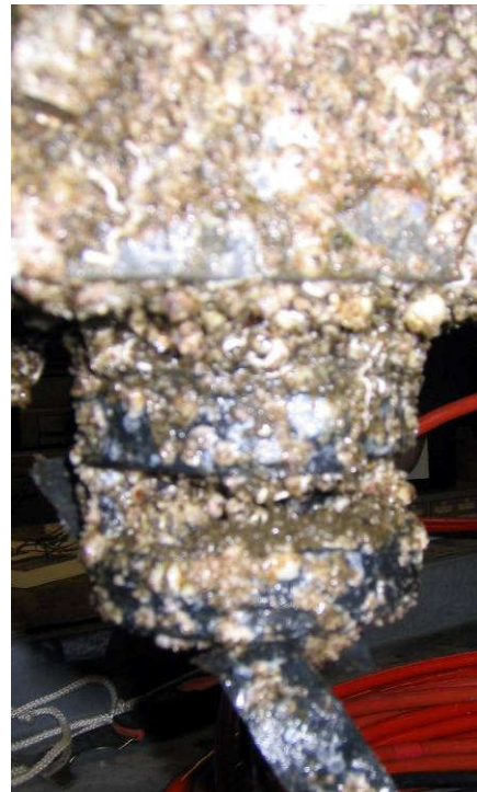
Sensor after the four weeks deployment.
