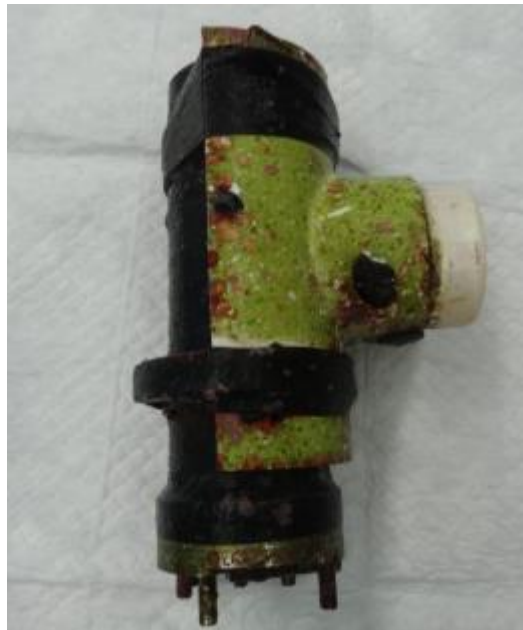
Photo 6. The JFE AroW-USB prior to and following the 18 week HIMB field trial.
