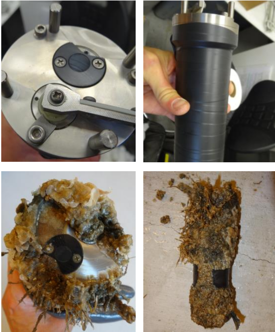
Photo 4. The JFE AroW-USB instrument and following the 12 week CBL field trial.
