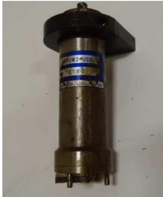
Photo 2. JFE AroW-USB prior to and following 15 week deployment under ice for the MTU field test.
