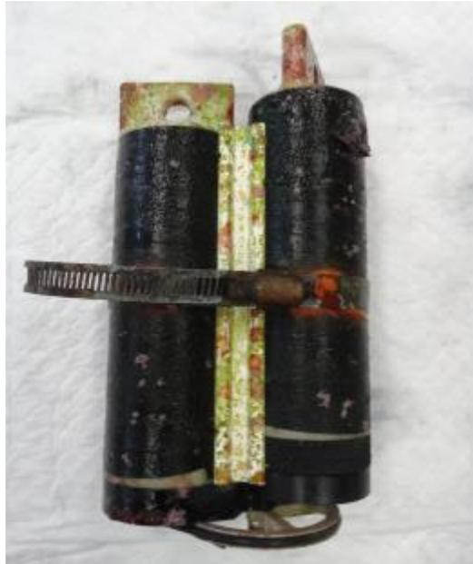
**Photo 6.** The PME miniDOT prior to and following the 18 week HIMB field trial.
