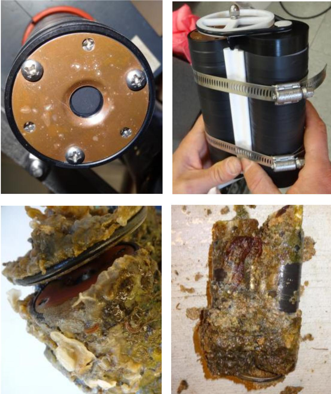
**Photo 4.** The PME miniDOT instrument before and following the 12 week CBL field trial.
