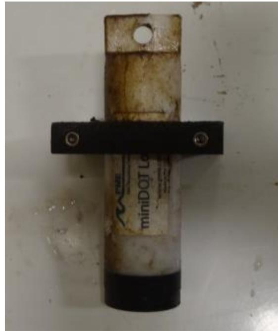
**Photo 2.** PME miniDOT prior to and following 15 week deployment under ice for the MTU field test.
