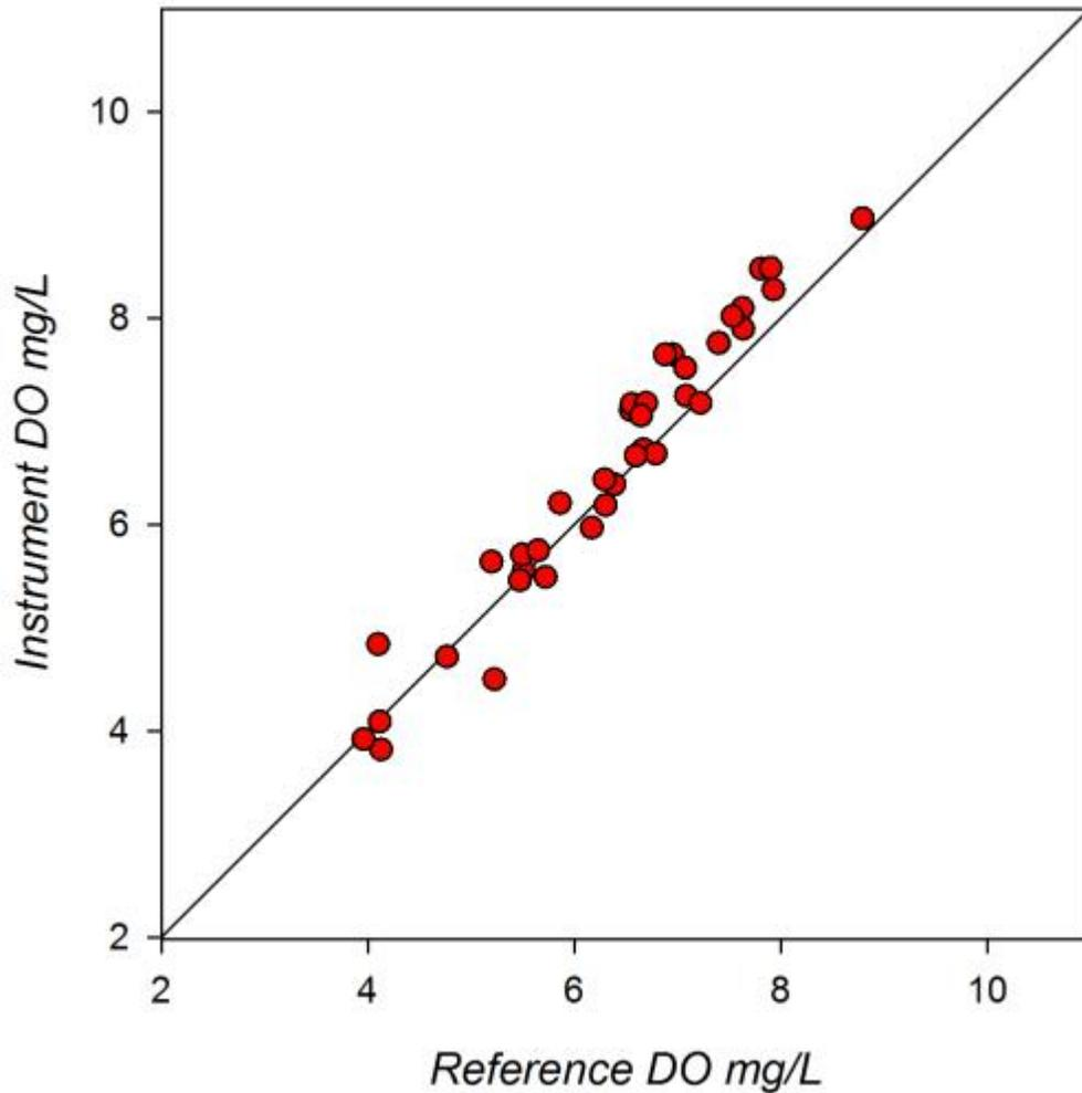
**Figure 7.** HIMB field response plot of HACH HL4 compared to reference DO samples determined by Winkler Titration. The plotted line represents a 1:1 correspondence.
