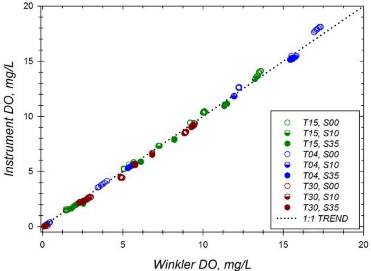
**Figure J.** Concordance of the Hach HL4 LDO (sn 0431) oxygen measures paired with discrete Winkler DO reference samples. In general readings are well correlated across a range of DO concentrations (hypoxic to supraoxic). Dotted line represents perfect agreement between the two measures.
