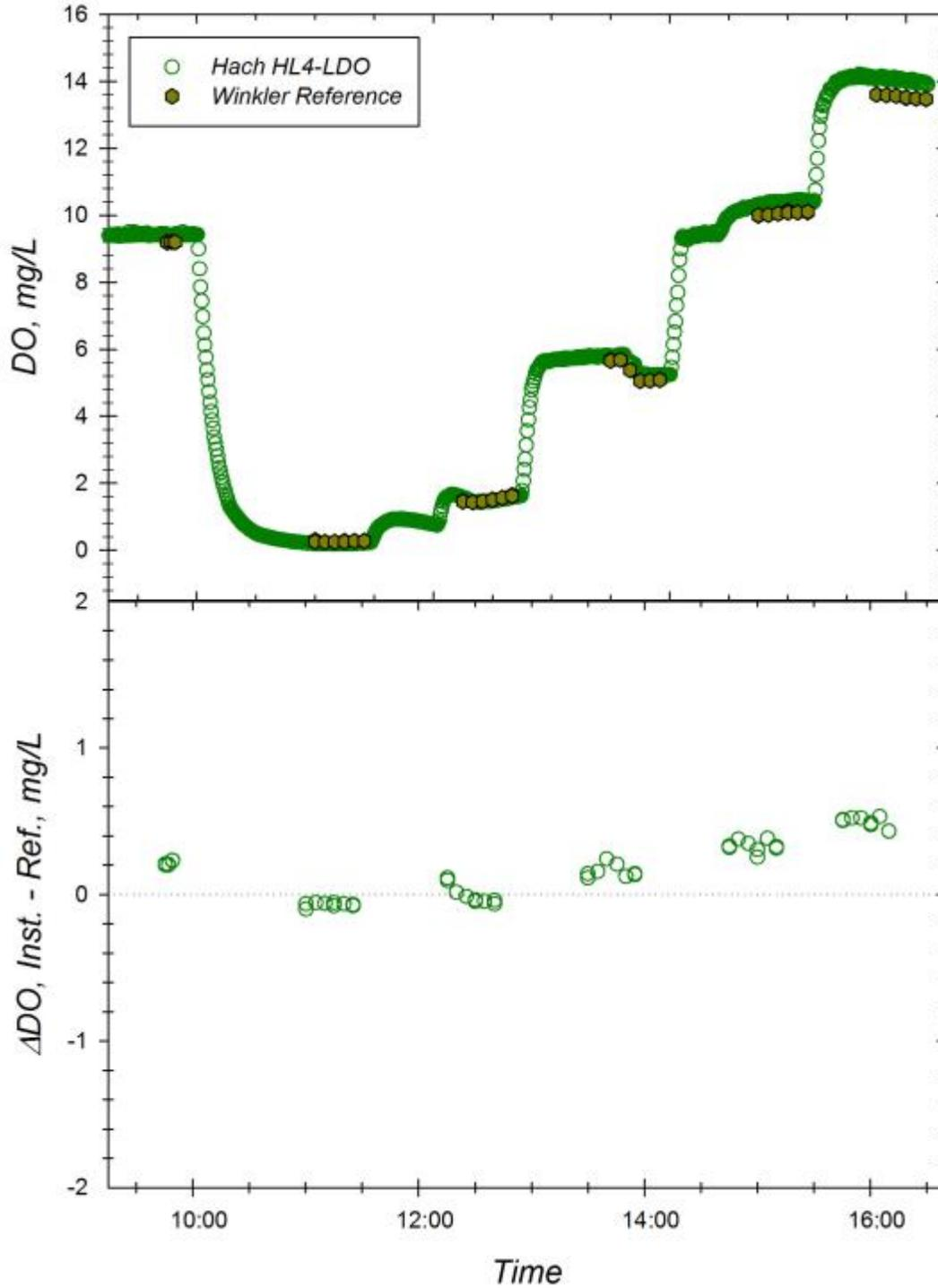
**Figure A.** Response of the Hach HL4 LDO (sn 0431) to changing dissolved oxygen concentrations at 15.4 °C and S=0.00. *Top Panel:* Time series of instrument readings and Winkler reference samples drawn at level of sensor foil in well-mixed test tanks. *Bottom Panel:* Corresponding offset between instrument reading and Winkler DO reference sample during exposure trial. Dotted line represents zero offset from reference.
