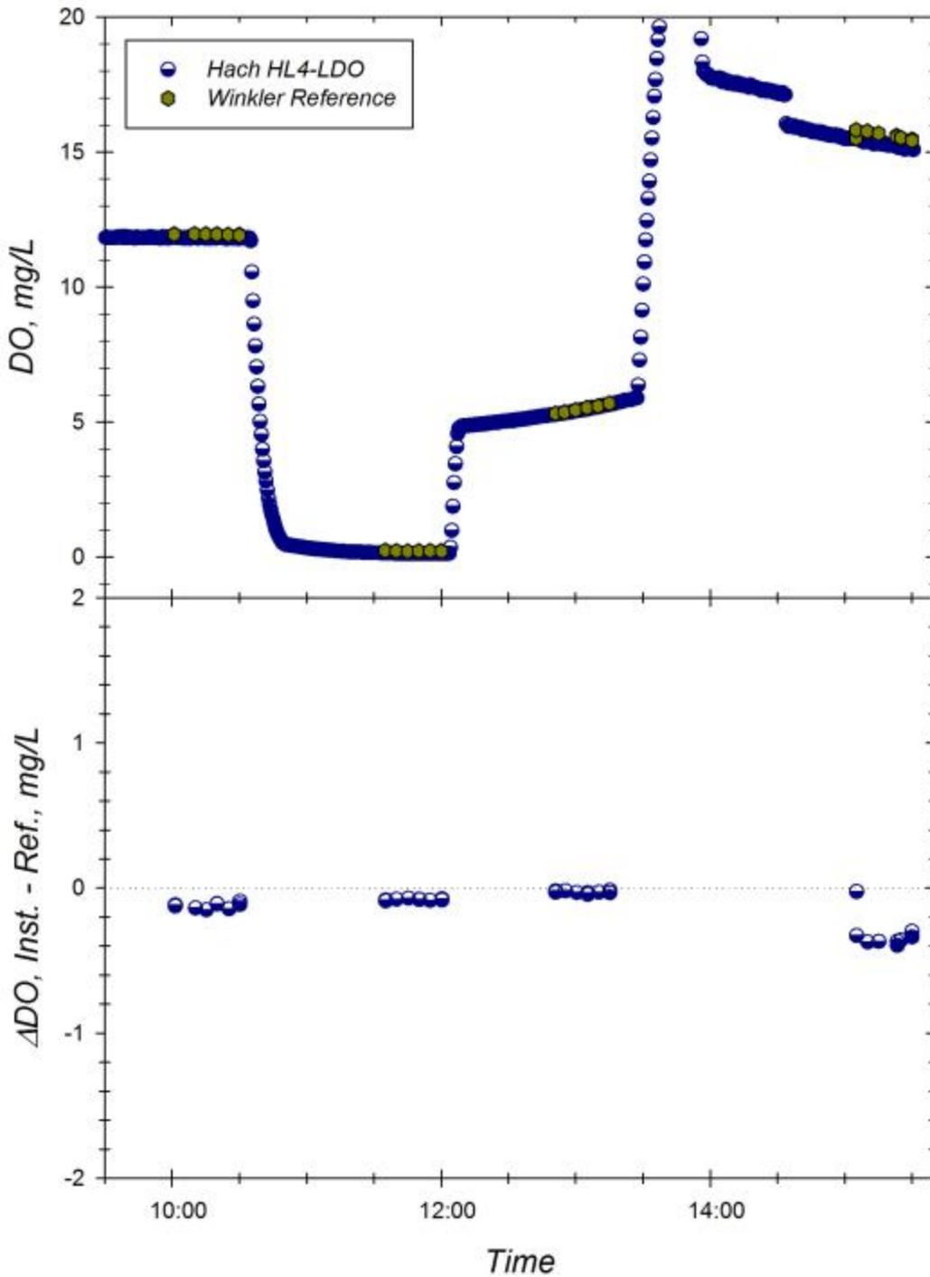
**Figure E.** Response of the Hach HL4 LDO (sn 0431) to changing dissolved oxygen concentrations at 5.3 °C and S=8.98. *Top Panel:* Time series of instrument readings and Winkler reference samples drawn at level of sensor foil in well-mixed test tanks. *Bottom Panel:* Corresponding offset between instrument reading and Winkler DO reference sample during exposure trial. Dotted line represents zero offset from reference.
