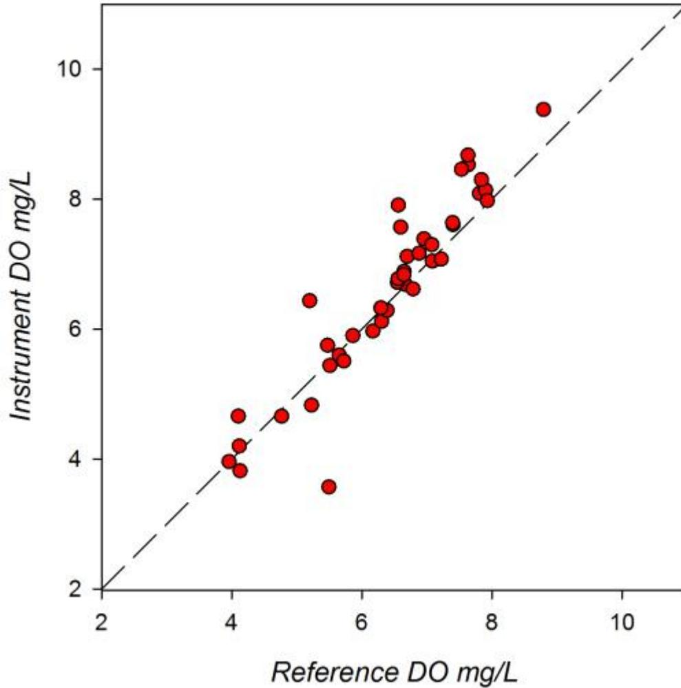
**Figure 9.** HIMB field response plot of HACH DS5X compared to reference DO samples determined by Winkler Titration. The plotted line represents a 1:1 correspondence.
