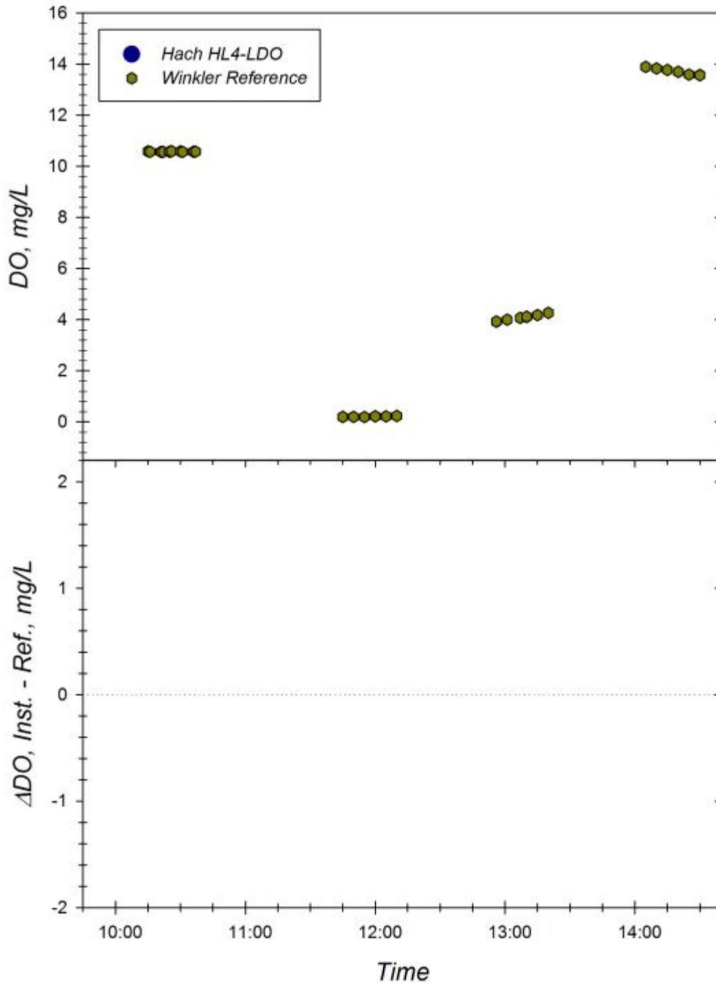
**Figure F.** Response of the Hach HL4 LDO (sn 0431) to changing dissolved oxygen concentrations at 5.2 °C and S=34.77. *Top Panel:* Time series of instrument readings and Winkler reference samples drawn at level of sensor foil in well-mixed test tanks. *Bottom Panel:* Corresponding offset between instrument reading and Winkler DO reference sample during exposure trial. Dotted line represents zero offset from reference. Due to apparent internal power failure, no data was recorded for this trial.
