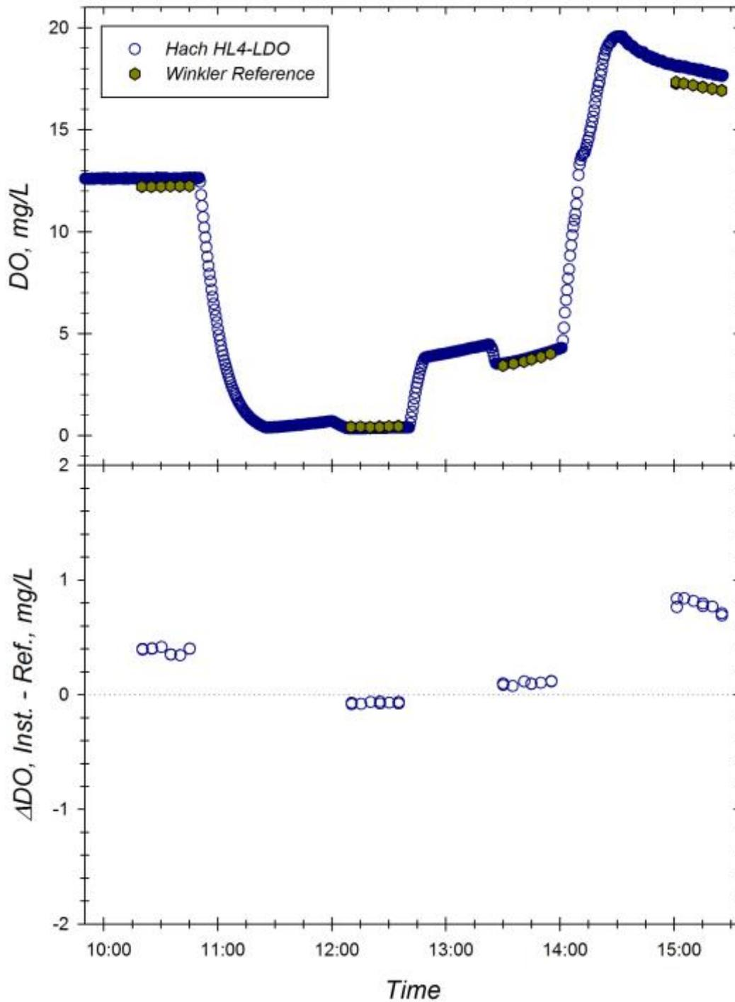
**Figure D.** Response of the Hach HL4 LDO (sn 0431) to changing dissolved oxygen concentrations at 5.4 °C and S=0.00. *Top Panel:* Time series of instrument readings and Winkler reference samples drawn at level of sensor foil in well-mixed test tanks. *Bottom Panel:* Corresponding offset between instrument reading and Winkler DO reference sample during exposure trial. Dotted line represents zero offset from reference.
