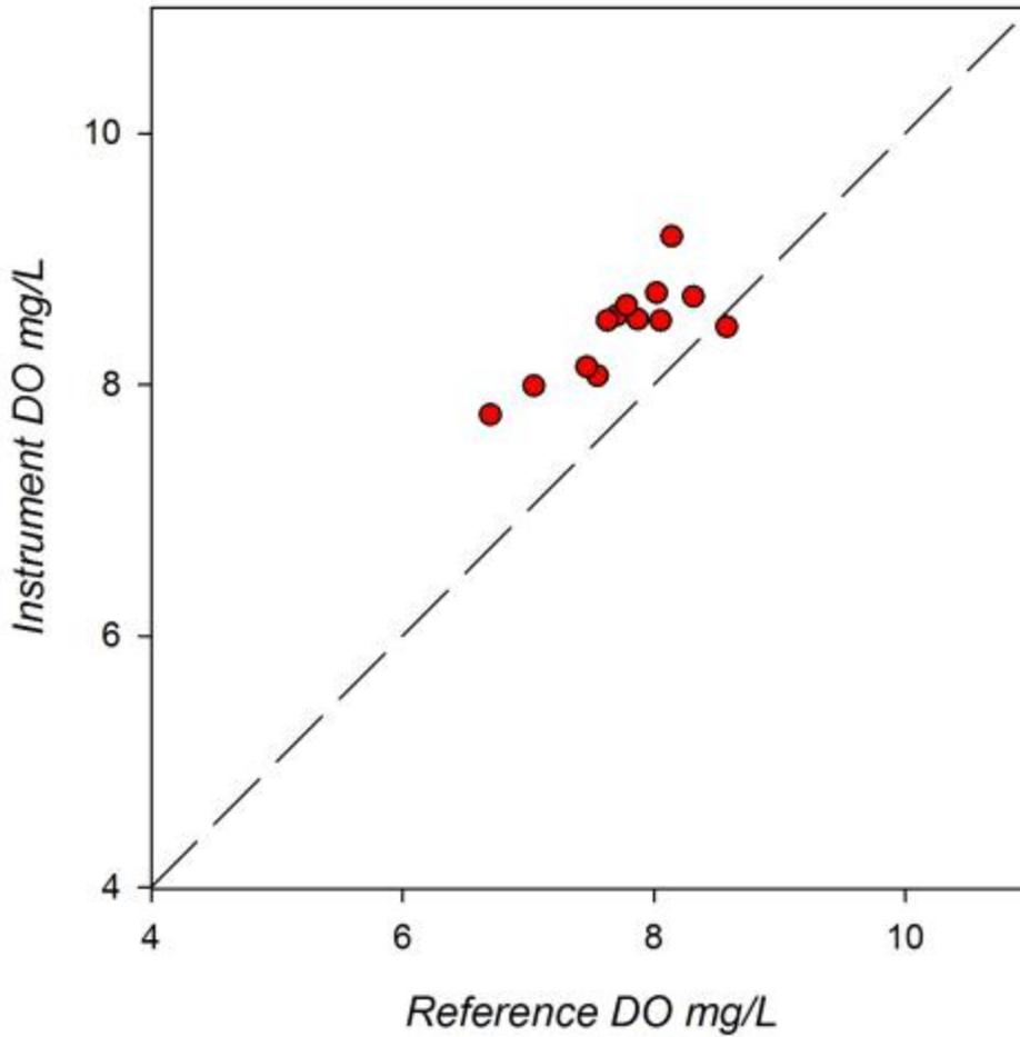
**Figure 4.** CBL field response plot of HACH HL4 compared to reference DO samples determined by Winkler Titration. The plotted line represents a 1:1 correspondence.
