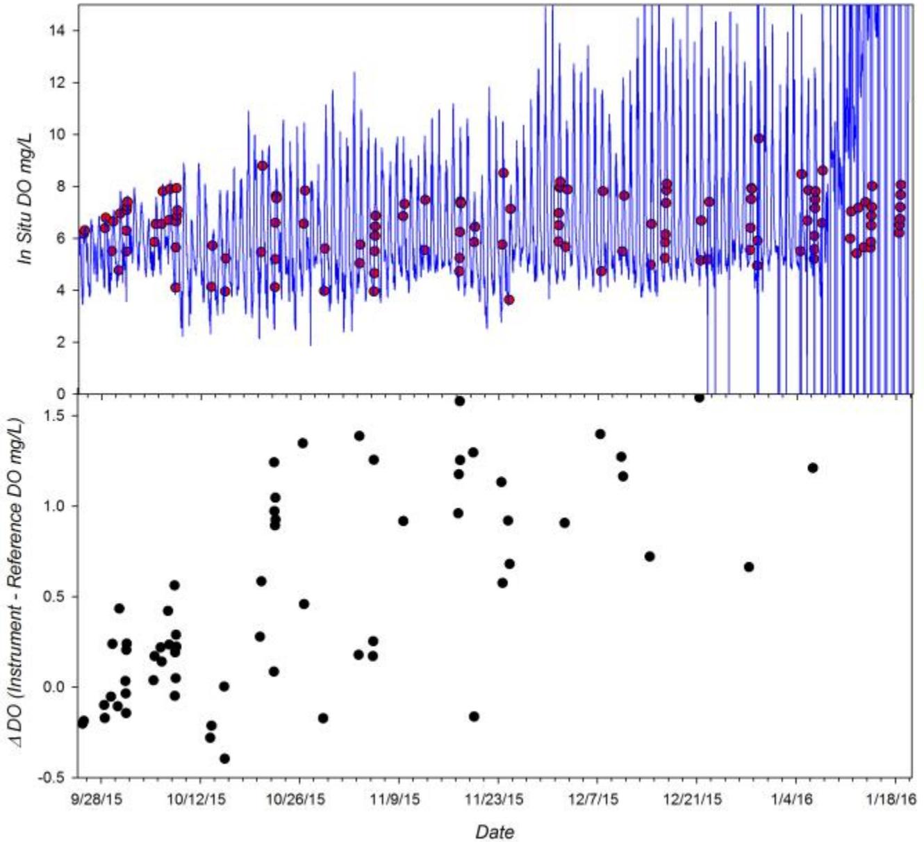
**Figure 8.** *Top panel:* Time series of DO measured by HACH DS5X deployed during the 18 week HIMB field trial. Continuous DO recordings from instrument (blue line) and DO of adjacent grab samples determined by Winkler Titrations (red circles.) *Bottom Panel:* Time series of the difference between the DS5X and reference measurements for each matched pair in the range of  $\pm 2$ mg/L DO (n=53 of a total possible 129 observations).
