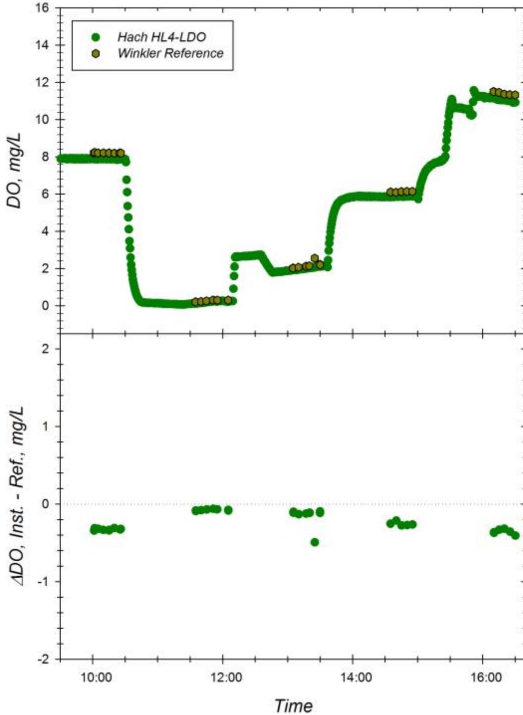
**Figure C.** Response of the Hach HL4 LDO (sn 0431) to changing dissolved oxygen concentrations at 15.4 °C and S=34.20. *Top Panel:* Time series of instrument readings and Winkler reference samples drawn at level of sensor foil in well-mixed test tanks. *Bottom Panel:* Corresponding offset between instrument reading and Winkler DO reference sample during exposure trial. Dotted line represents zero offset from reference.
