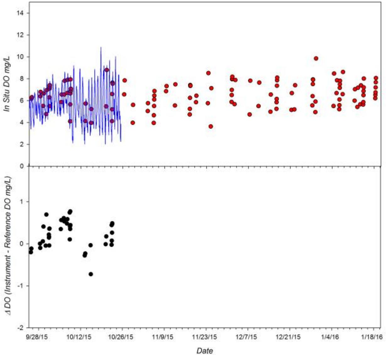
**Figure 6.** *Top panel:* Time series of DO measured by HACH HL4 deployed during the 18 week HIMB field trial. Continuous DO recordings from instrument (blue line) and DO of adjacent grab samples determined by Winkler Titrations (red circles.) *Bottom Panel:* Time series of the difference between the HL4 and reference measurements for each matched pair in (n=39 of a total possible 129 observations).
