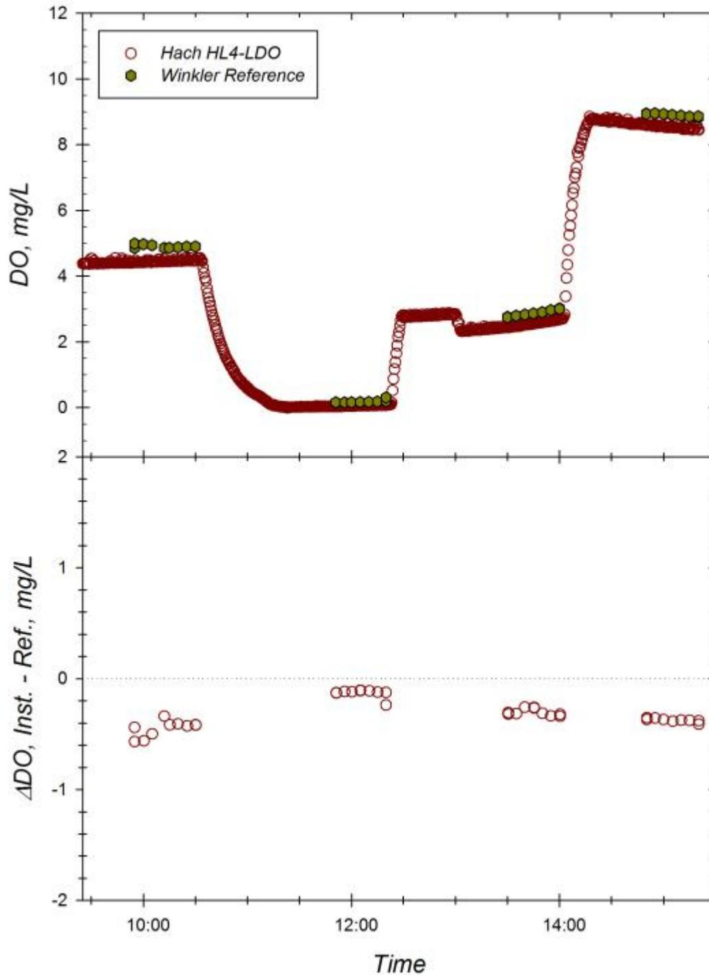
**Figure G.** Response of the Hach HL4 LDO (sn 0431) to changing dissolved oxygen concentrations at 30.2 °C and S=0.00. *Top Panel:* Time series of instrument readings and Winkler reference samples drawn at level of sensor foil in well-mixed test tanks. *Bottom Panel:* Corresponding offset between instrument reading and Winkler DO reference sample during exposure trial. Dotted line represents zero offset from reference.
