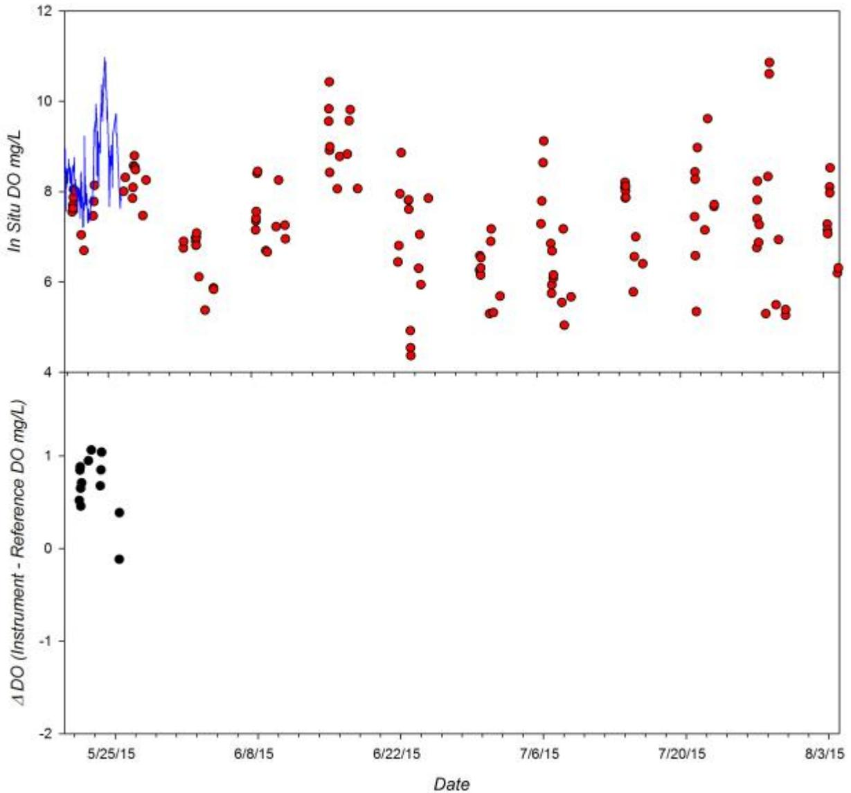
**Figure 3.** Time series of DO measured by the HL4 during the 12 week CBL field trial. *Top Panel:* Continuous DO recordings from instrument (blue line) and DO of adjacent grab samples determined by Winkler titration (red circles). *Bottom Panel:* Difference in measured DO relative to reference samples (Instrument – Reference) observed during deployment.
