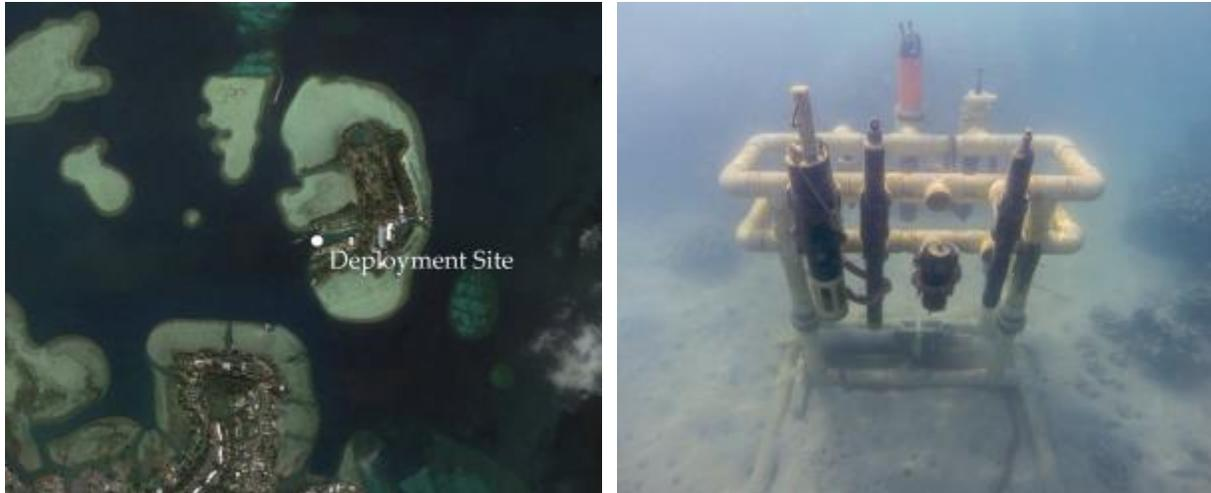
**Photo 4.** Aerial view of HIMB deployment site (left) and instrument rack in-situ (right).
