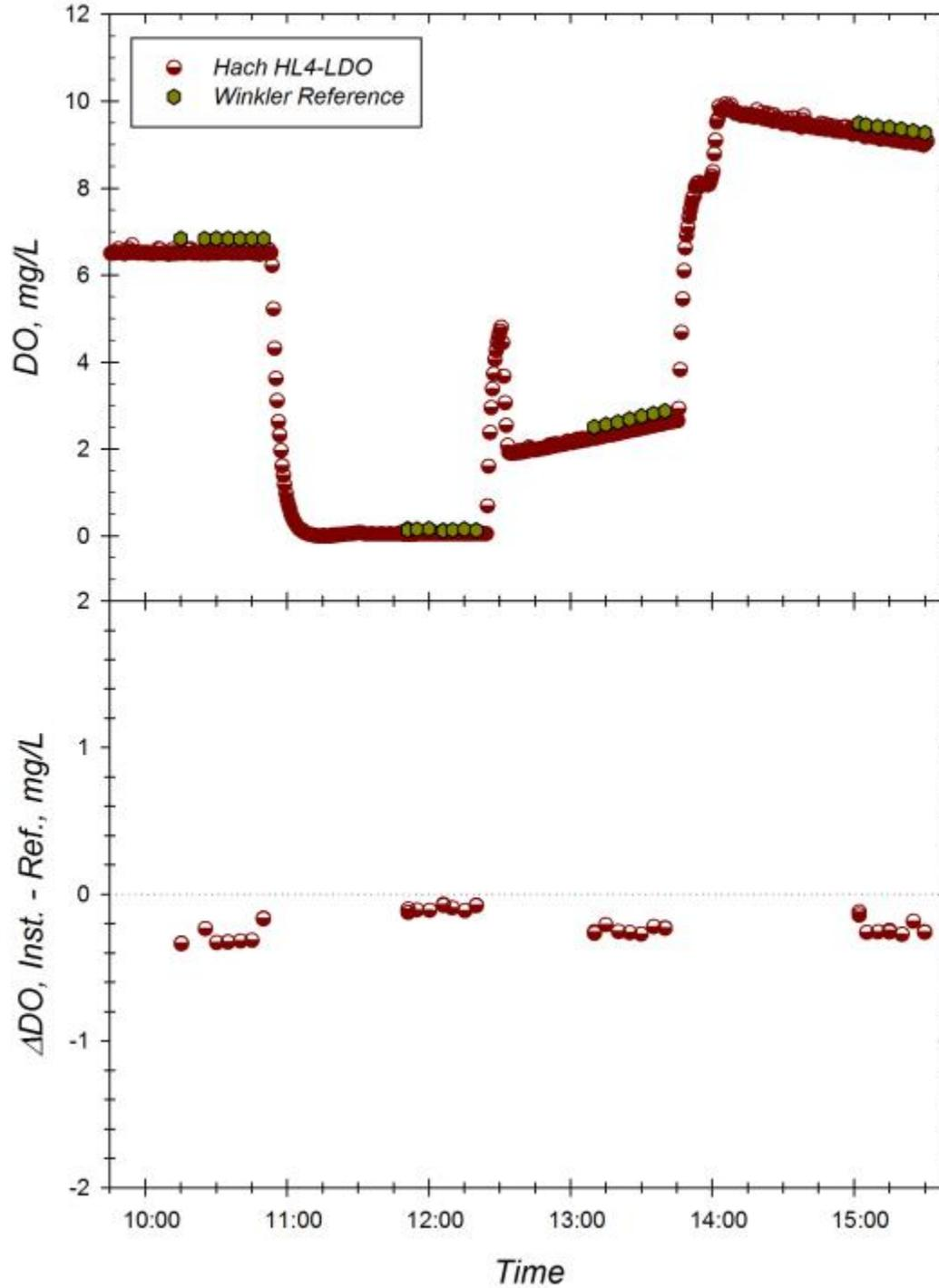
**Figure H.** Response of the Hach HL4 LDO (sn 0431) to changing dissolved oxygen concentrations at 30.5 °C and S=9.28. *Top Panel:* Time series of instrument readings and Winkler reference samples drawn at level of sensor foil in well-mixed test tanks. *Bottom Panel:* Corresponding offset between instrument reading and Winkler DO reference sample during exposure trial. Dotted line represents zero offset from reference.
