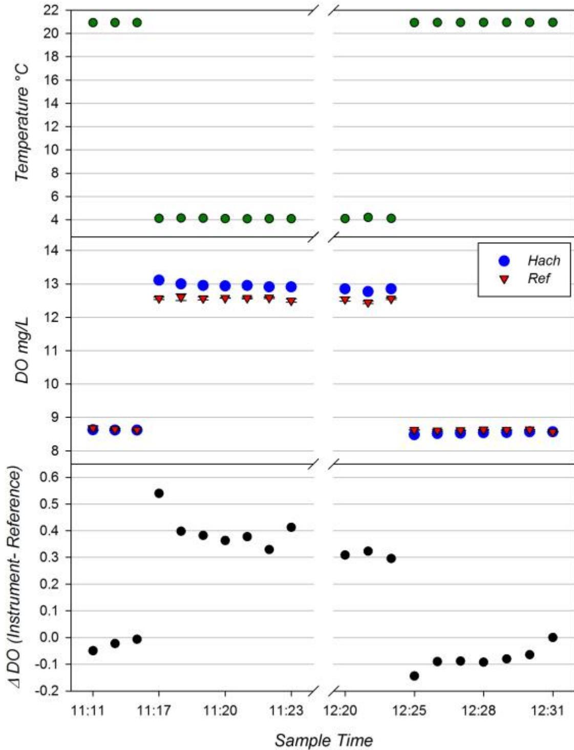
**Figure 16.** Results of the HACH HL4 for the Lake Michigan trials. *Top panel:* HL4 temperature data at sample snap. *Middle panel:* DO recordings from instrument (blue dot) and DO of adjacent sample snaps determined by Winkler Titrations (red triangles.) *Bottom panel:* Time series of the difference between the HL4 and reference measurements for each matched pair. Cast 1 and 2 are plotted on the same graph and separated by the axis break.
