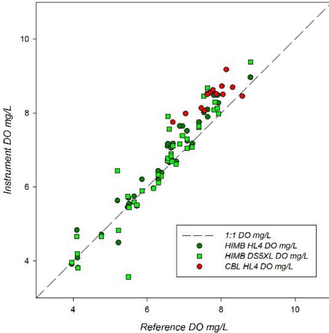
**Figure 10.** Global response plot for the HL4 (circles) and DS5XL (squares) instruments observed during the three ACT field trials. Black dotted line represents a 1:1 correspondence.
