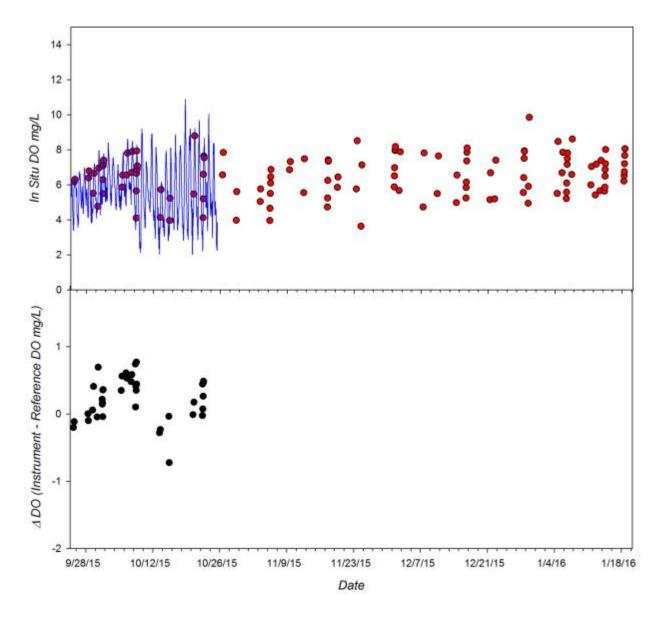
**Figure 6**. *Top panel:* Time series of DO measured by HACH HL4 deployed during the 18 week HIMB field trial. Continuous DO recordings from instrument (blue line) and DO of adjacent grab samples determined by Winkler Titrations (red circles.) *Bottom Panel: T*ime series of the difference between the HL4 and reference measurements for each matched pair in (n=39 of a total possible 129 observations).
