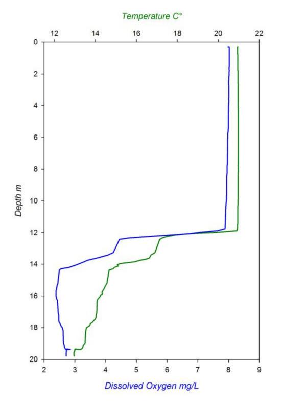
**Figure 12**. Temperature and DO concentration profiles for Muskegon Lake. Values were obtained from the average of multiple instruments sampling at 1s frequency. The hypolimnion was approximately 8m thick and contained depressed DO levels of less than 3 mg/L.
