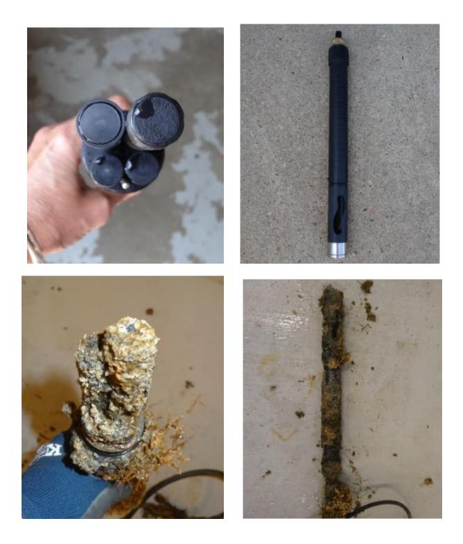
**Photo 3**. The Hach HL4 prior to and following the 18 week CBL field trial.
