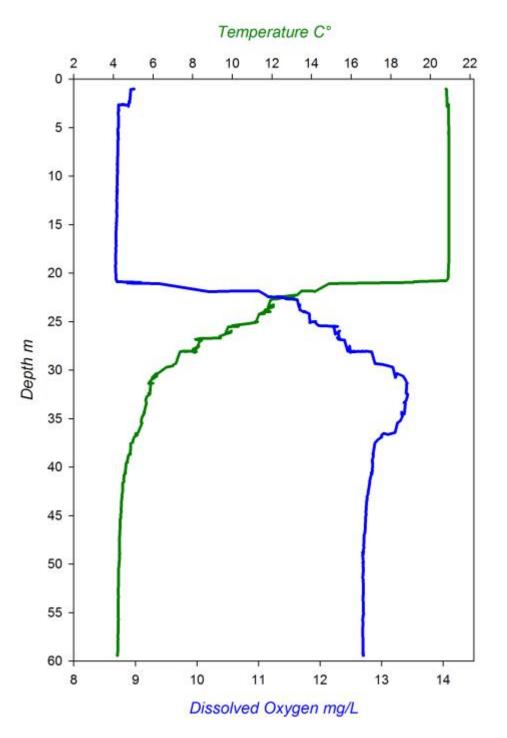
**Figure 14.** Temperature and DO concentration profiles for Lake Michigan. Values were obtained from the average of multiple instruments sampling at 1s frequency. The hypolimnion was approximately 40m thick (the rosette was stopped at 60m about 30m below the thermocline) and contained elevated DO levels of more than 12.6 mg/L.
