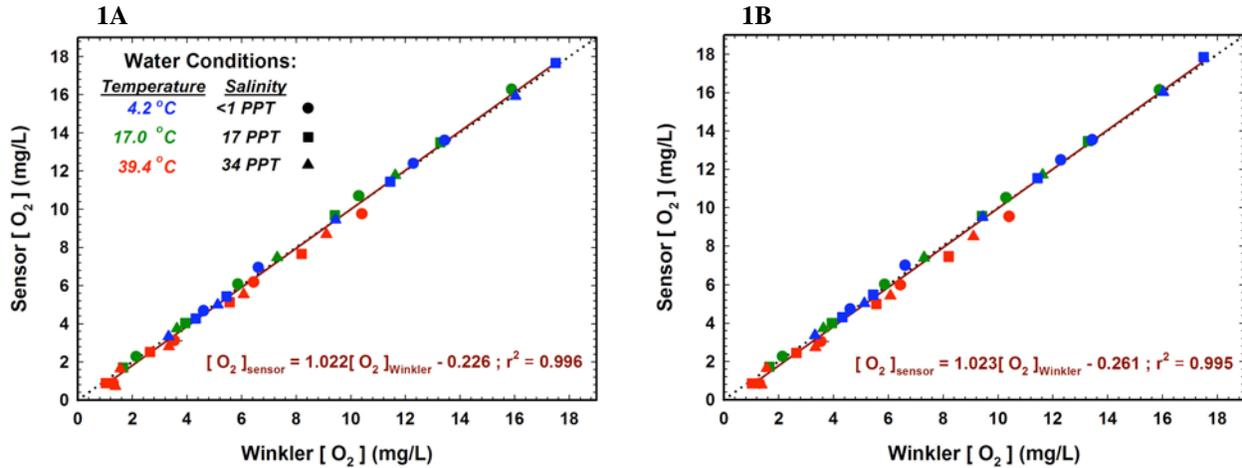
**Laboratory Precision** – The precision test was conducted in a well-mixed freshwater bath (0.0 ppt) held at 17.2 °C that was continuously aerated (i.e., air saturated). The mean, standard deviation (STD), and coefficient of variance (% CV = STD/Mean x 100) for DO values (mg/L) generated from 30 replicate Winkler titrations of water samples collected from the bath and 30 replicate instrument values taken simultaneously, are listed below in Table 3.
