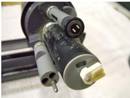
Sensor without the biofouling prevention system after four-week laboratory deployment.
