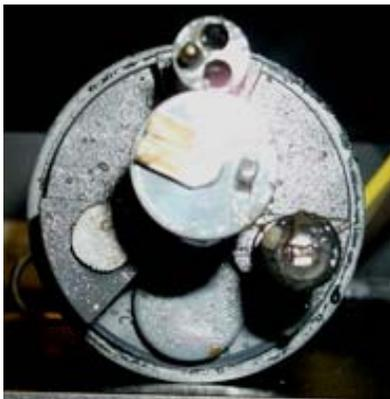
Sensor without the biofouling prevention system after four-week field deployment.
