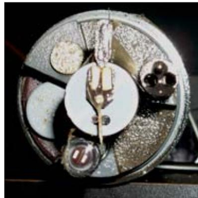
Sensor with the biofouling prevention system after four-week field deployment.
