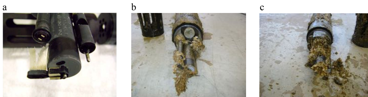
Figure 11. Biofouling of dissolved oxygen sensors after 26-days deployment in Chesapeake Bay in September 2012 (a) predeployment, (b) with biofouling prevention, (c) without biofouling prevention system.
