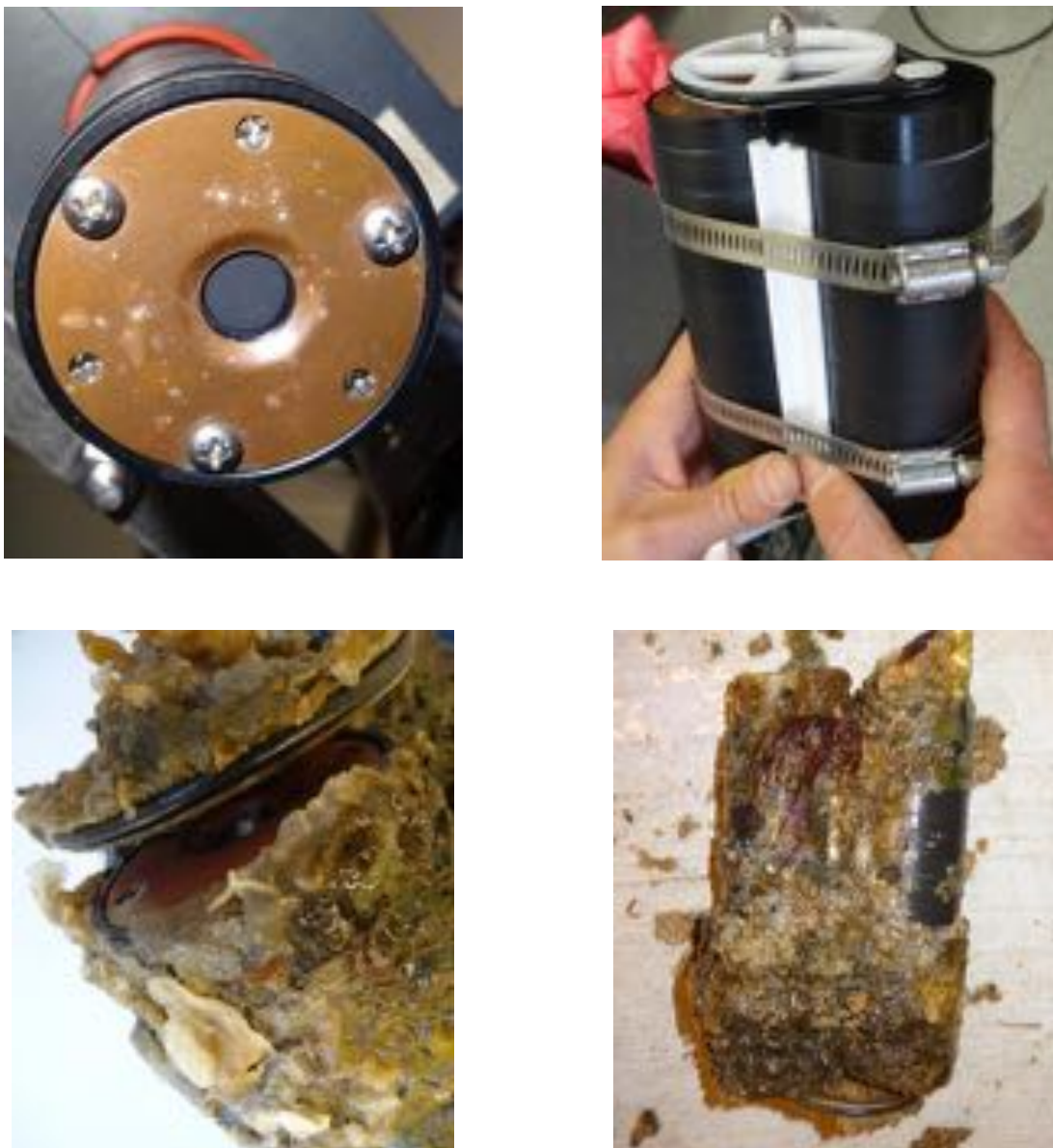
Figure 14. An example of a test instrument prior to deployment and the test instrument after the Chesapeake Bay field deployment to indicate potential impact of biofouling.
