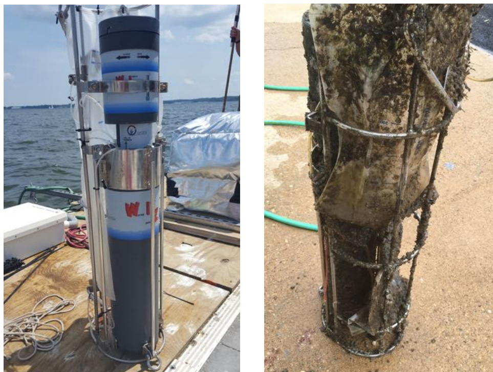
Figure 10. Pre- and post-deployment at CBL showing extent of bio-fouling.
