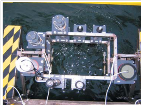
Dissolved oxygen sensor mooring frame prior to deployment off the Darling Marine Center Pier
