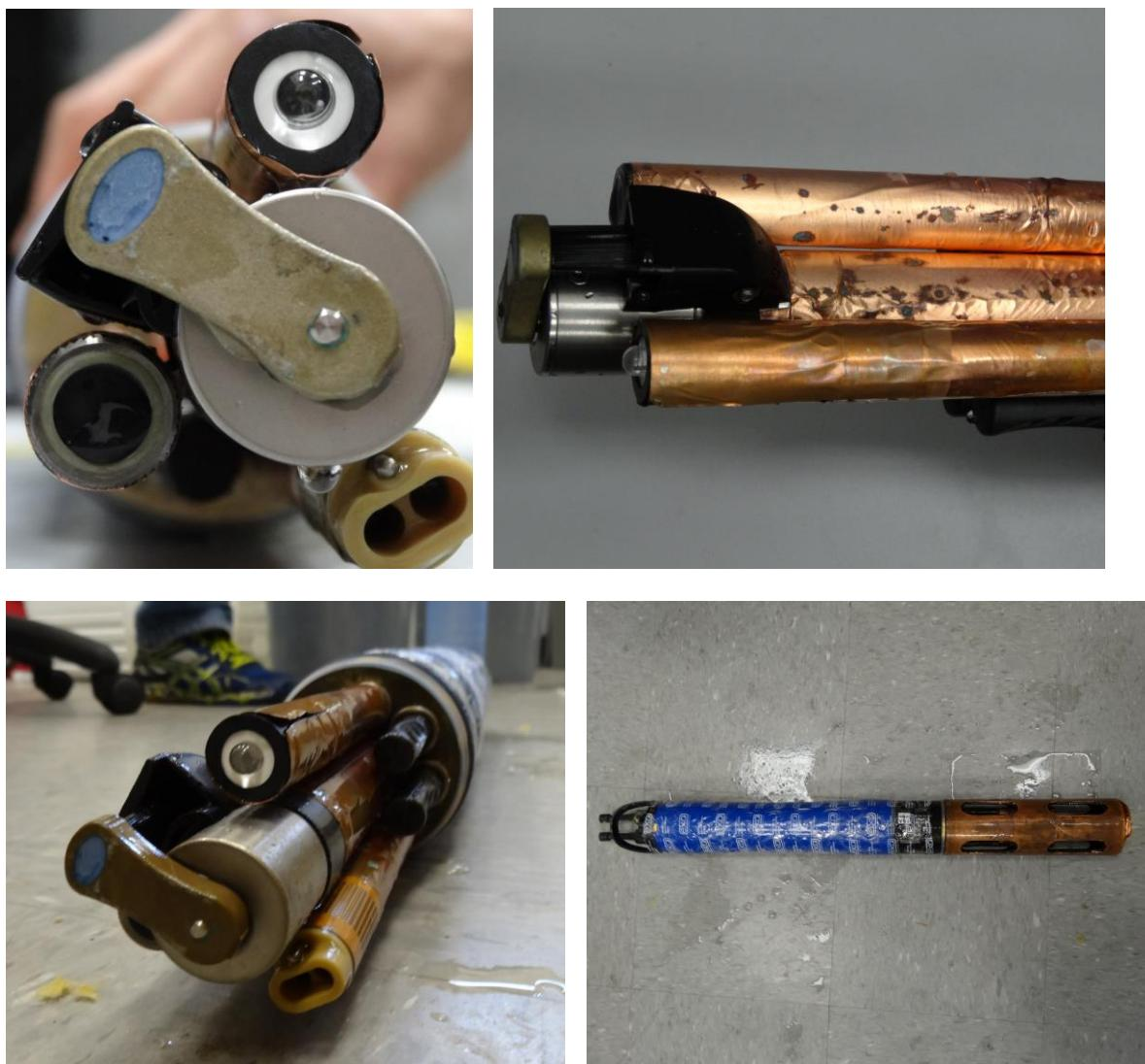
**Photo 7.** The Xylem EXO prior to and following the 1 month deployment for the CBL field test.
