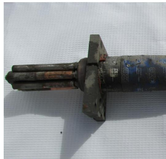
**Photo 3.** The Xylem EXO pH prior to and following the 1 month deployment for the MLML field test.
