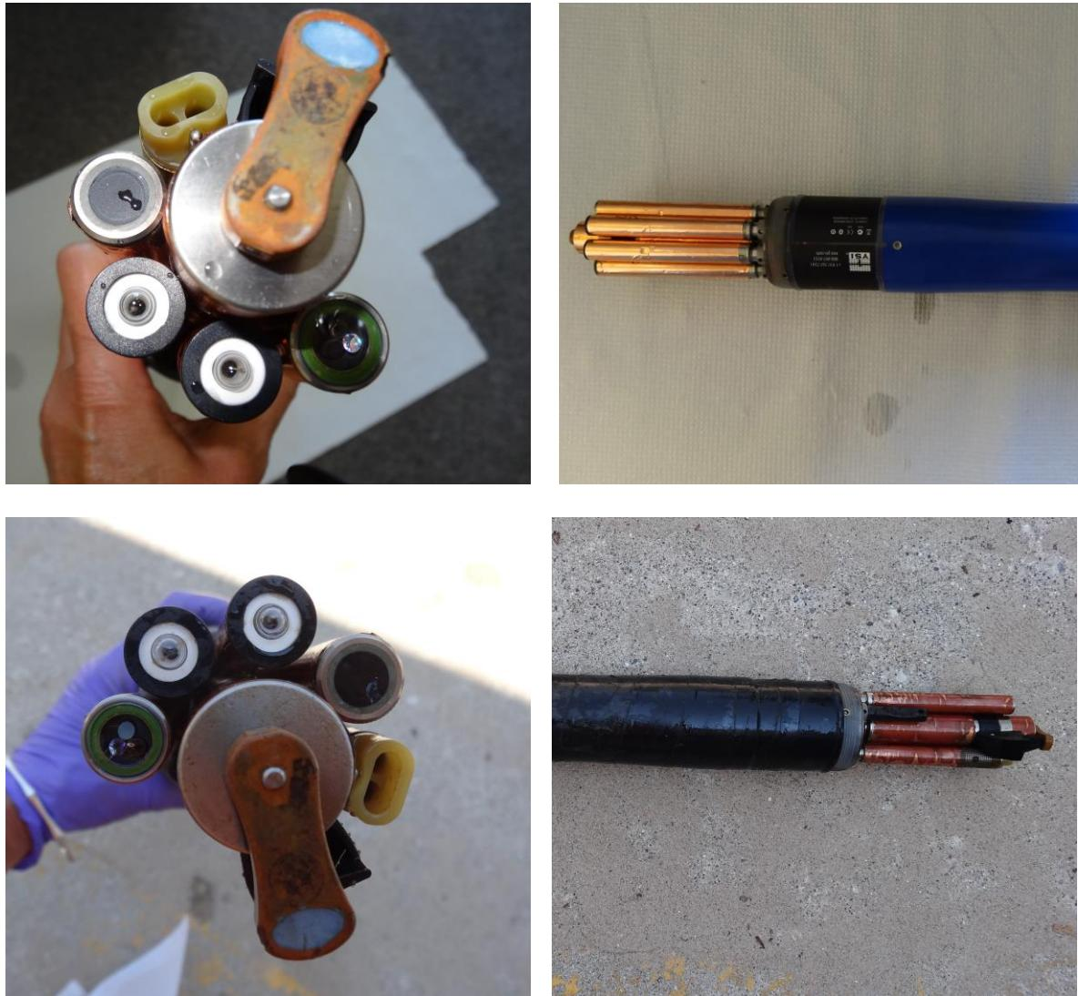
**Photo 9.** The Xylem EXO pH sensor prior to and following the 1 month deployment for the Great Lakes field test.
