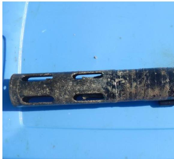
**Photo 5.** The Xylem EXO pH sensor prior to and following the 3 month deployment for the HIMB field test.
