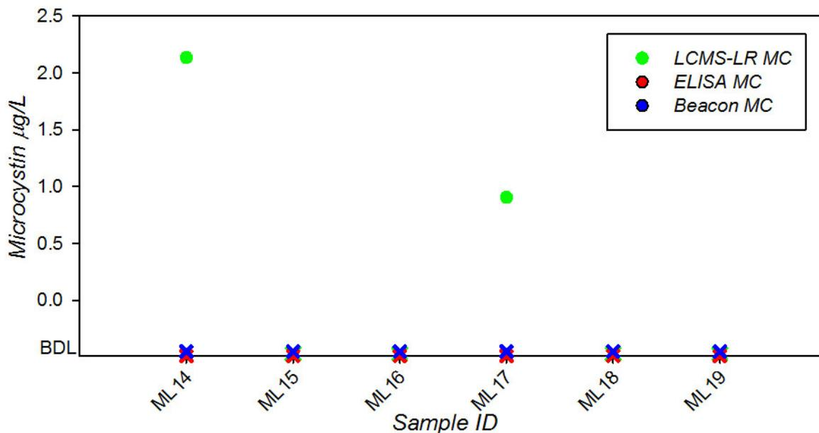
Figure 18. MLML Pinto and El Estero Lakes (ML 15) comparison of instrument (blue), reference ELISA (red) and LCMS-LR (green) whole microcystin data. Error bars denote one standard deviation for Beacon (n=2) and ELISA (n=2), LCMS-LR has no error bars as it was a single value. Beacon BDL < 0.5 µg/L. Samples ML18 and ML 19 are independently collected field duplicates.
