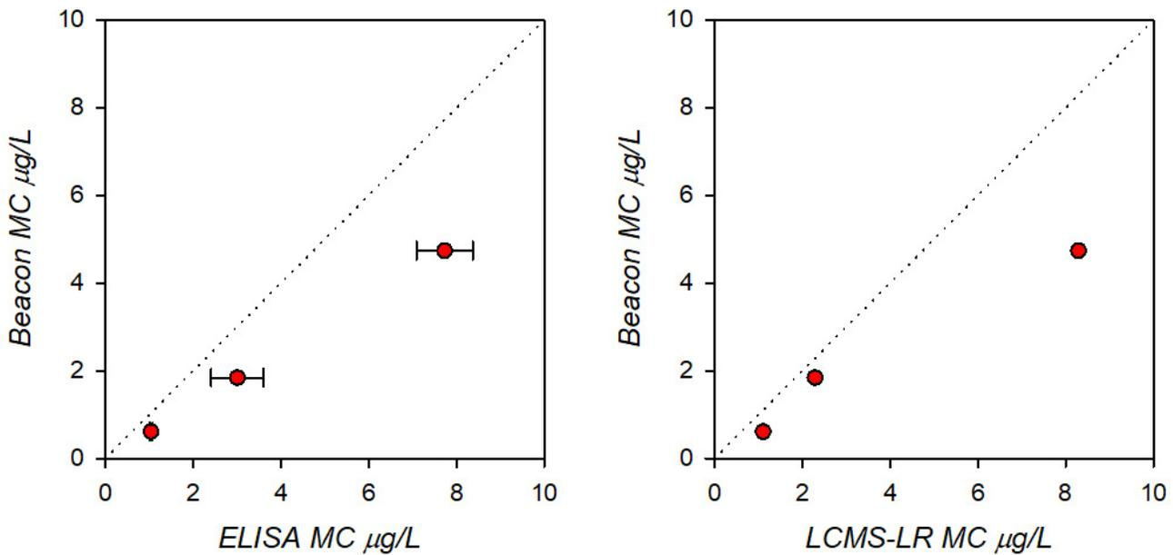
Figure 3. A cross plot of the Beacon measurements compared to reference ELISA (left) and LCMS-LR (right) for the common lysate laboratory trial. Error bars are one standard deviation of analytical replicates (n=2) for ELISA data, LCMS-LR and Beacon data has no error bars as there are no replicates.
