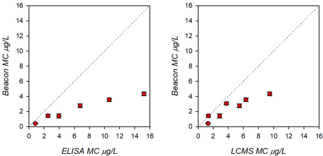
Figure 9. A cross plot of Beacon measurements compared to reference ELISA and LCMS-LR microcystin measurements for the laboratory range trial. Error bars represent one standard deviation (n = 2) for Beacon and ELISA, LCMS-LR have no error bars as there was a single value.
