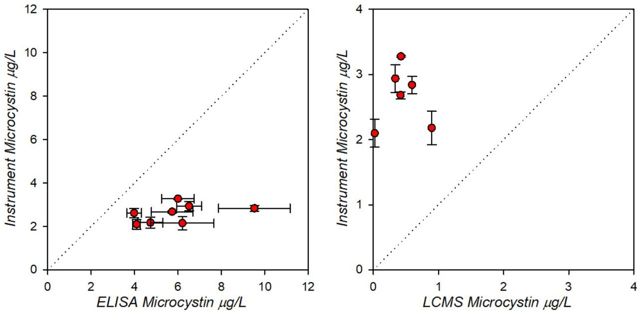
Figure 15. Sandusky Bay field response plot of Beacon compared to the ELISA (left) and LCMS-LR (right) whole water reference data. Error bars represent one standard deviation for Beacon and ELISA (n=2), LCMS-LR has no error bars as there was only one value. Data below detection is not included.
