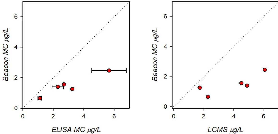
Figure 6. Cross plots for the Beacon measured microcystin compared to reference ELISA (left) and LCMS-LR (right) for the laboratory mixed species trial. Error bars are one standard deviation (n=2), LCMS-LR and Beacon data has no error bars as there was a single value. Beacon BDL data (<0.3 µg/L) is not included.
