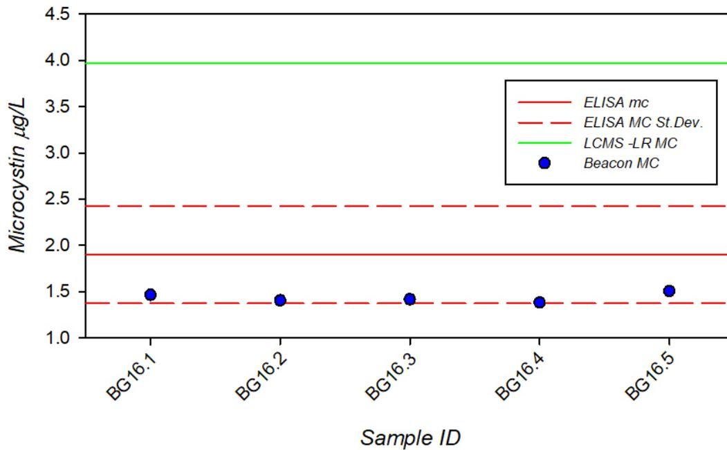
Figure 10. Results of the precision trial laboratory test using repeated measurement of a diluted certified MC standard to a targeted concentration of 1.5 µg/L, the ELISA estimated the concentration at 1.9 ±0.53.
