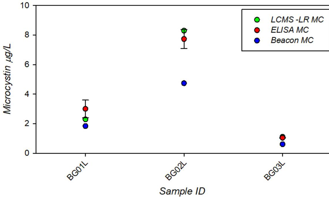
Figure 2. Comparison of microcystin estimates of samples analyzed by Beacon (blue), ELISA (red), and LCMS-LR (green) from the BGSU lab common lysate trial. Error bars are one standard deviation of the analytical replicates (n=2) for ELISA. LCMS-LR and Beacon have no error bars as there are no replicates.
