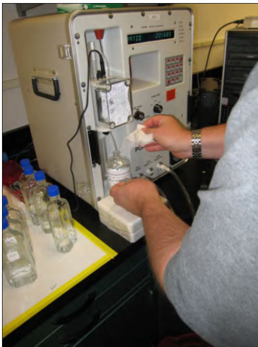
Figure 1. Analytical instrumentation (Portasal 8410A) used for laboratory analysis of salinity reference samples and one of the test baths and instrument racks used for the laboratory tests.
