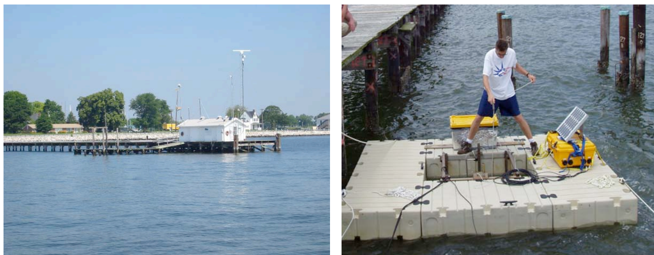
Figure 1. Site Photos from the field deployment in Chesapeake Bay, MD. Left - fixed pier at mouth of Patuxent River on the campus of the Chesapeake Biological Laboratory. Right - ACT staff collecting a reference sample next to the instrument sampling inlet through a well on the sampling platform.
