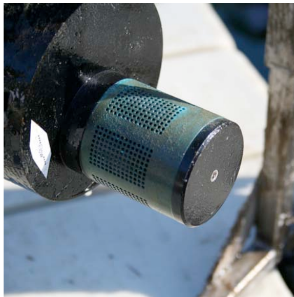
ISUS sampling inlet after test deployment
