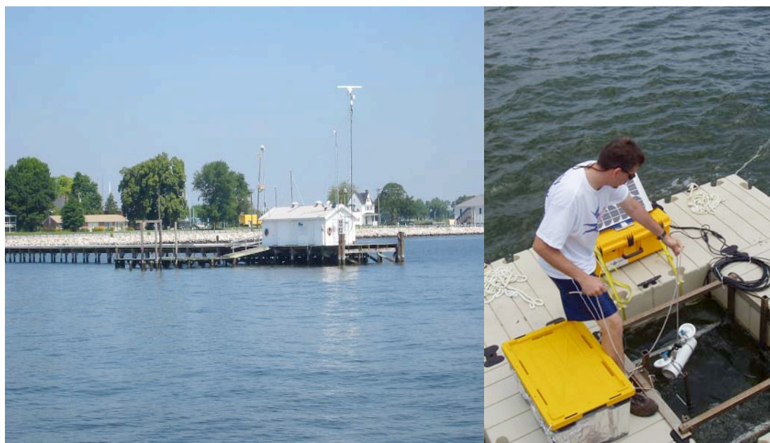
Figure 10. Site Photos from the field deployment in Chesapeake Bay, MD. Left - fixed pier at mouth of Patuxent River on the campus of the Chesapeake Biological Laboratory. Right - ACT staff collecting a reference sample next to the instrument sampling inlet through a well on the sampling platform.
