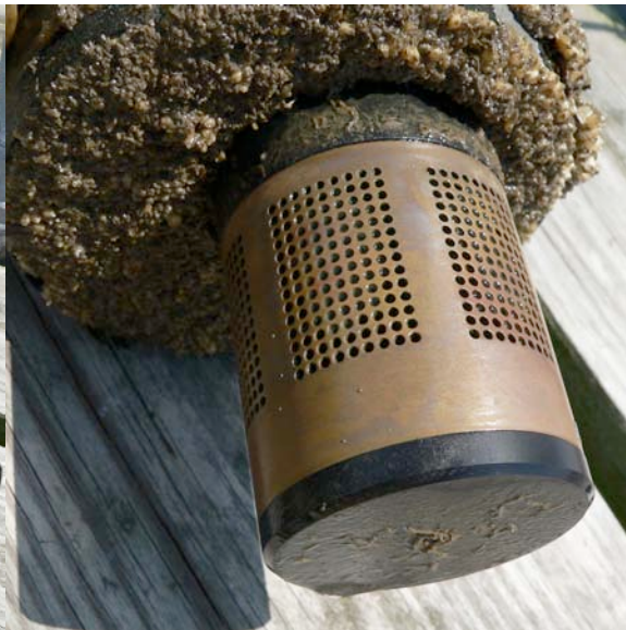
ISUS V3 sample inlet after moored deployment
