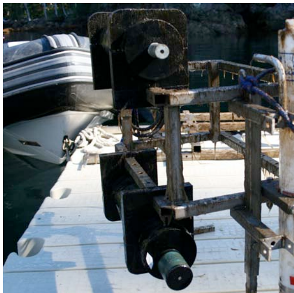
Satlantic ISUS V3 after test deployment
