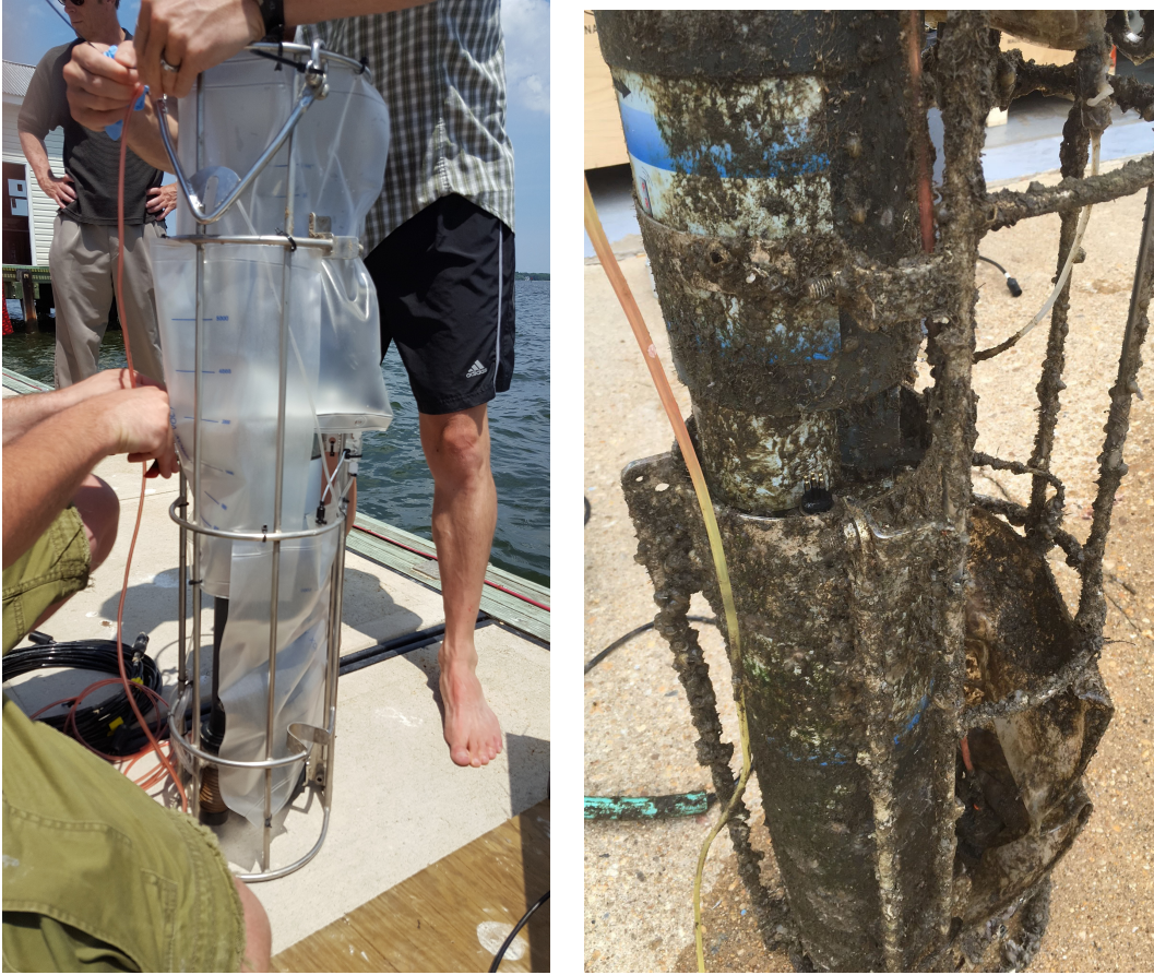
Figure 17. Photographs of the Systea-PO4 instrument prior to and following the CBL field trial.
