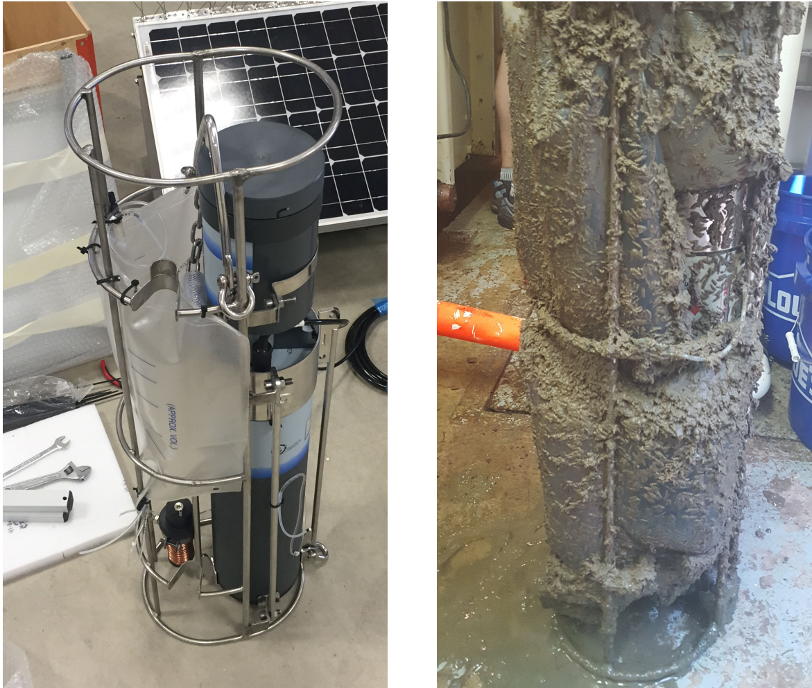
Figure 12. Photographs of the Systea-PO4 prior to and following a 32 day field test in the Maumee River.
