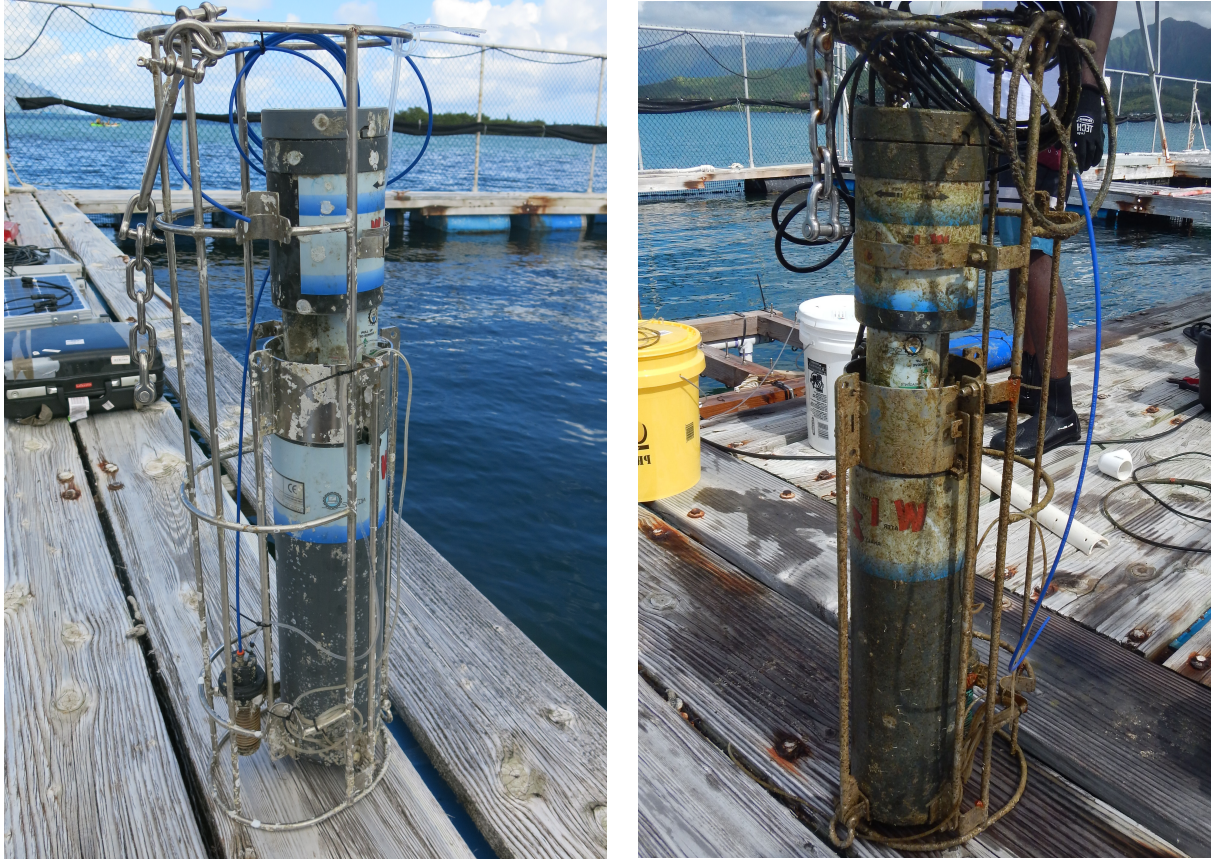
Figure 22. Photographs of the Systea-PO4 prior to and following the one month HIMB field trial.
