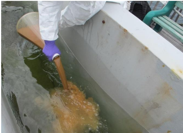
Photo 5. Addition of oil and Corexit 9500
