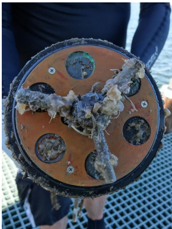
Figure 45. Instrument photographs prior to deployment ( top ) and upon retrieval ( bottom ).
