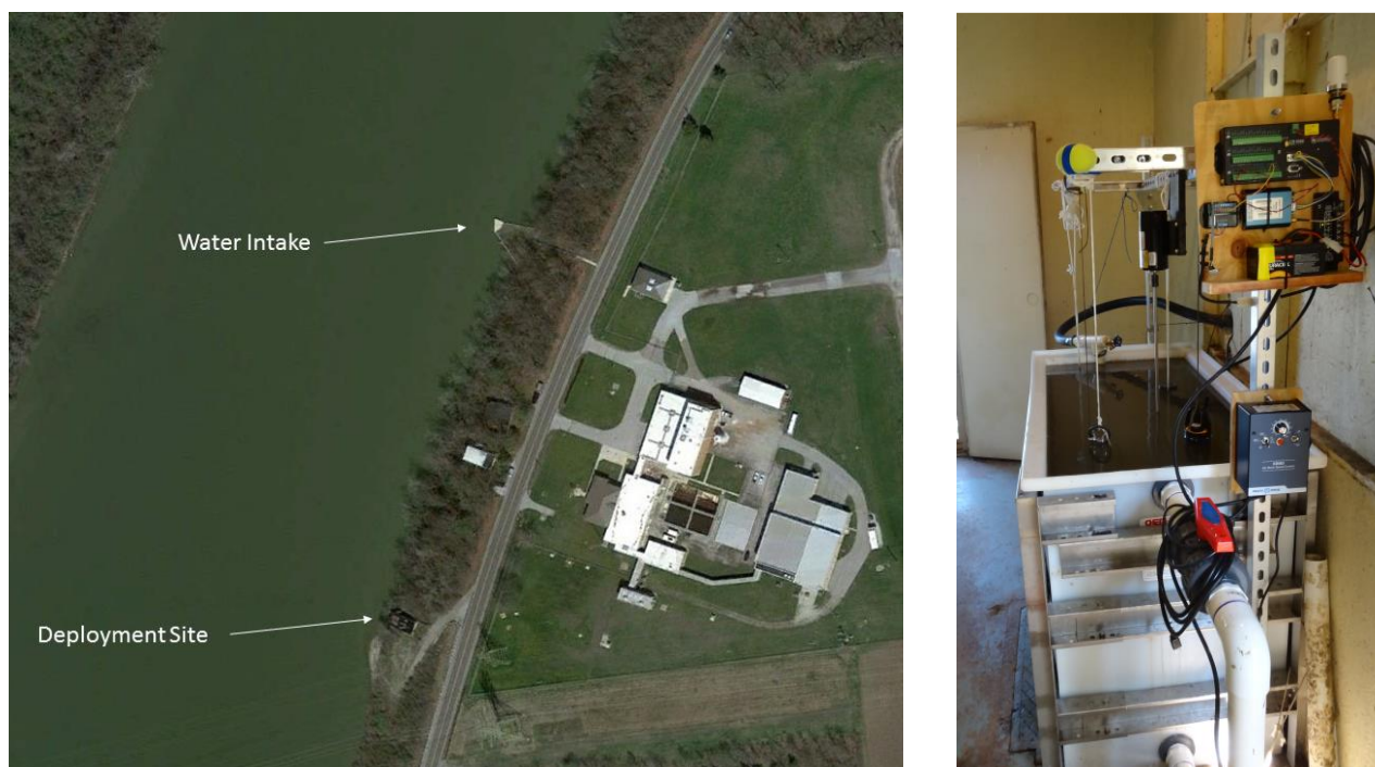
Figure 34. Aerial view of the Maumee River and Bowling Green Water Treatment plant (left) and the flow-through deployment tank servicing the supply of river water to the test instruments (right).
