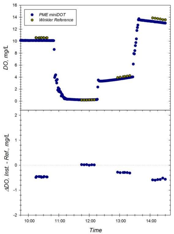
**Figure F.** Response of the PME miniDOT (sn 7392-340698) to changing dissolved oxygen concentrations at 5.2°C and S=34.77. *Top Panel*: Time series of instrument readings and Winkler reference samples drawn at level of sensor foil in well-mixed test tanks. *Bottom Panel*: Corresponding offset between instrument reading and Winkler DO reference sample during exposure trial. Dotted line represents zero offset from reference.
