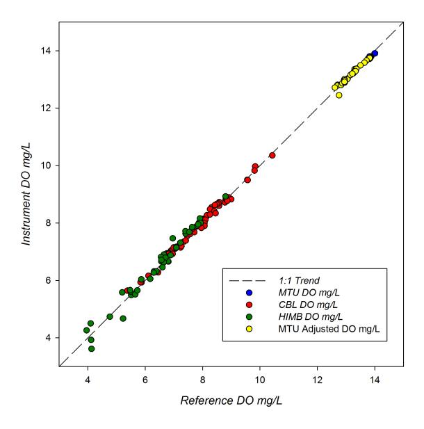
**Figure 10.** Global response plot for the PME miniDOT instruments observed during the three ACT field trials. Black dotted line represents a 1:1 correspondence.
