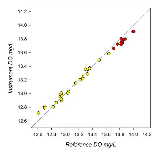
**Figure 3**. MTU GLRI field response plot for the first month of deployment of PME miniDOT instrument compared to reference DO samples. The plotted line represents a 1:1 correspondence. (Yellow circles denote adjusted reference values).
