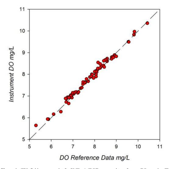
**Figure 6.** CBL field response plot for PME miniDOT compared to reference DO samples. The plotted line represents a 1:1 correspondence.
