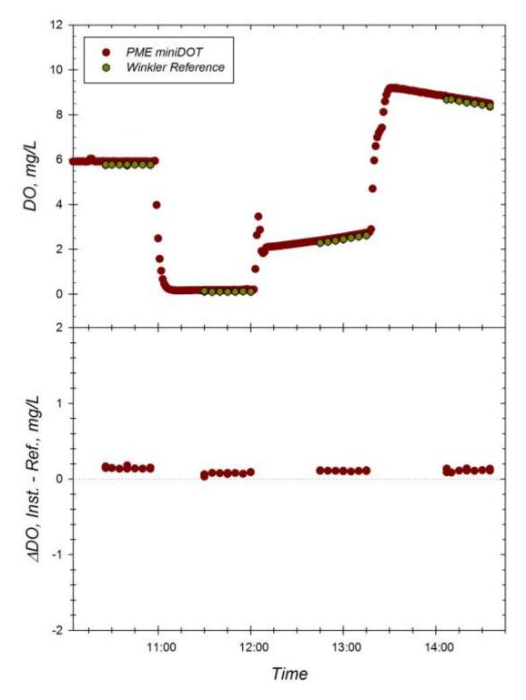
**Figure I.** Response of the PME miniDot (sn 7392-340698) to changing dissolved oxygen concentrations at 30.6°C and S=34.43. *Top Panel*: Time series of instrument readings and Winkler reference samples drawn at level of sensor foil in well-mixed test tanks. *Bottom Panel*: Corresponding offset between instrument reading and Winkler DO reference sample during exposure trial. Dotted line represents zero offset from reference.
