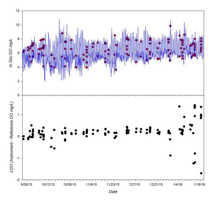
**Figure 8**. *Top panel*: Time series of DO measured by PME miniDOT deployed during the 18 week HIMB field trial. Continuous DO recordings from instrument (blue line) and DO of adjacent grab samples determined by Winkler Titrations (red circles.) *Bottom Panel*: Time series of the difference between the PME and reference measurements (Instrument DO mg/L – Reference DO mg/L) for each matched pair in the range of  $\pm 2$ mg/L DO (n=128 of a total possible 129 observations).
