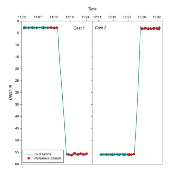
**Figure 13**. Time series of the rosette profiling and Niskin bottle sampling for the two profiling trials in Lake Michigan.
