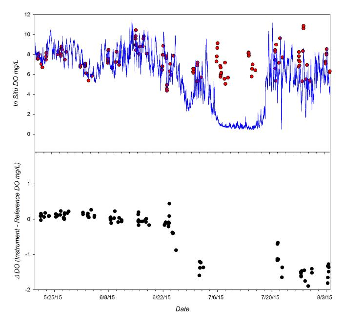
**Figure 5.** Time series of DO measured by the PME miniDOT during the 12 week CBL field trial. *Top Panel*: Continuous DO recordings from instrument (blue line) and DO of adjacent grab samples determined by Winkler titration (red circles). *Bottom Panel*: Difference in measured DO relative to reference samples (Instrument DO mg/L – Reference DO mg/L) observed during deployment.
