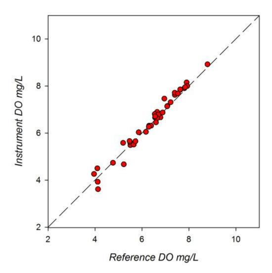
**Figure 9.** HIMB field response plot of PME miniDOT compared to reference DO samples determined by Winkler Titration. The plotted line represents a1:1 correspondence.
