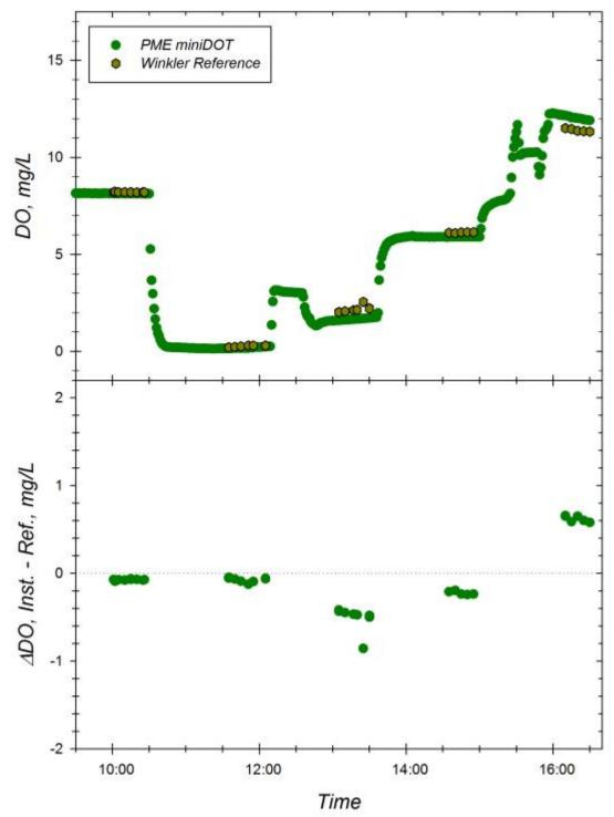
**Figure C.** Response of the PME miniDOT (sn 7392-340698) to changing dissolved oxygen concentrations at 15.4°C and S=34.20. *Top Panel*: Time series of instrument readings and Winkler reference samples drawn at level of sensor foil in well-mixed test tanks. *Bottom Panel*: Corresponding offset between instrument reading and Winkler DO reference sample during exposure trial. Dotted line represents zero offset from reference.
