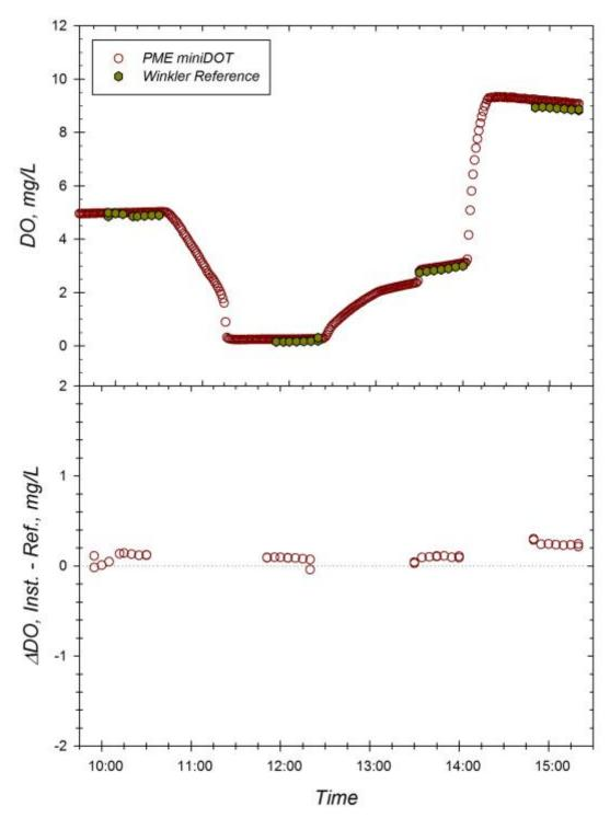
**Figure G.** Response of the PME miniDOT (sn 7392-340698) to changing dissolved oxygen concentrations at 30.2°C and S=0.00. *Top Panel*: Time series of instrument readings and Winkler reference samples drawn at level of sensor foil in well-mixed test tanks. *Bottom Panel*: Corresponding offset between instrument reading and Winkler DO reference sample during exposure trial. Dotted line represents zero offset from reference.
