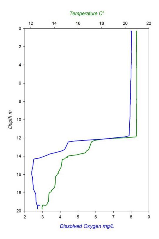
**Figure 12**. Temperature and DO concentration profiles for Muskegon Lake. Values were obtained from the average of multiple instruments sampling at 1s frequency. The hypolimnion was approximately 8m thick and contained depressed DO levels of less than 3 mg/L.
