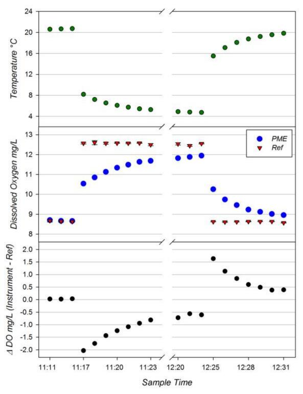
Figure 16. Results of the PME miniDOT for the Lake Michigan trials. *Top panel:* PME temperature data at sample snap. *Middle panel:* DO recordings from instrument (blue dot) and DO of adjacent sample snaps determined by Winkler Titrations (red triangles.) *Bottom panel:* Time series of the difference between the PME and reference measurements for each matched pair. Cast 1 and 2 are plotted on the same graph and separated by the axis break.
