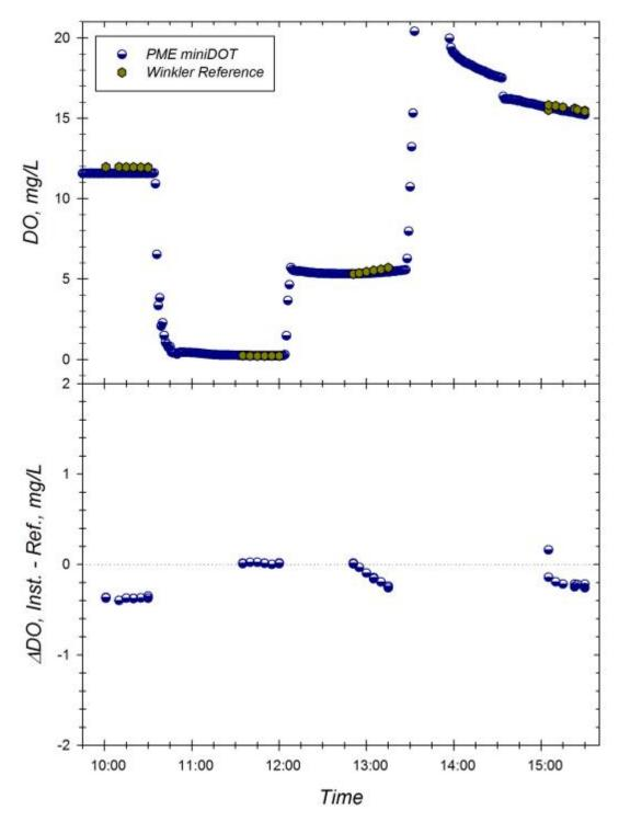
**Figure E.** Response of the PME miniDOT (sn 7392-340698) to changing dissolved oxygen concentrations at 5.3°C and S=8.98. *Top Panel*: Time series of instrument readings and Winkler reference samples drawn at level of sensor foil in well-mixed test tanks. *Bottom Panel*: Corresponding offset between instrument reading and Winkler DO reference sample during exposure trial. Dotted line represents zero offset from reference.
