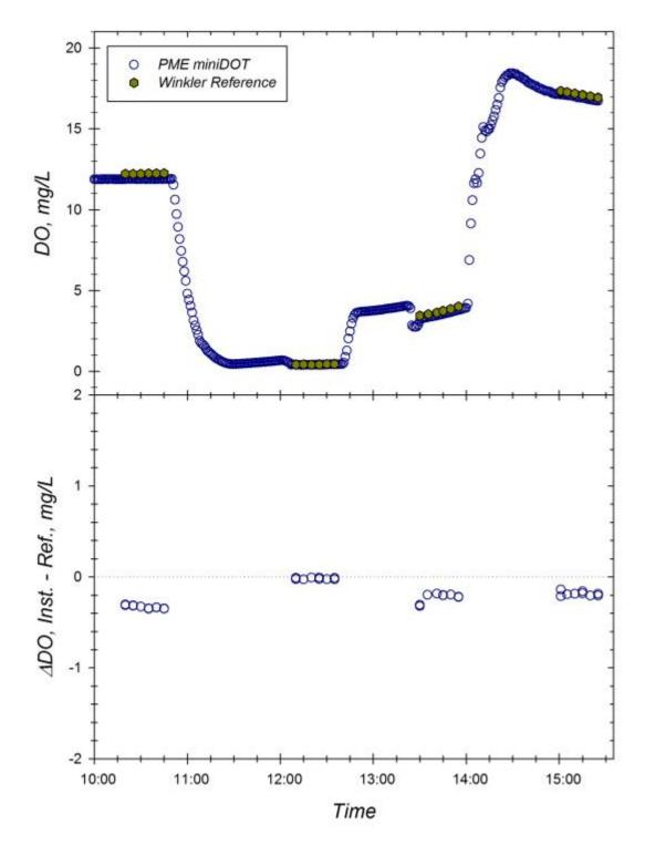
**Figure D.** Response of the PME miniDOT (sn 7392-340698) to changing dissolved oxygen concentrations at 5.4°C and S=0.00. *Top Panel*: Time series of instrument readings and Winkler reference samples drawn at level of sensor foil in well-mixed test tanks. *Bottom Panel*: Corresponding offset between instrument reading and Winkler DO reference sample during exposure trial. Dotted line represents zero offset from reference.
