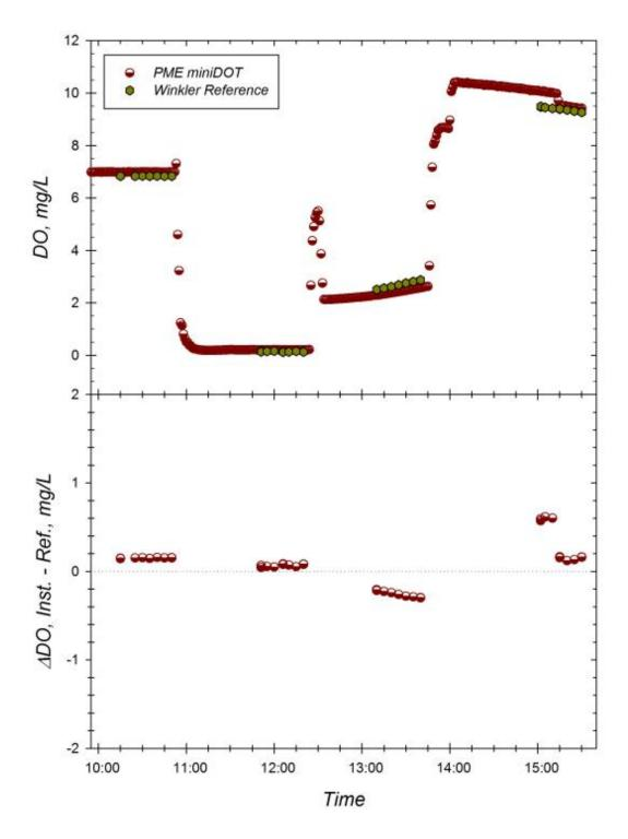
**Figure H.** Response of the PME miniDOT (sn 7392-340698) to changing dissolved oxygen concentrations at 30.5°C and S=9.28. *Top Panel*: Time series of instrument readings and Winkler reference samples drawn at level of sensor foil in well-mixed test tanks. *Bottom Panel*: Corresponding offset between instrument reading and Winkler DO reference sample during exposure trial. Dotted line represents zero offset from reference.
