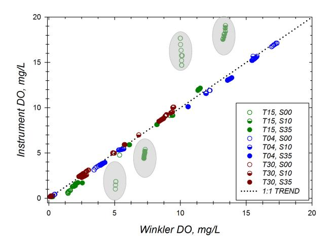
**Figure J.** Concordance of the PME miniDOT (sn 7392-340698) oxygen measures paired with discrete Winkler DO reference samples. In general readings are well correlated across a range of DO concentrations (hypoxic to supraoxic). Offsets in instrument readings increase at higher DO levels and with salinity. Dotted line represents perfect agreement between the two measures.
