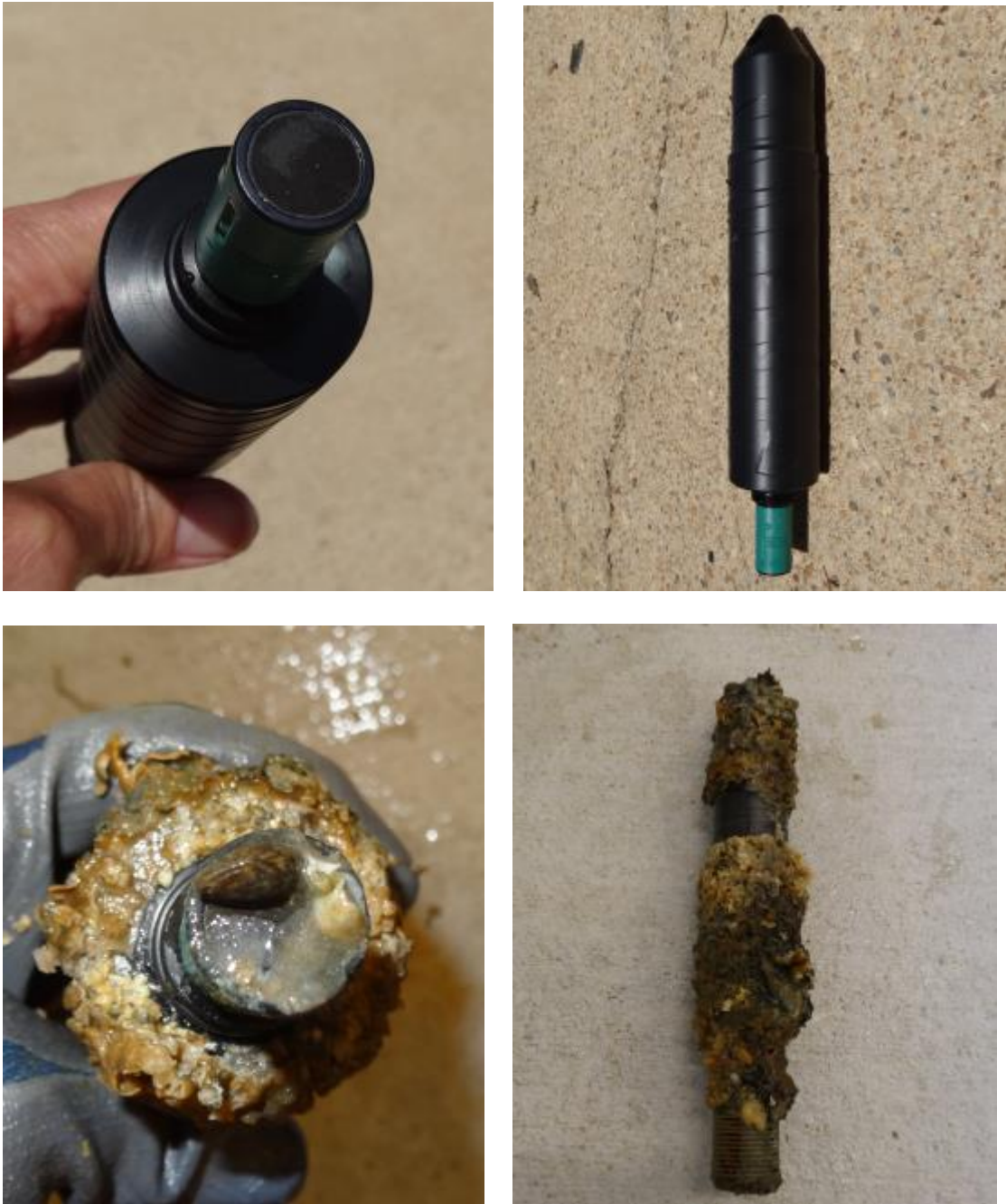
Photo 4. The HOBO instrument before and following the 12 week CBL field trial.
