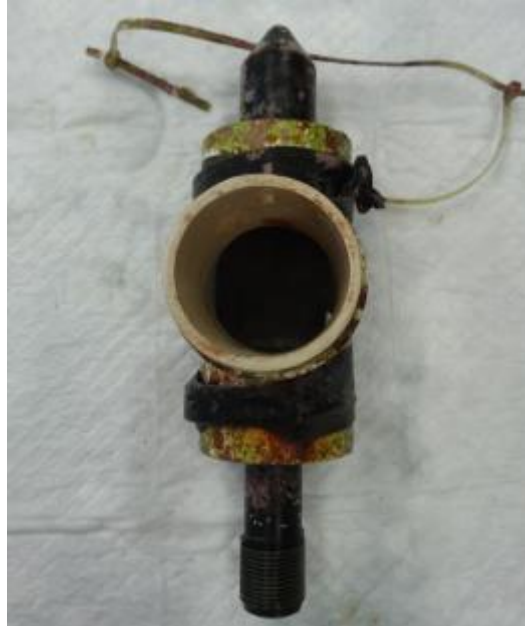
Photo 6. The HOBO U26 prior to and following the 18 week HIMB field trial.
