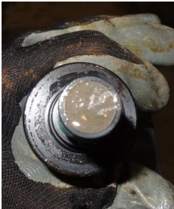
Photo 2. HOBO U26 prior to and following 15 week deployment under ice for the MTU field test.
