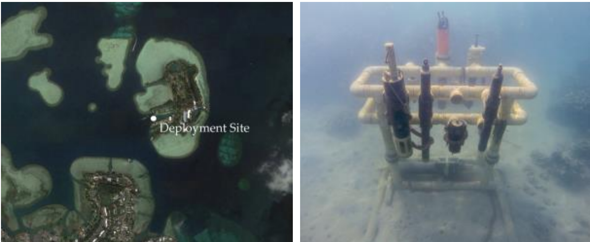
Photo 5. Aerial view of HIMB deployment site (left) and instrument rack in-situ (right).
