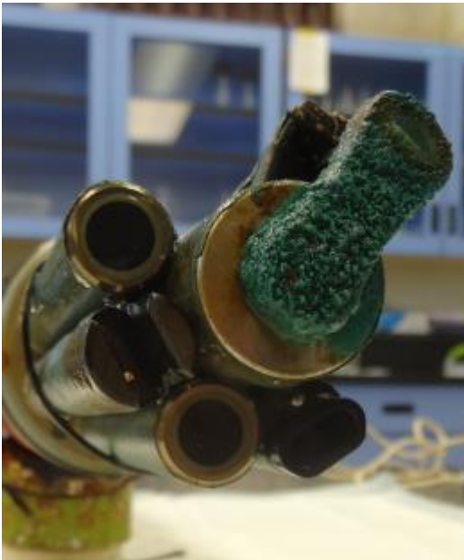
Photo 6. The EXO2 prior to and following the 18 week HIMB field trial.
